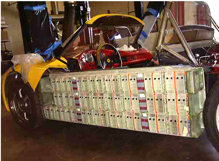
Lithium-ion battery modules were installed in the side panels of AC Propulsion's Tzero electric car. The vehicle used one hundred modules. Each contained sixty-eight finger-sized cells, for a total of sixty-eight hundred battery cells. (PHOTO COURTESY OF TOM GAGE.)
