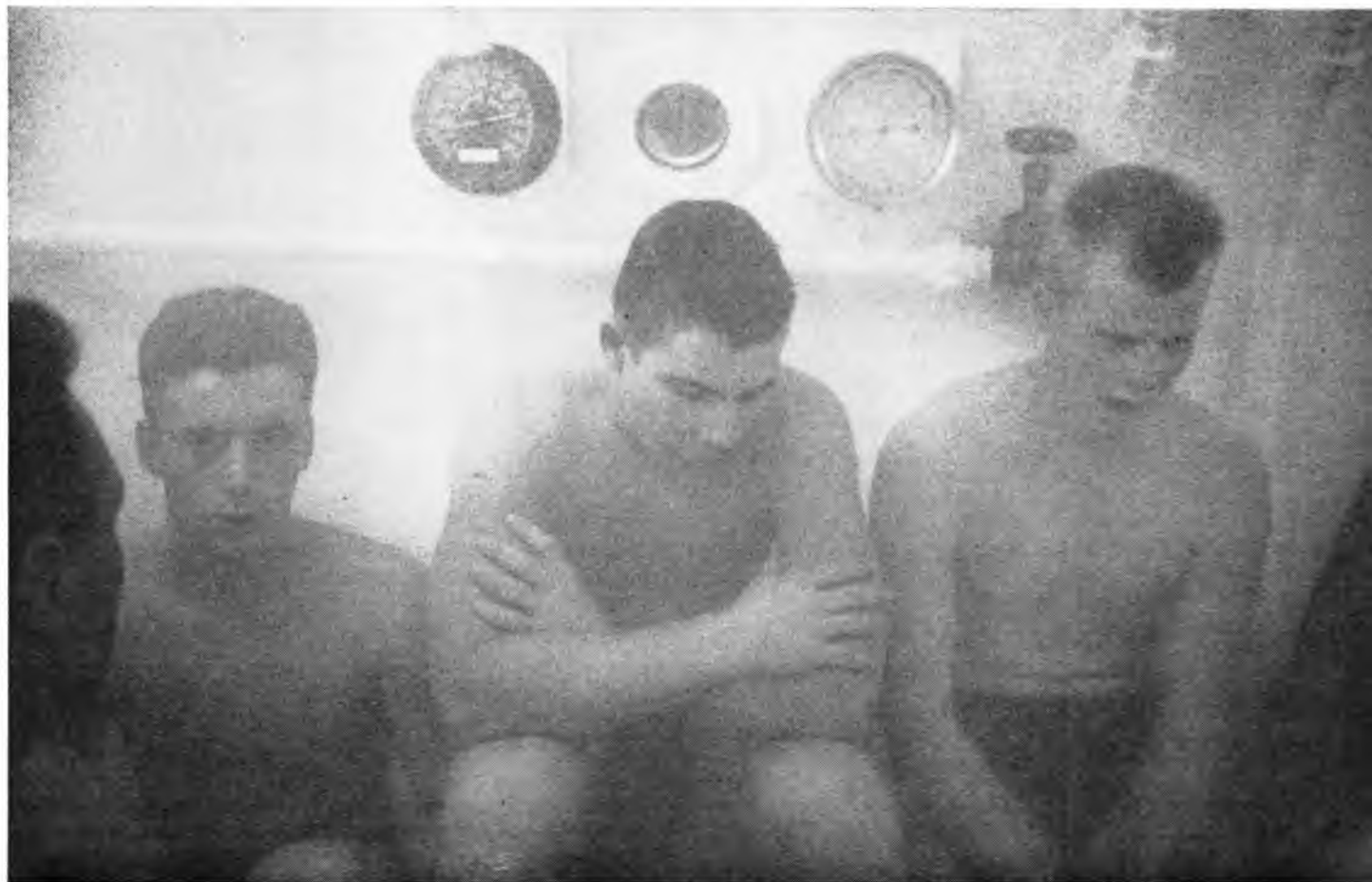
Fog rises in preliminary pressure chamber when Prahm's class is subjected to 44.4 pounds of pressure per square inch, equivalent to pressure in 100 feet of water. Chamber gets extremely warm and nitrogen in air makes men feel giddy.
