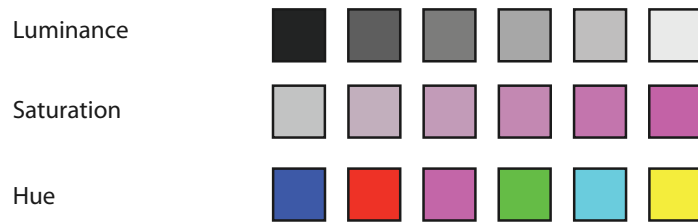
Figure 10.5. The luminance and saturation channels are automatically interpreted as ordered by our perceptual system, but the hue channel is not.
