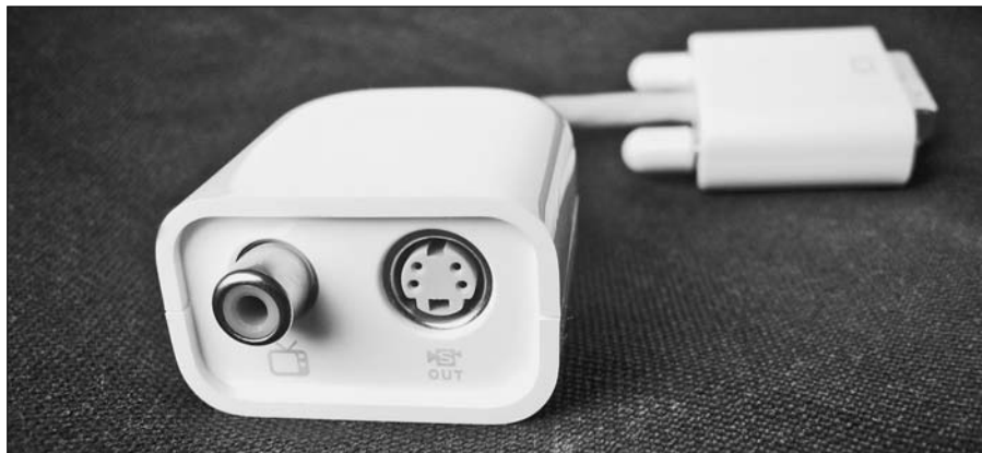
Figure 9-4: Apple's DVI to Video Adapter gives you composite video (left) and S-Video (right).
