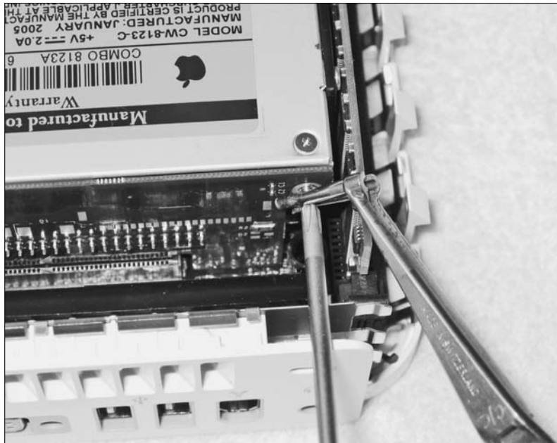
Figure 8-9: Hold the screw in place with tweezers while you screw it in.
