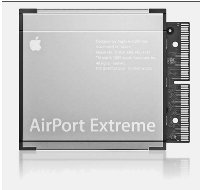
Figure 6-6: A standard AirPort Extreme card fits in the Mac mini.
