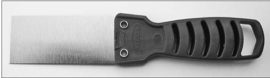
Figure 4-1: A 1½-inch putty knife is the best tool for opening the Mac mini.
