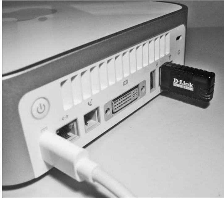
Figure 6-7: The tiny D-Link USB Bluetooth adapter is cheaper than internal Bluetooth.
