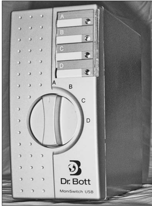
Figure 2-4: A KVM switch lets you share one keyboard and monitor between two Macs.
