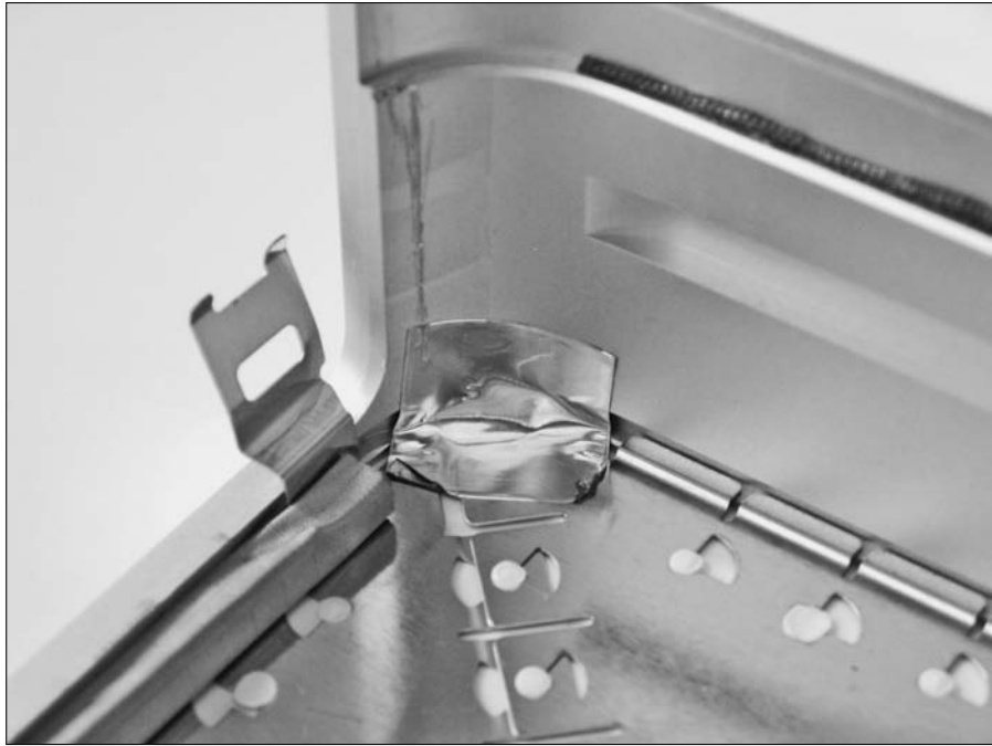
Figure 17-4: Pull up the metal tape in the corners of the casing.
