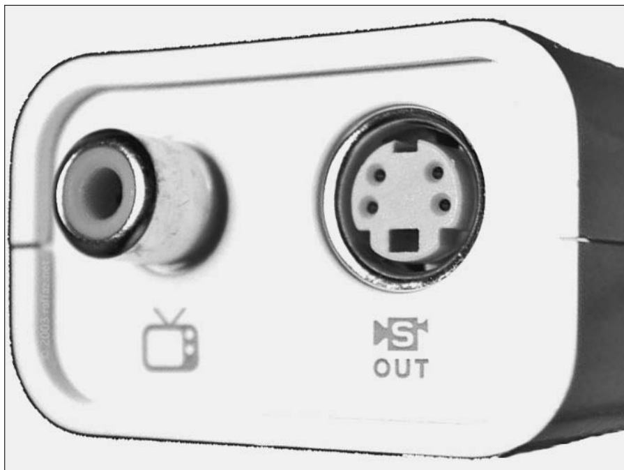
Figure 2-5: Connect to a TV via S-Video or composite video with the Apple DVI to Video Adapter.
