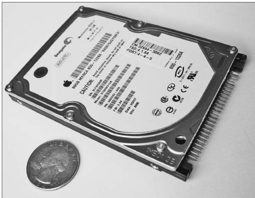
Figure 7-4: The Mac mini uses a 2.5-inch hard drive, shown here next to two bits.
