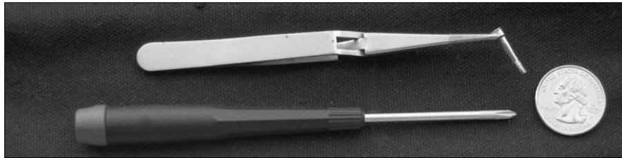
Figure 5-5: A jeweler's #0 Phillips and a pair of bent nose forceps.
