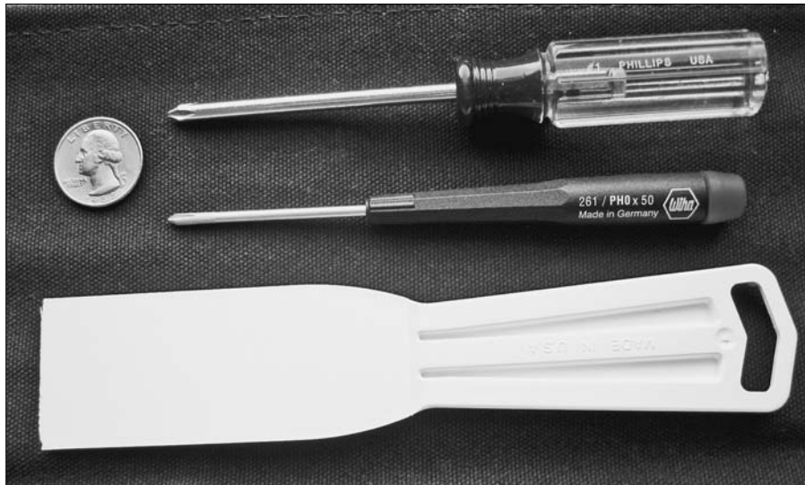
Figure 7-5: Use these tools to replace the mini's hard drive.
