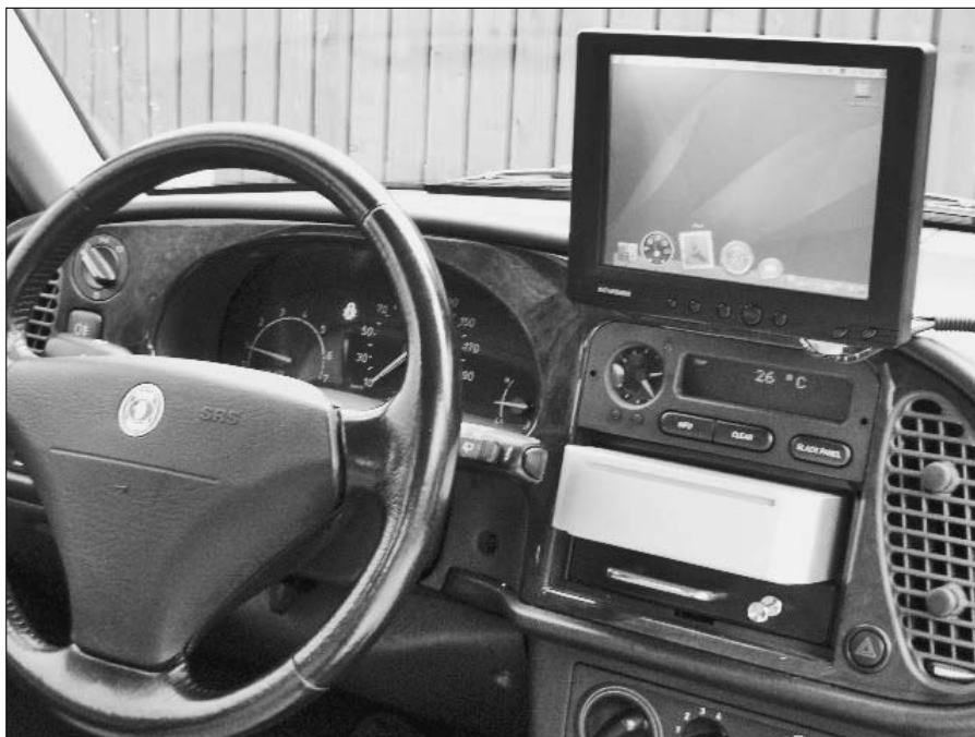
Figure 14-4: A Mini Dock installation.
