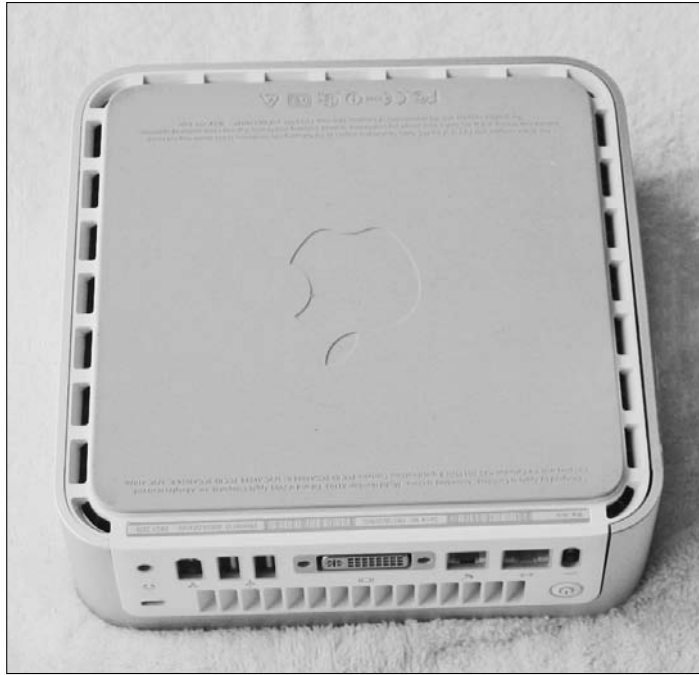
Figure 17-1: Don't block the air vents that ring the bottom of the mini.
