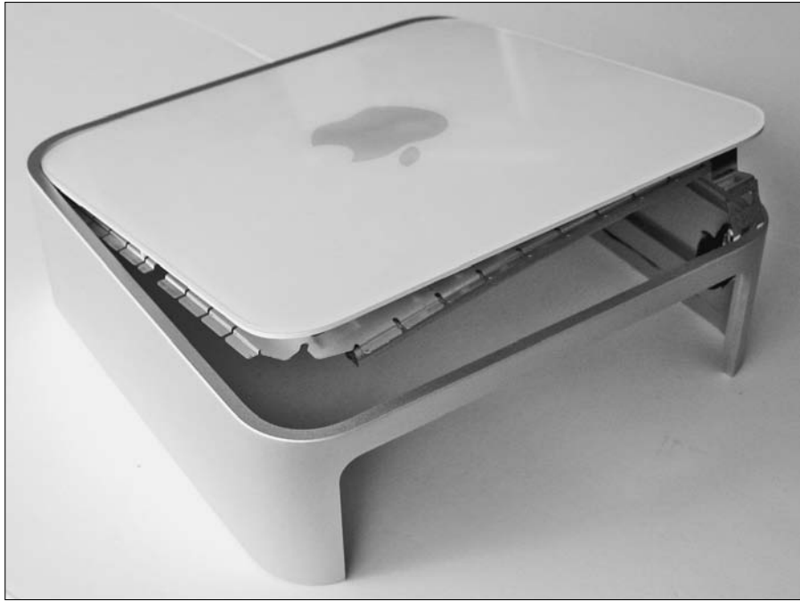
Figure 17-5: When you push with your thumbs, the top pops out.
