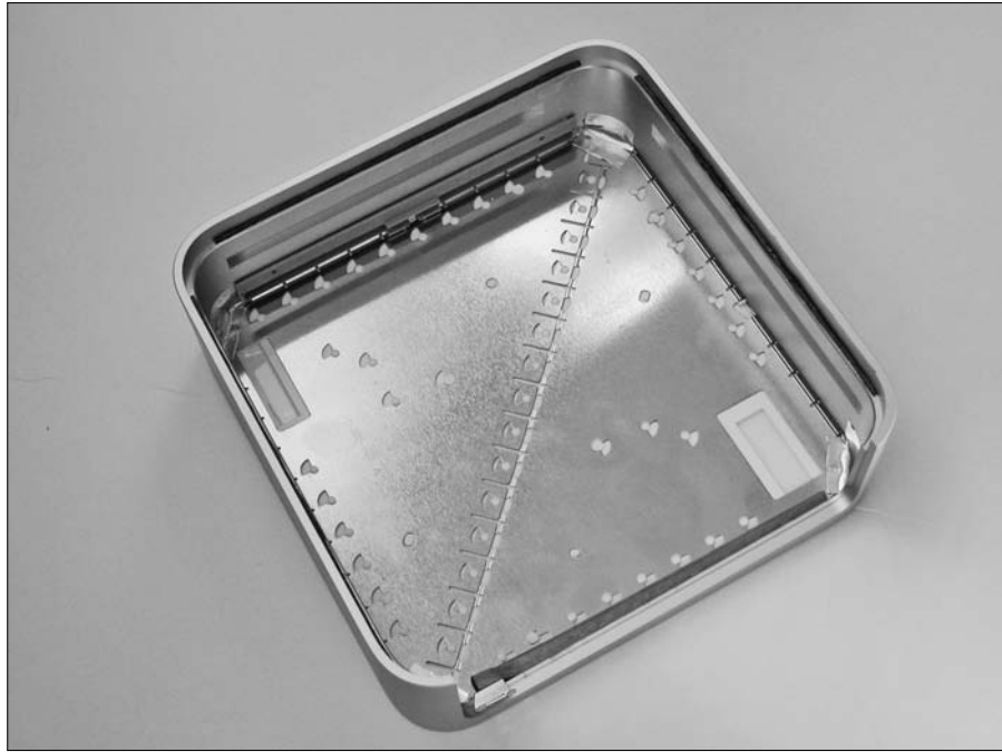
Figure 17-3: The white plastic top is attached to the EMI shield with small plastic rivets.
