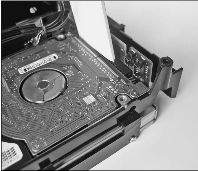
Figure 7-9: Unplug the hard drive from the intercon- nect board with a plastic tool.
