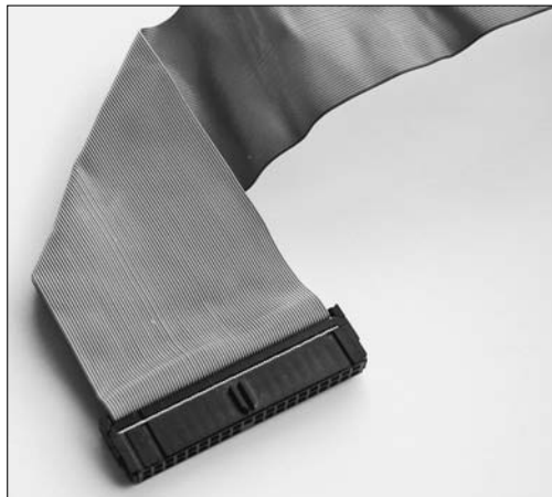
Figure 19-7: Fold and bend the ribbon cable to create 90-degree turns.
