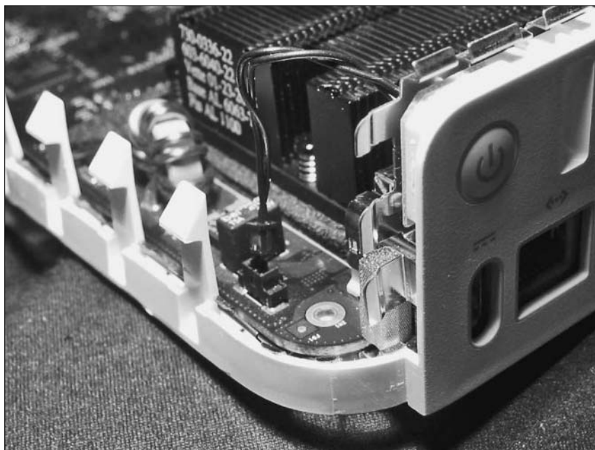
Figure 20-9: The power-on cable is located in the corner near the power switch.
