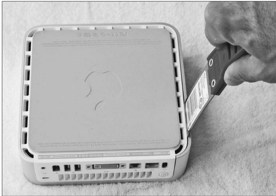
Figure 4-4: Insert the putty knife and push outward and down to release the tabs.
