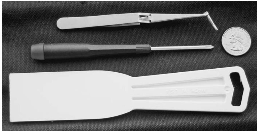
Figure 8-3: Use these tools to replace the mini's optical drive.
