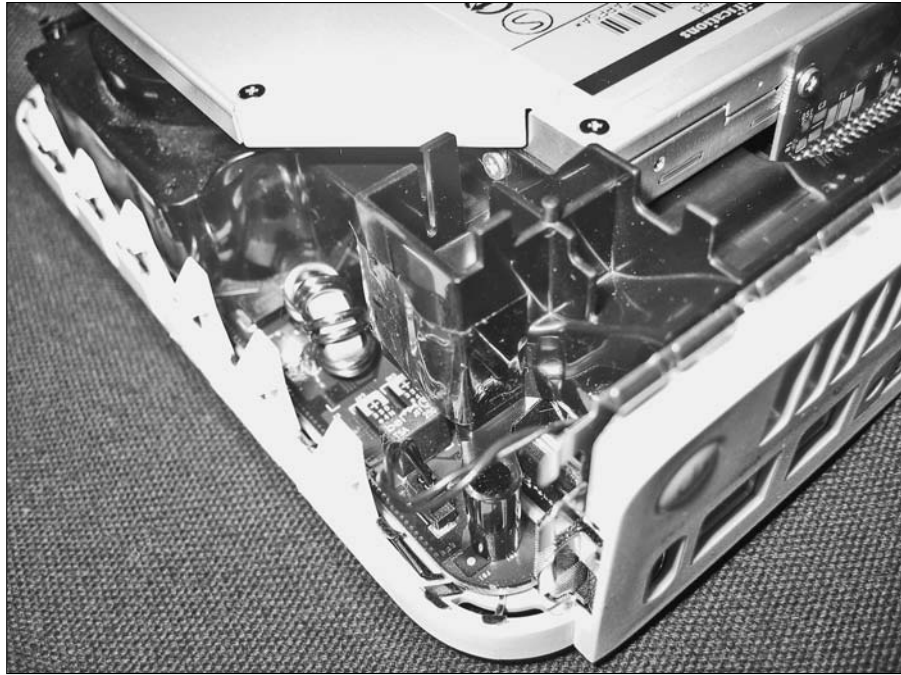
Figure 6-4: Snap the AirPort antenna onto this black column.
