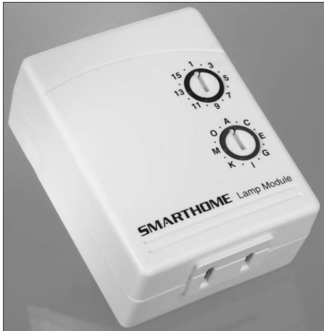
Figure 10-5: Set an X10 address on many modules by turning two dials.
