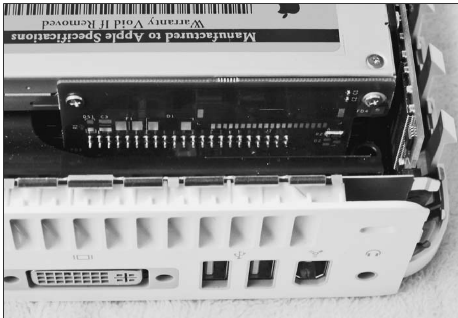
Figure 8-7: Remove these two screws in the interconnect board.
