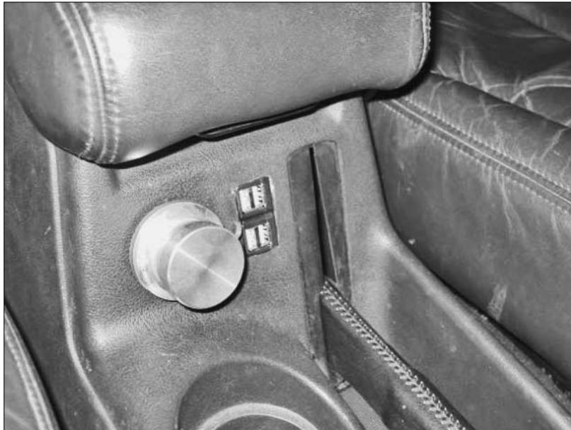
Figure 15-2: A USB hub custom- fitted into a car console.
