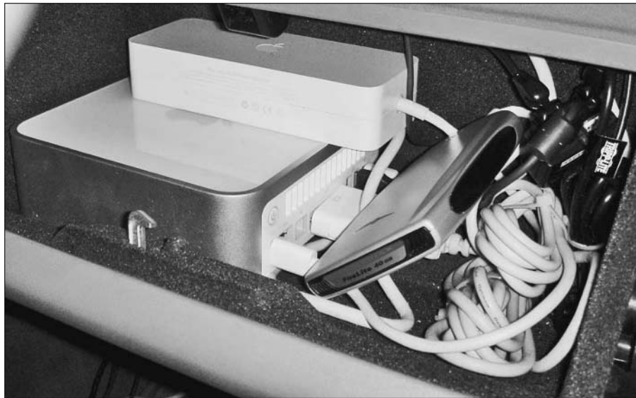
Figure 14-5: A Mac mini installed in the glove box of a Land Rover Discovery II.
