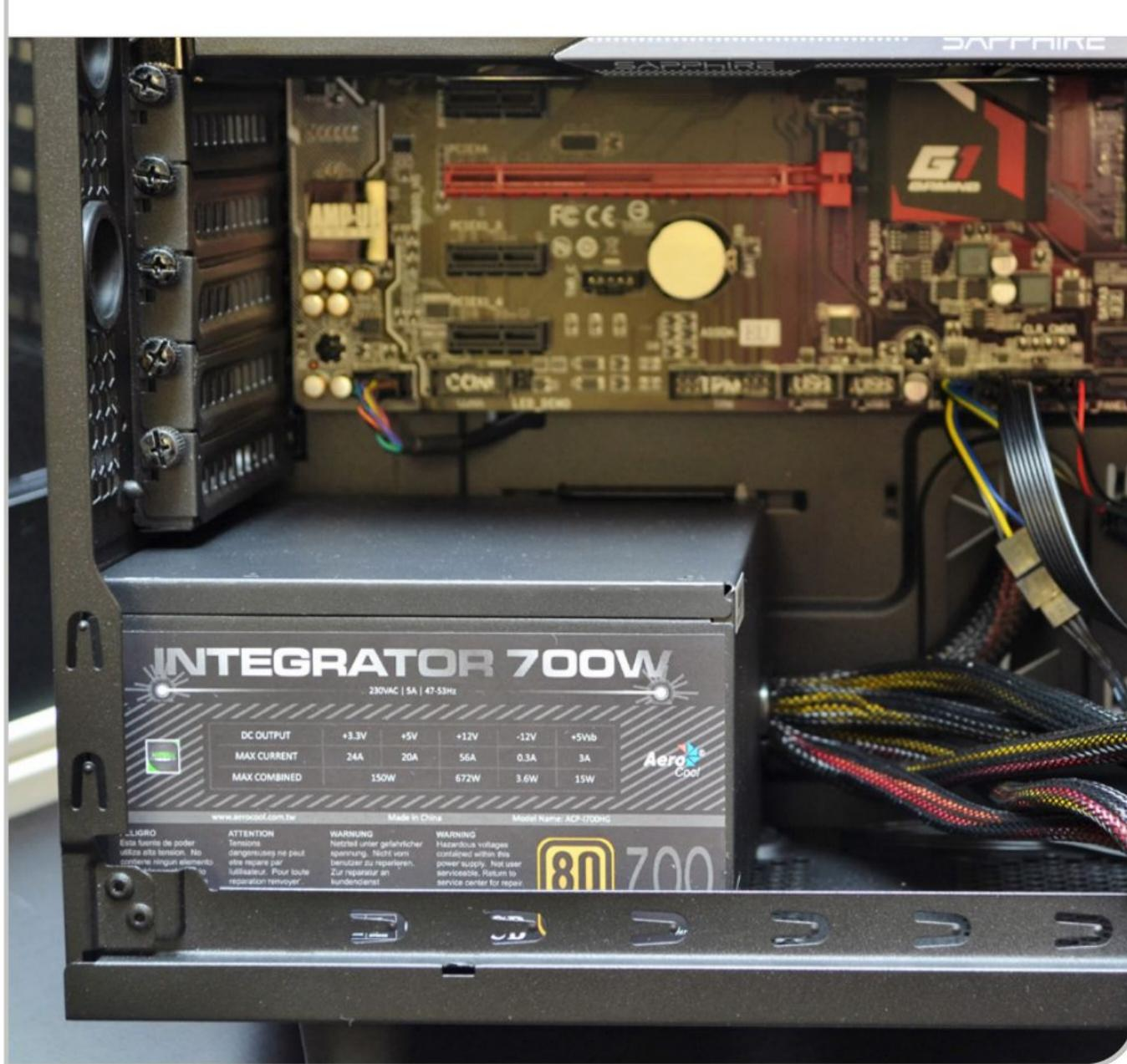
Power related problems are often the cause of a system not booting (when we get to that point). Make sure everything is properly connected and that you haven't missed a power cable before checking for less obvious problems. Some power supply's let you switch the input voltage between 110V (US) and 230V (UK). Make sure yours is set correctly for your location.
