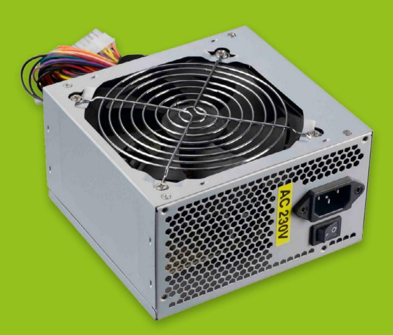
This can sometimes be a problem when using an older PSU in a new build. Newer motherboards with current generation graphics cards may require higher startup current than some of the older power supplies can deliver. This results in the system trying to start but struggling without enough power to run everything it needs to.
