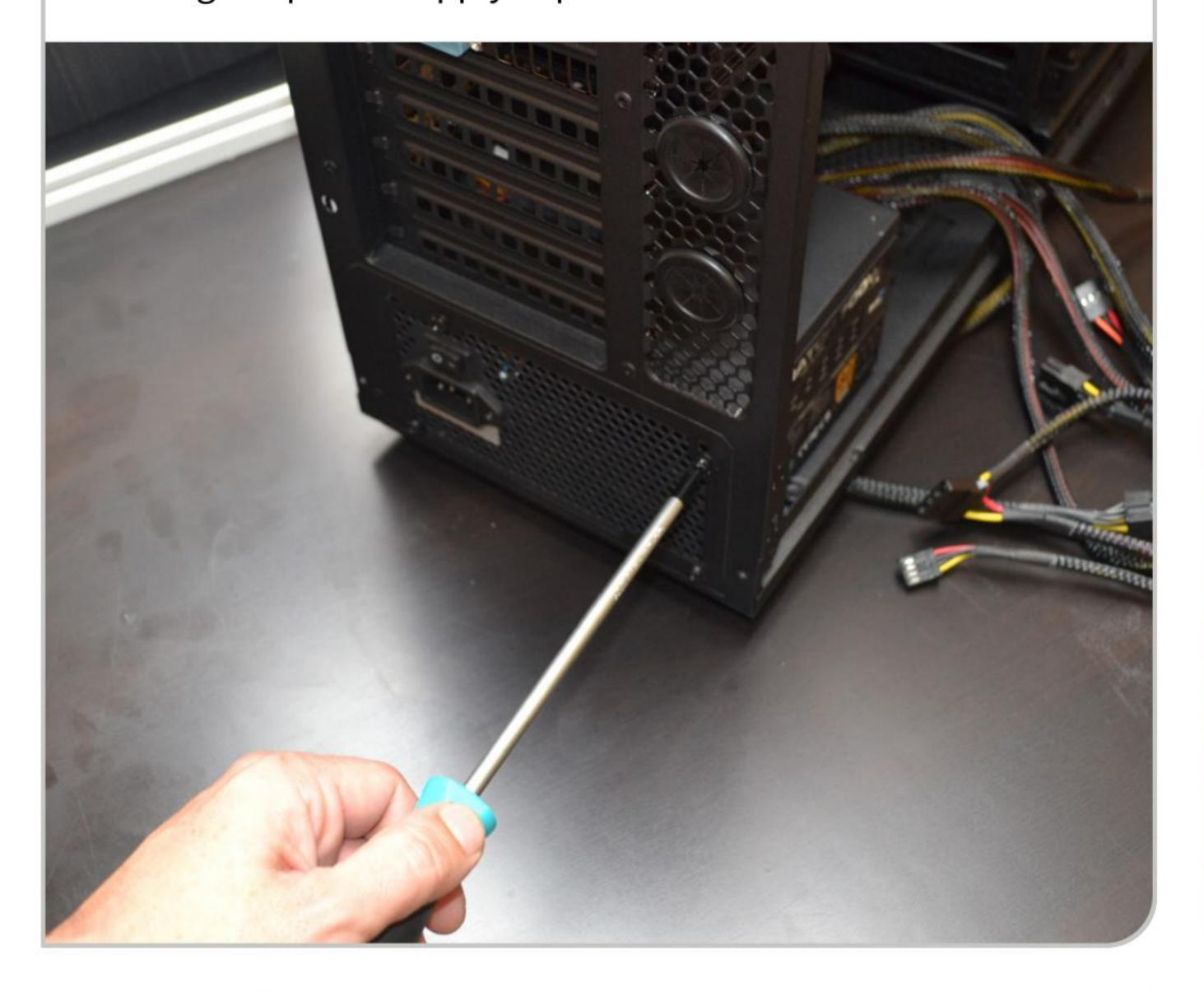
If your case has cable management holes in the back of the chassis, you can start feeding cables through at the bottom of the case. Work out how many of the different PSU cables you need: probably a 4+4-pin, the main 20+4-pin, the PCIe 6-pin and a couple of SATA connections and tidy up the rest. If you are using a modular PSU, store the excess cables safely in the box.
