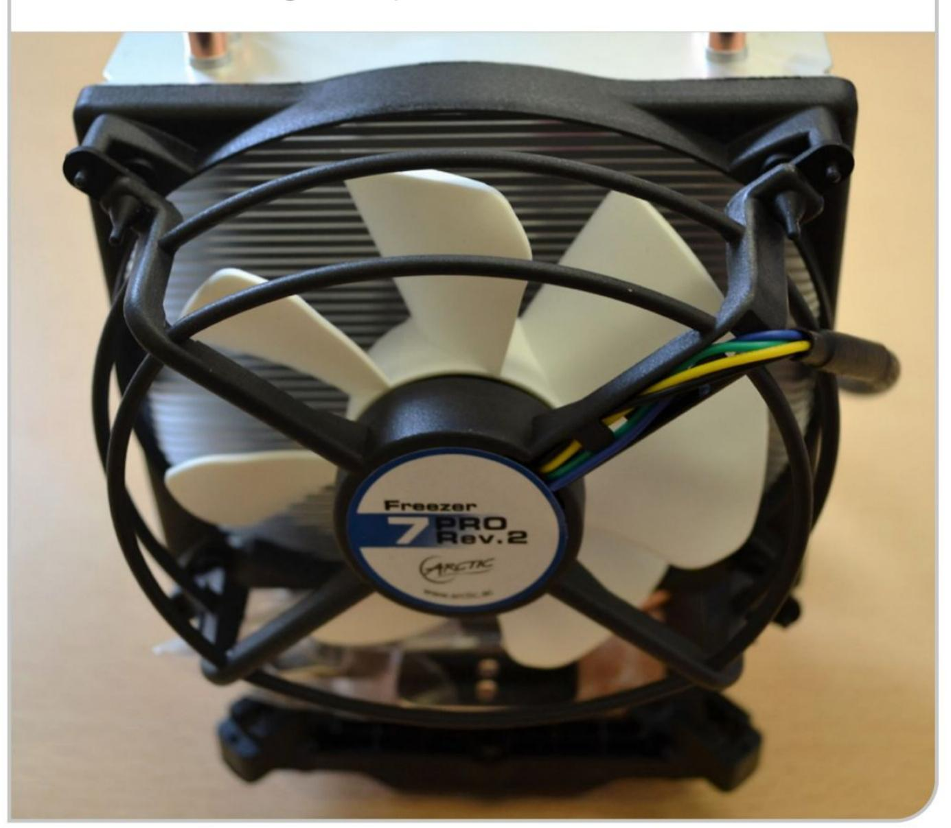
You can now carefully sit the CPU cooler on top of the CPU, ensuring that it is sitting level and use the supplied screws or other fixings to secure it in place. This step is quite an important one to get right first time, as trying to remove it and then clean up thermal paste is a chore. As you apply slight, even pressure, the thermal paste will spread to fill the gap.
