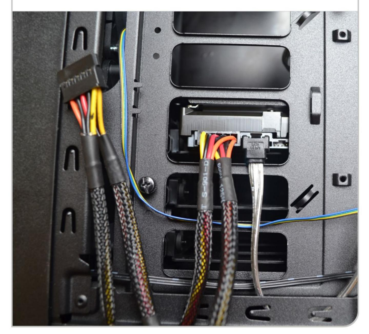
STEP 5 Keep airflow in mind and don't cover any case fans or coolers with a cable if at all possible. The Component placement within a system is also important. Drives, graphics cards and other expansion cards should be positioned in such a way that their cables, or the components themselves, don't interfere with one another. Don't be afraid to move a component if needed.
