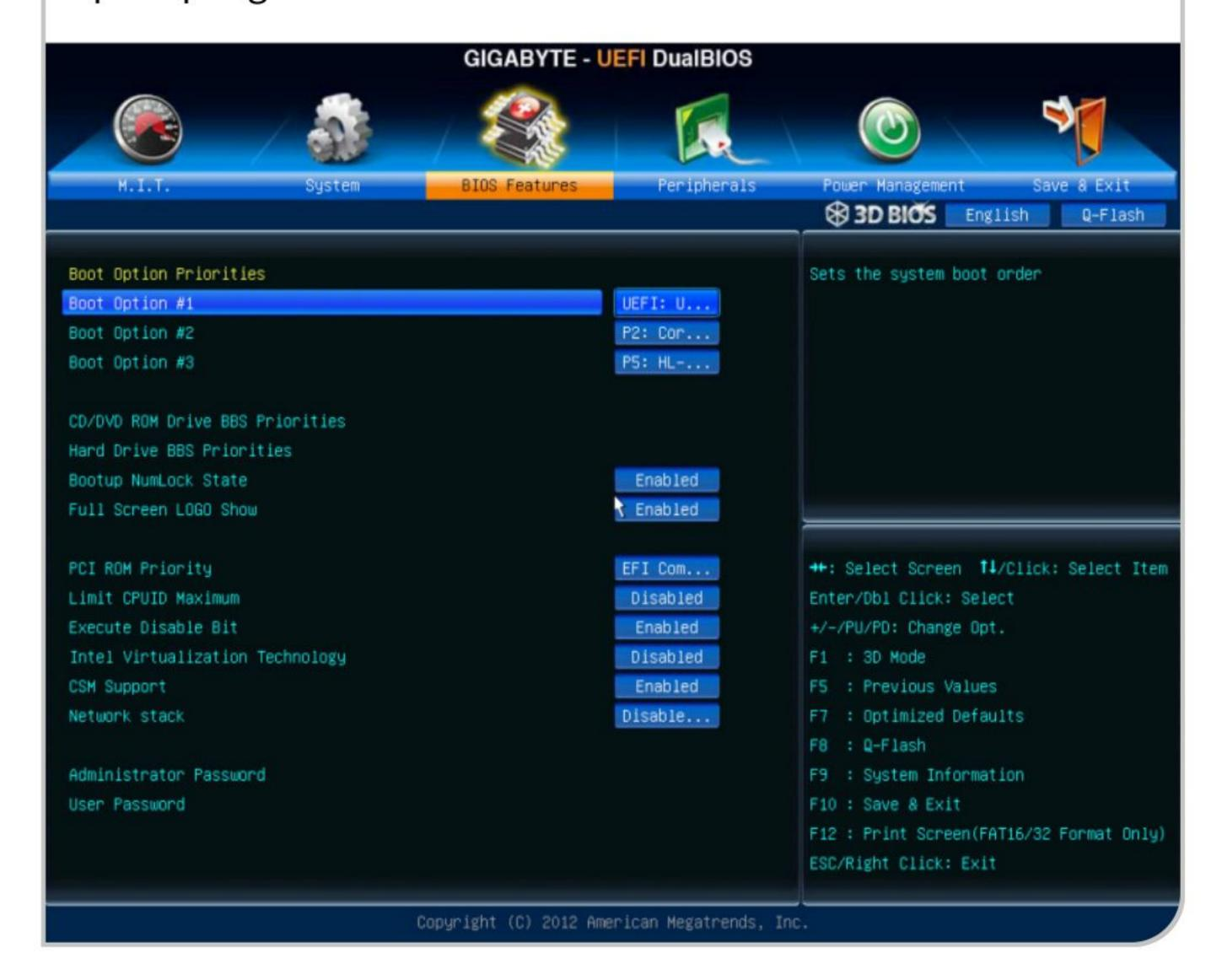
Use the arrow keys to select the BOOT tab. System devices appear in order of priority. BIOS settings allow you to run a boot sequence from a floppy drive, a hard drive, a CD-ROM drive or an external device. You may configure the order that your computer searches these physical devices for the boot sequence. The first device in the order list has the first boot priority.
