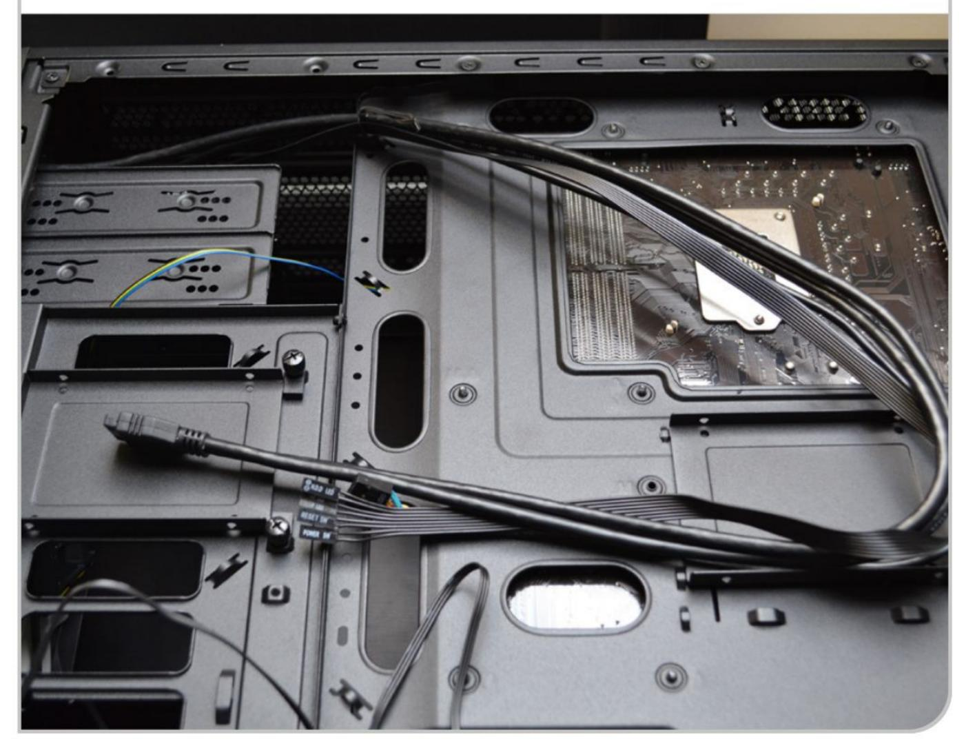
Apart from possibly the case fan connection, connections for front USB, audio in and out sockets and the power and reset switches are normally positioned along the bottom edge of the motherboard. Each connection socket will be labelled on the motherboard but this is sometimes hard to see. Check the motherboard manual if unsure.
