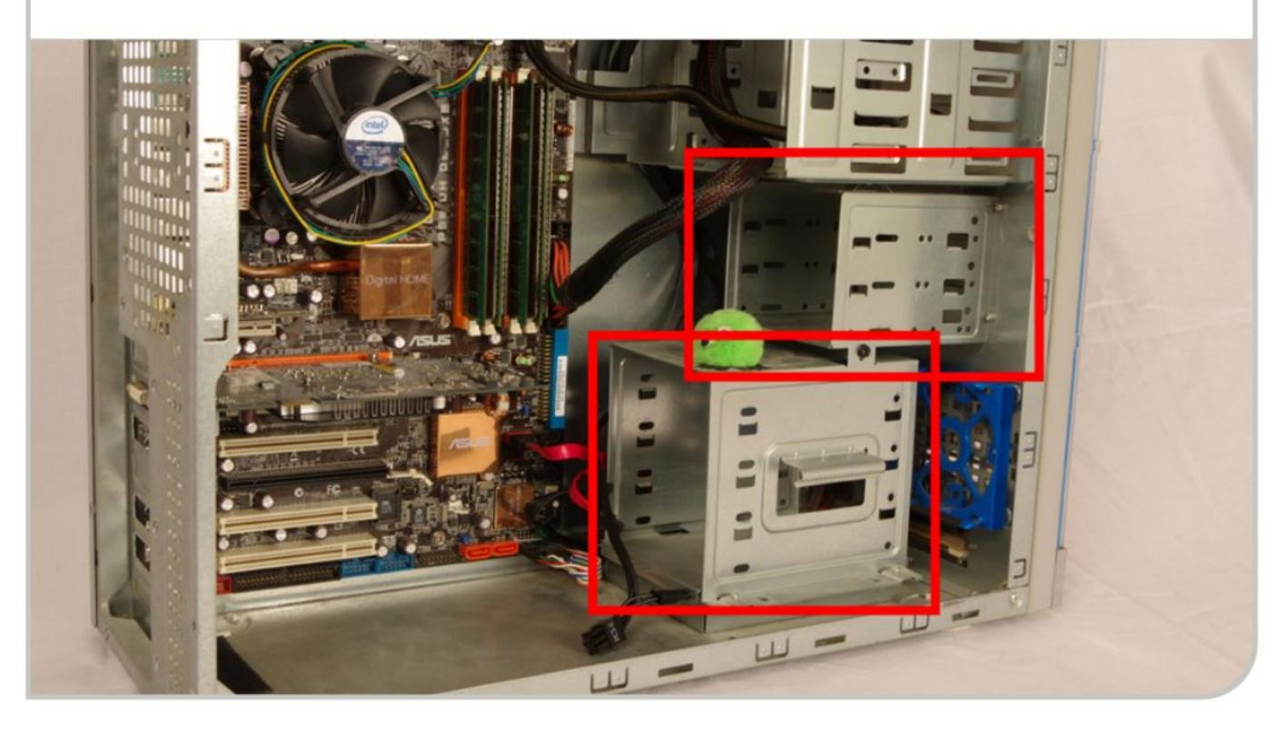
Once you've decided on a good position for the SSD within the drive bay, carefully slot the drive on its mounting plate into the drive bay. Position it so that the screw holes on the PC chassis line up with the holes on the mounting plate.
