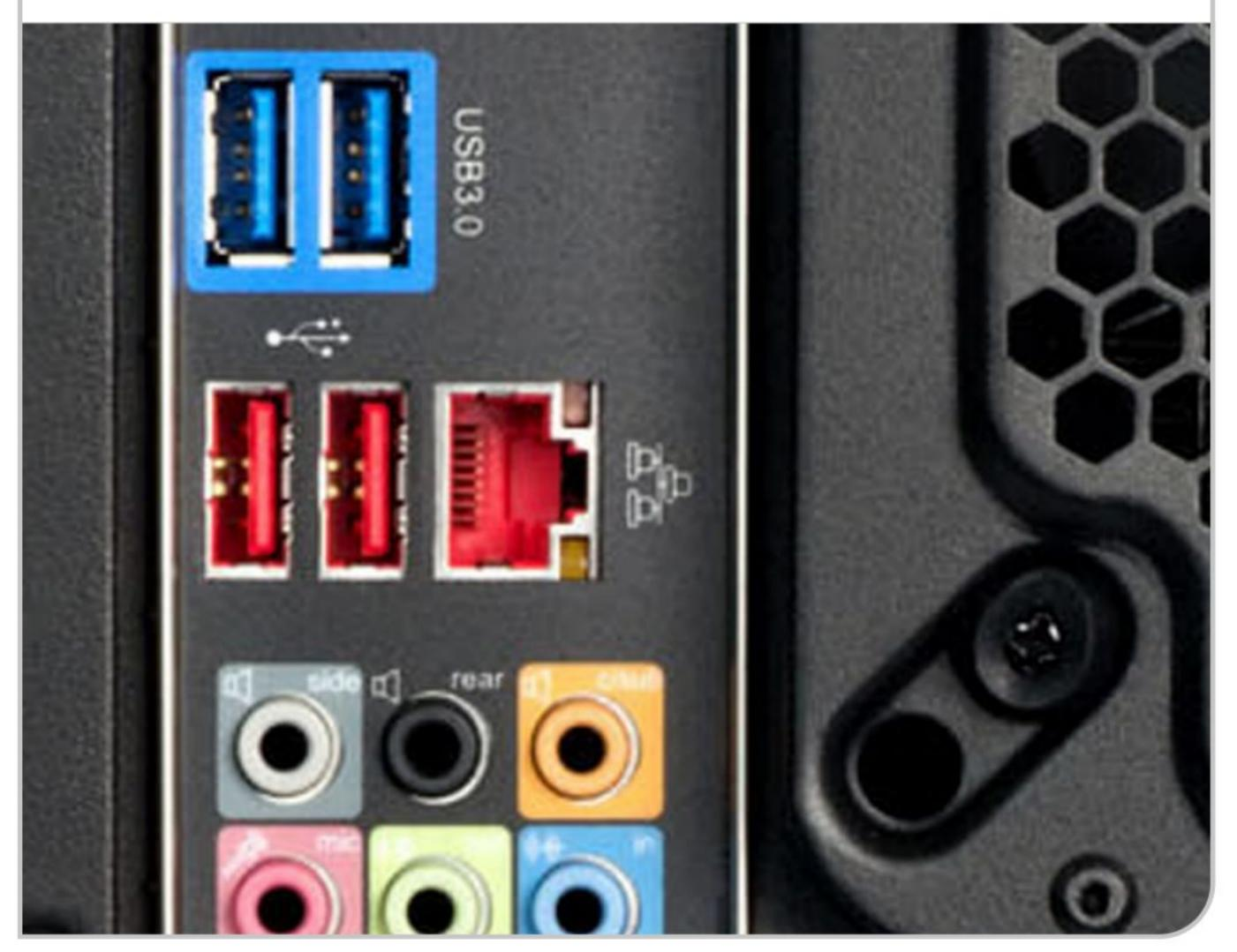
STEP 2 If you have a set of speakers that you'd like to use, connect them now. If you're simply connecting a pair of stereo speakers, connect the 3.5mm audio cable from the speakers into the green audio jack on the back of the PC or into your dedicated sound card. Surround sound speakers require more connections. Simply match the colour-coded cables with the matching coloured ports.
