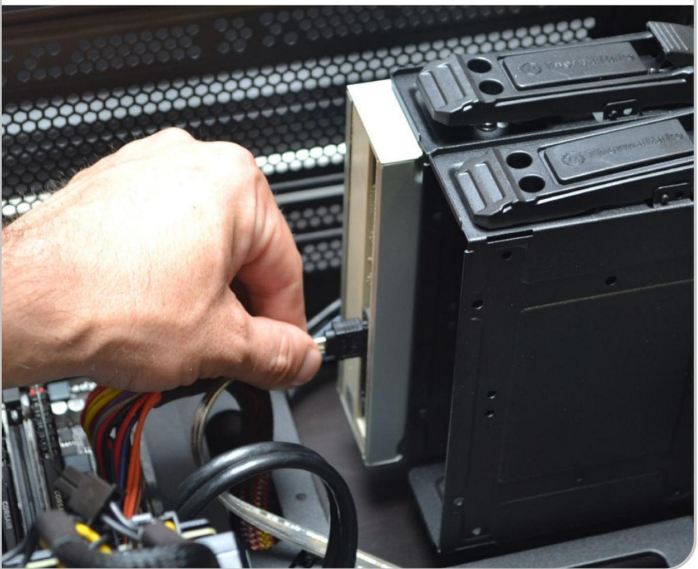
You can now replace the front panel of the case and adjust the position of the optical drive, if needs be, by loosening the fixing screws slightly and using the slots to slide it back or forward. If you have a second optical drive to fit and if your case features a second bay, repeat steps 1-4. There are several other components that can be fitted into a 5 ¼ in drive bay, such as fan controllers.
