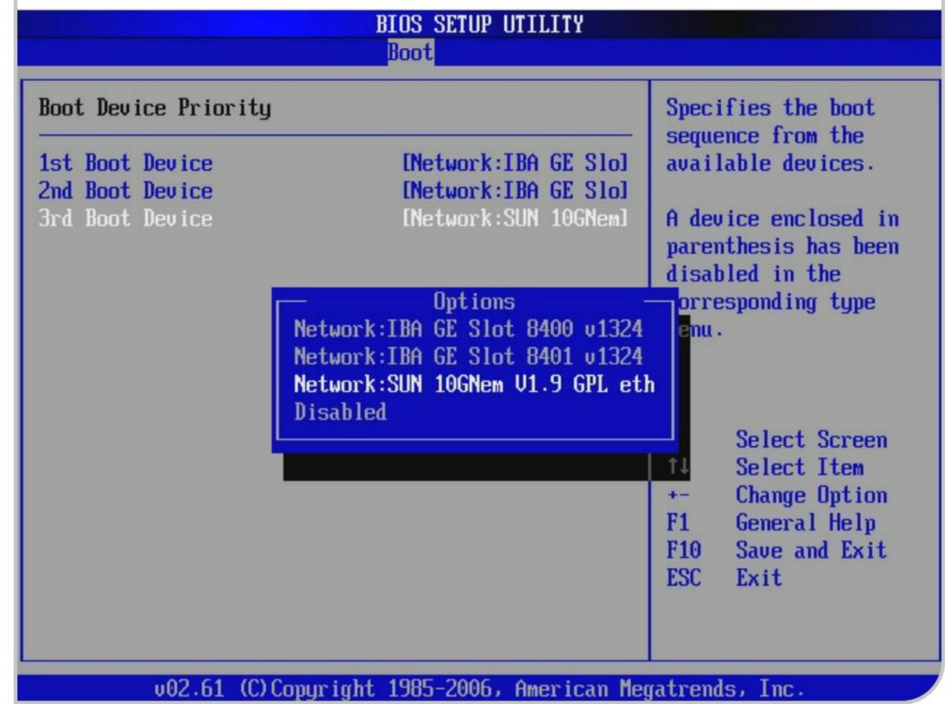
BIOS (Basic Input Output Subsystem) is a programmable chip that controls how information is passed to various devices in the computer system. A typical method to access the BIOS settings screen is to press ESC, F1, F2, F8 or F10 during the boot sequence. Power your PC up, insert your bootable disc or USB, restart and press the relevant keyboard key until the BIOS menu opens.
