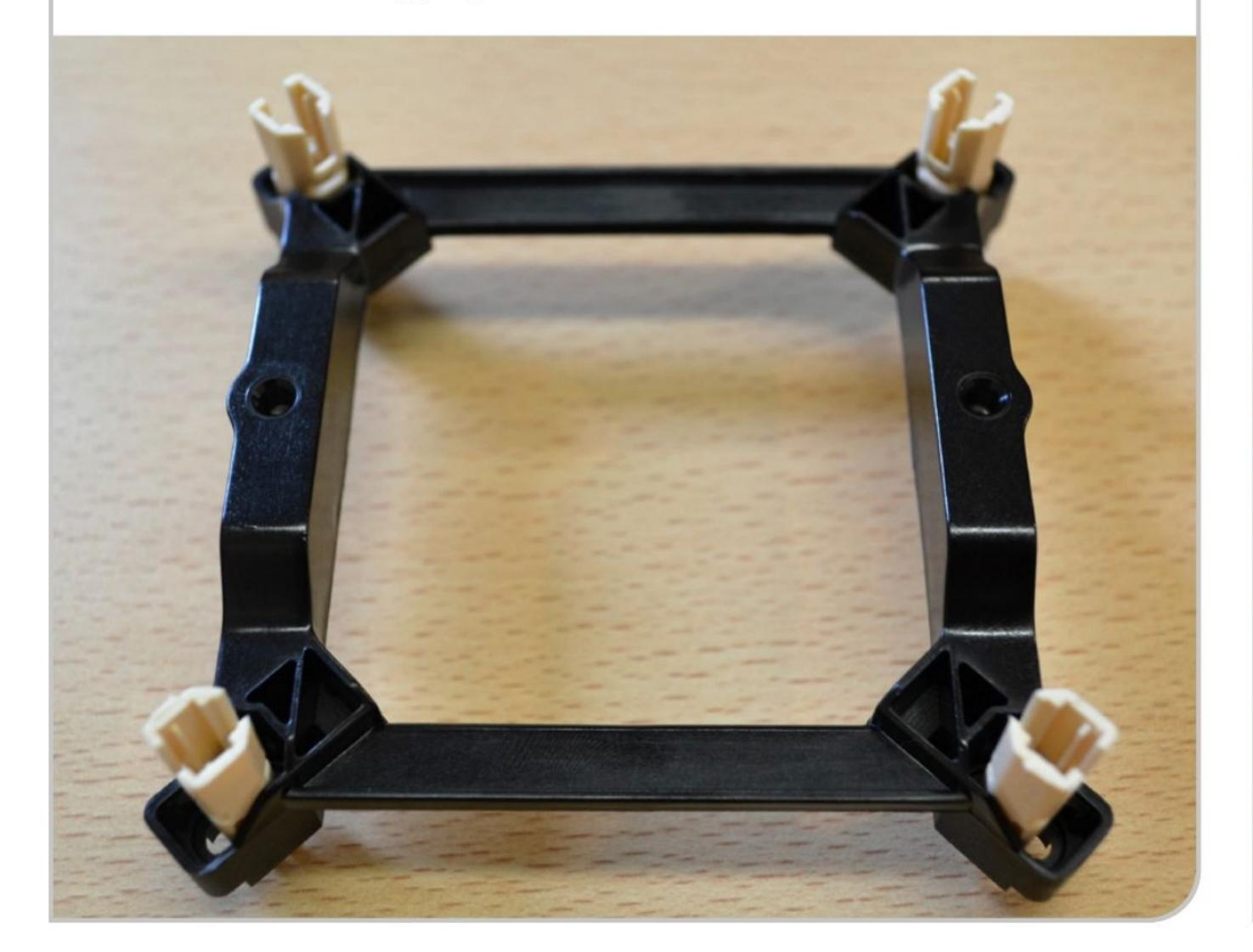
Carefully position the mounting plate on to the motherboard, lining up the pegs with the holes on the board, before pressing them through. This will see the mounting plate held loosely in position. You now need to push a pin into the mounting peg in each of the corners, pressing firmly down until you feel a slight click. The mounting peg is now held firmly in place.
