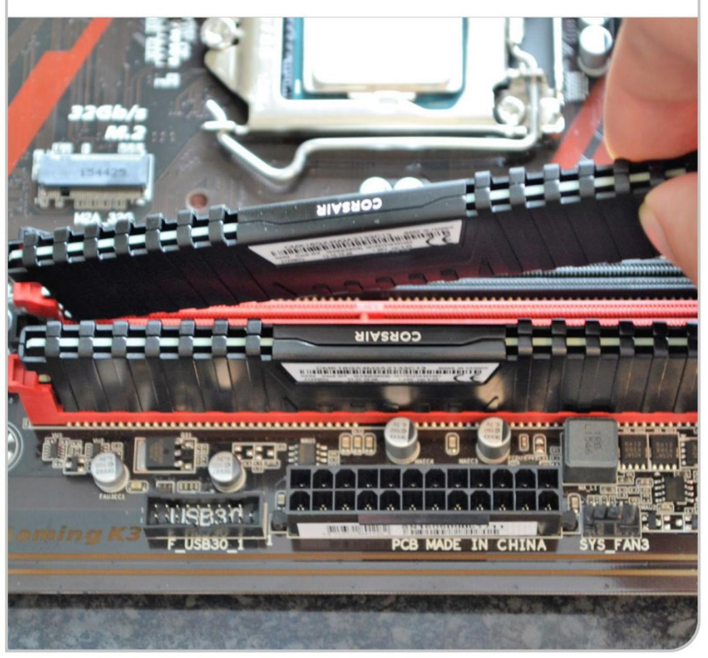
Memory modules have an offset notch in the row of connectors on the bottom. This will correspond with a divider in the motherboard memory socket, ensuring that you can't insert the DIMM the wrong way around. The memory socket will also usually have a hinged clip at each end that needs to be pressed down and away from the socket.
