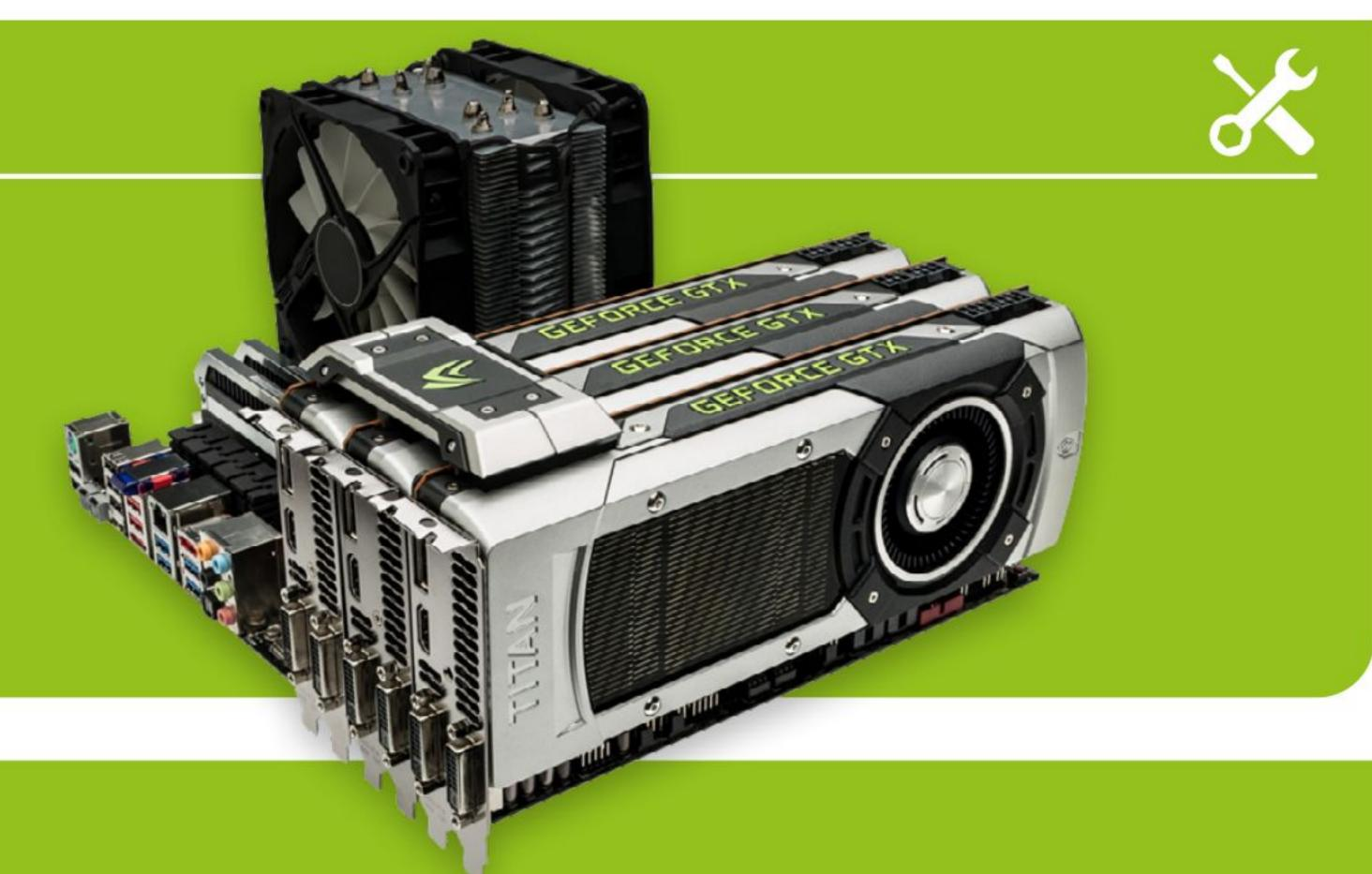
Make sure there is no cover on the card connector and then carefully lower it into the PCIe socket. These sockets always have a catch on them, which will help hold the card securely in place. You may need to slide or tilt this catch back to get the connector into the socket. The connector on the card will have a slot in it that will help you line it up with the socket correctly.
