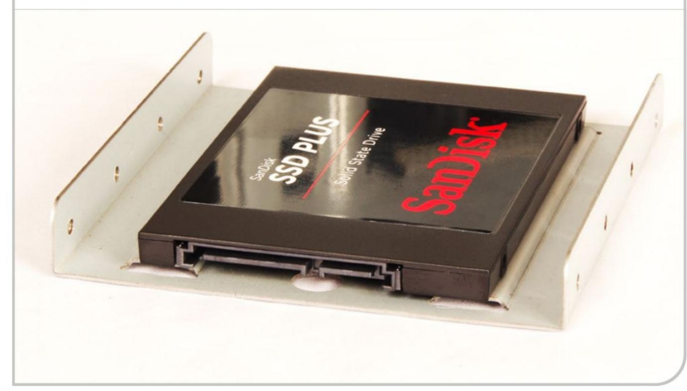
AN SSD can fit into either a 3.5-inch (floppy disk drive) bay or a 5.25-inch (HDD/optical drive) bay. Since many recent PC cases no longer have 3.5-inch bays we'll show how to fit your SSD into the larger one.
