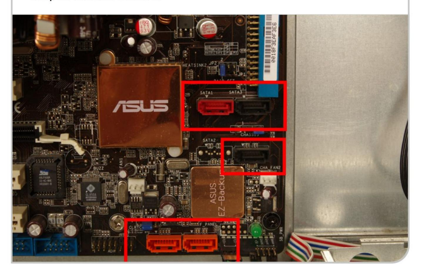
Plug one end of your SATA data cable into the socket on the motherboard. It should click into place. It can only go in one way and the two ends are identical, so you can't connect it the wrong way round.
