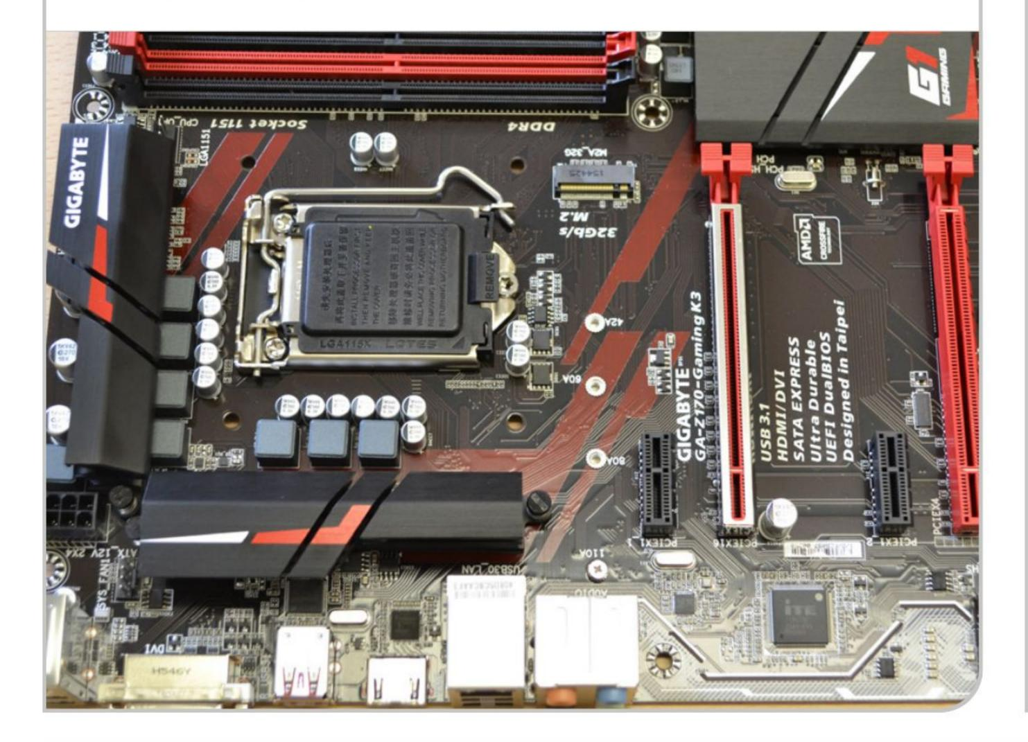
STEP 2 The process for fitting an AMD or Intel CPU is similar, but there are some physical differences between the two processor types, not least the arrangement of the contact pins. We are using an Intel Core i5 6600k CPU for our build and we will concentrate on that process. See further down the guide to see specific AMD CPU installation advice and precautions.
