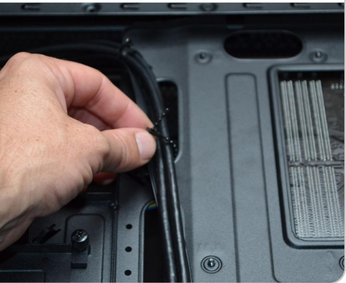
STEP 4 Some cables, such as the front panel audio, branch into two connections when you only need to use one. This usually means that a second connection branches off just before the main cable terminates. Fold the excess cable back on itself and tie it down to the main cable so it's out of the way. Do this for any other cables around the case, such as the PSU's SATA power cables.
