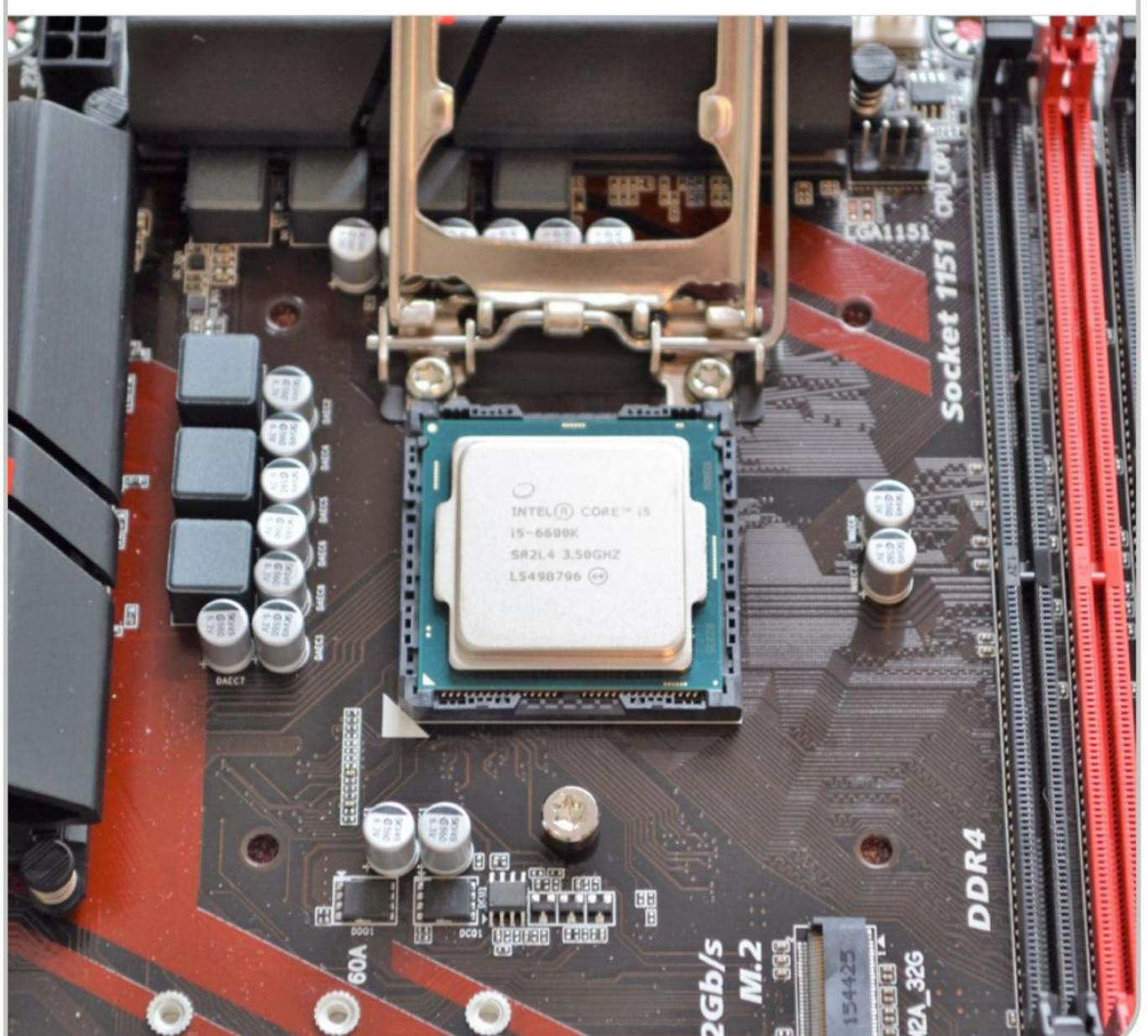
Carefully release the locking bar on the socket and lift it up. This will slide the processor lock back and hinge it up out of the way. Leave the plastic socket cover on for the moment. Take a close look at the now visible CPU socket and you will see a small arrow in the bottom left corner. If you look on the CPU itself, you will see that it also has a small arrow in one corner.
