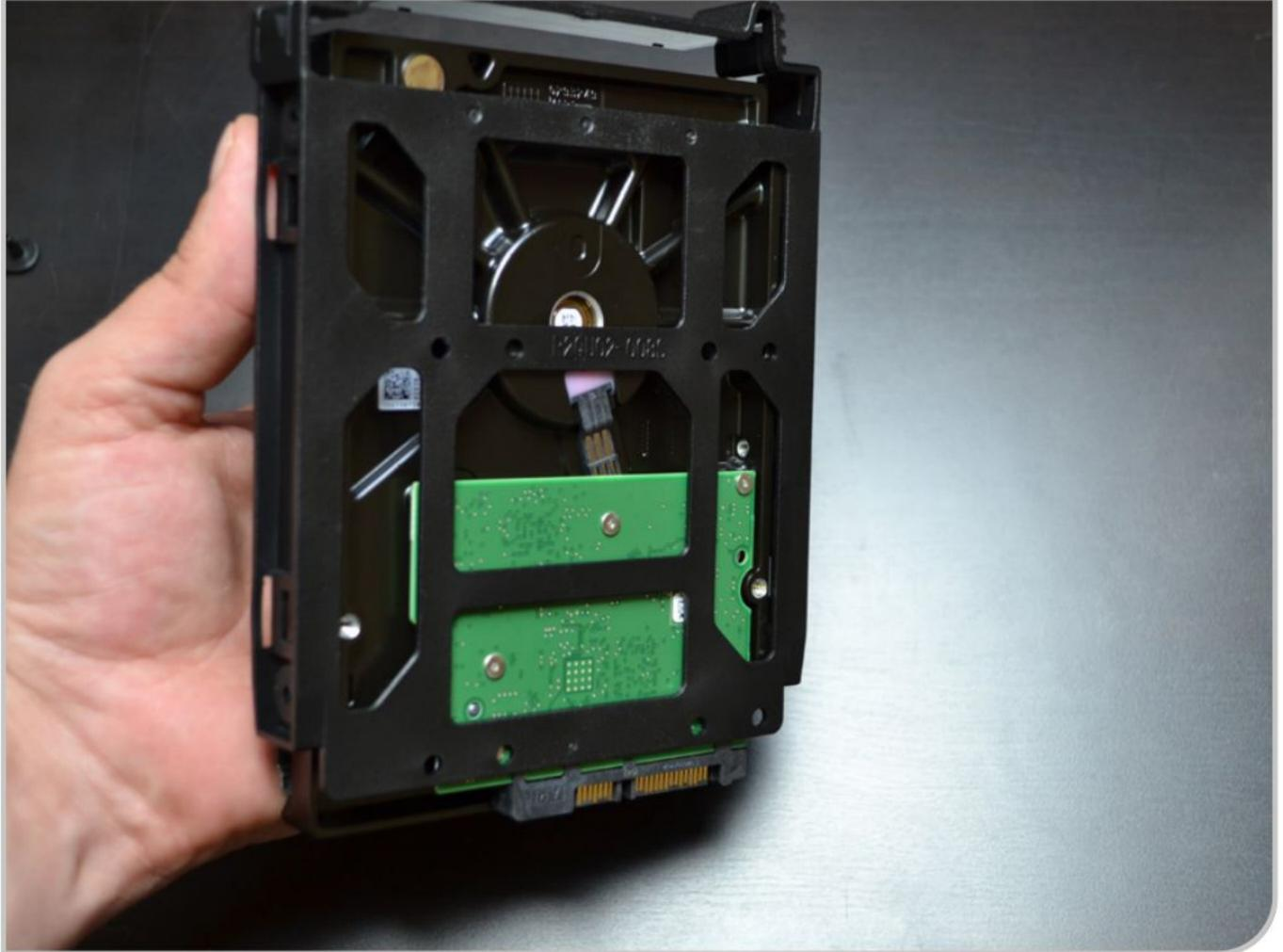
Pull a tray out of the cradle. Hard drive cradles are usually toolless but some may be screwed in. The method of fixing the hard drive into the tray varies between cases. Some will need to be screwed in and some will have screw-less fixings, such as the one shown here. Remove the screws or fixing and place your hard drive into the tray.
