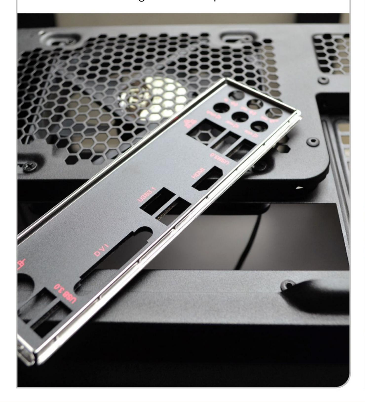
You obviously have to ensure that the plate is inserted the right way up, usually with the mouse and keyboard connections nearest the top of the case, and the on-board audio ports towards the bottom. Check on your specific motherboard just in case this is different. The back plate will have small protrusions or clips around the edge to help it attach to the rim of the hole.
