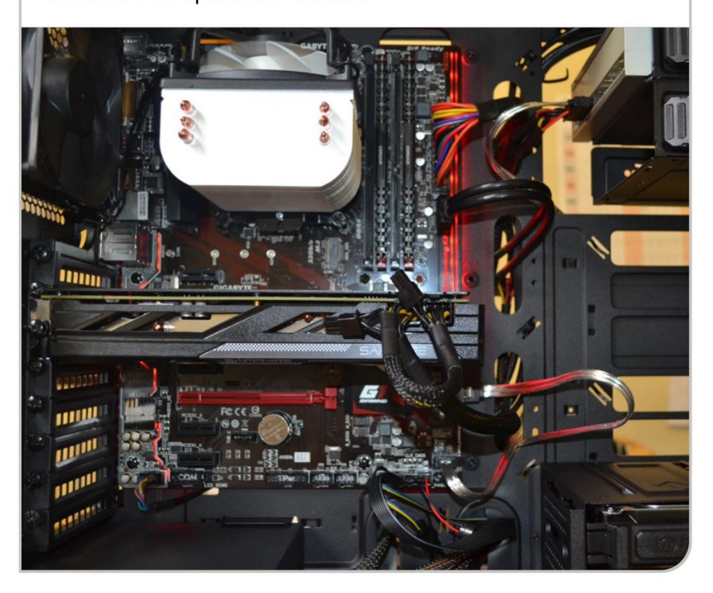
STEP 6 If your case doesn't provide the sort of cable management features we have been talking about here, don't worry, you can still manage the cables. Planning is even more important, as you want as many of the cables as possible running in a single direction. These can then all be gathered together into a bundle, tied up and positioned against the side panel if possible. Not ideal but better than no management!
