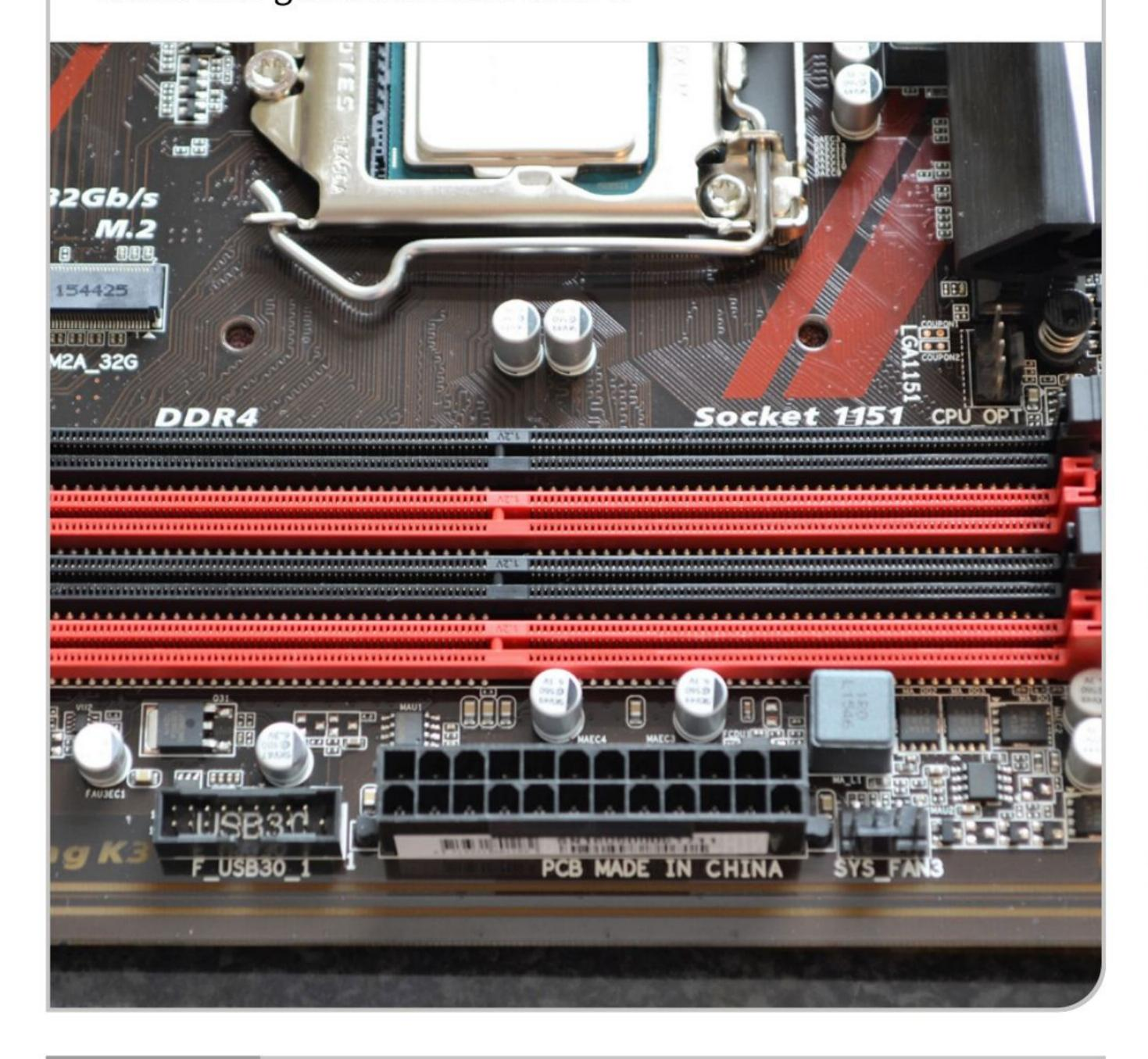
Hold the module at a slightly diagonal angle, so that one end slots into the socket first. Ensure that it is pressed up against the end of the socket and then lower the other end into place. Press firmly and evenly on the top of the module to seat it into the socket. The hinged clips at either end will close, locking the DIMM firmly into place.
