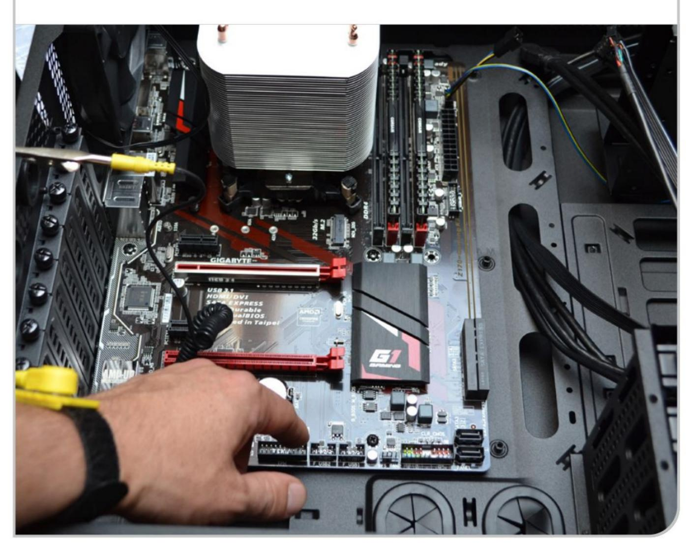
The front USB, audio jacks and case fan connectors are fairly simple to find and connect. The wiring for the power switch, HDD LED and the reset switch might seem a bit more confusing for the first time builder. All of these wires fit onto a single connection on the motherboard; this is just a double row of pins.
