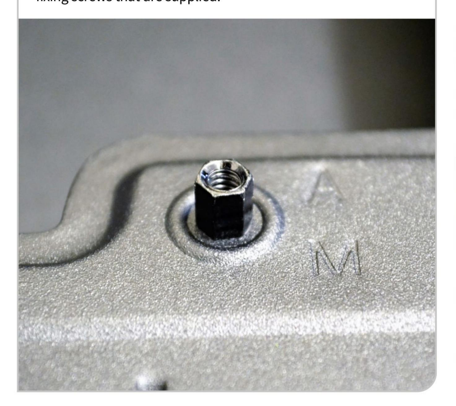
Carefully line up the back panel ports with the back plate holes, press the motherboard against the plate and screw one of the motherboard fixing screws into one of the holes to hold it in place. You can now insert screws into all of the other holes on the motherboard and tighten them carefully. You don't need to apply too much pressure when tightening the screws.
