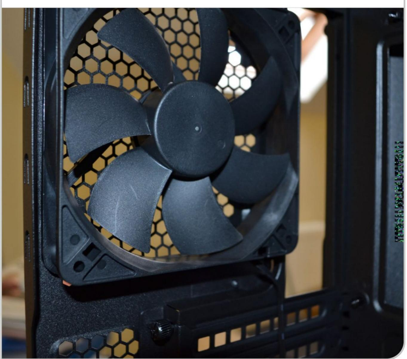
However, if you prefer you can replace the panel before you start adding components. Depending on the case you are using for your build, you might also be able to move or remove the optical drive racks and the hard drive racks, which are usually at the front of the case. Removing unwanted racks can help to increase airflow or just give more room for large components.
