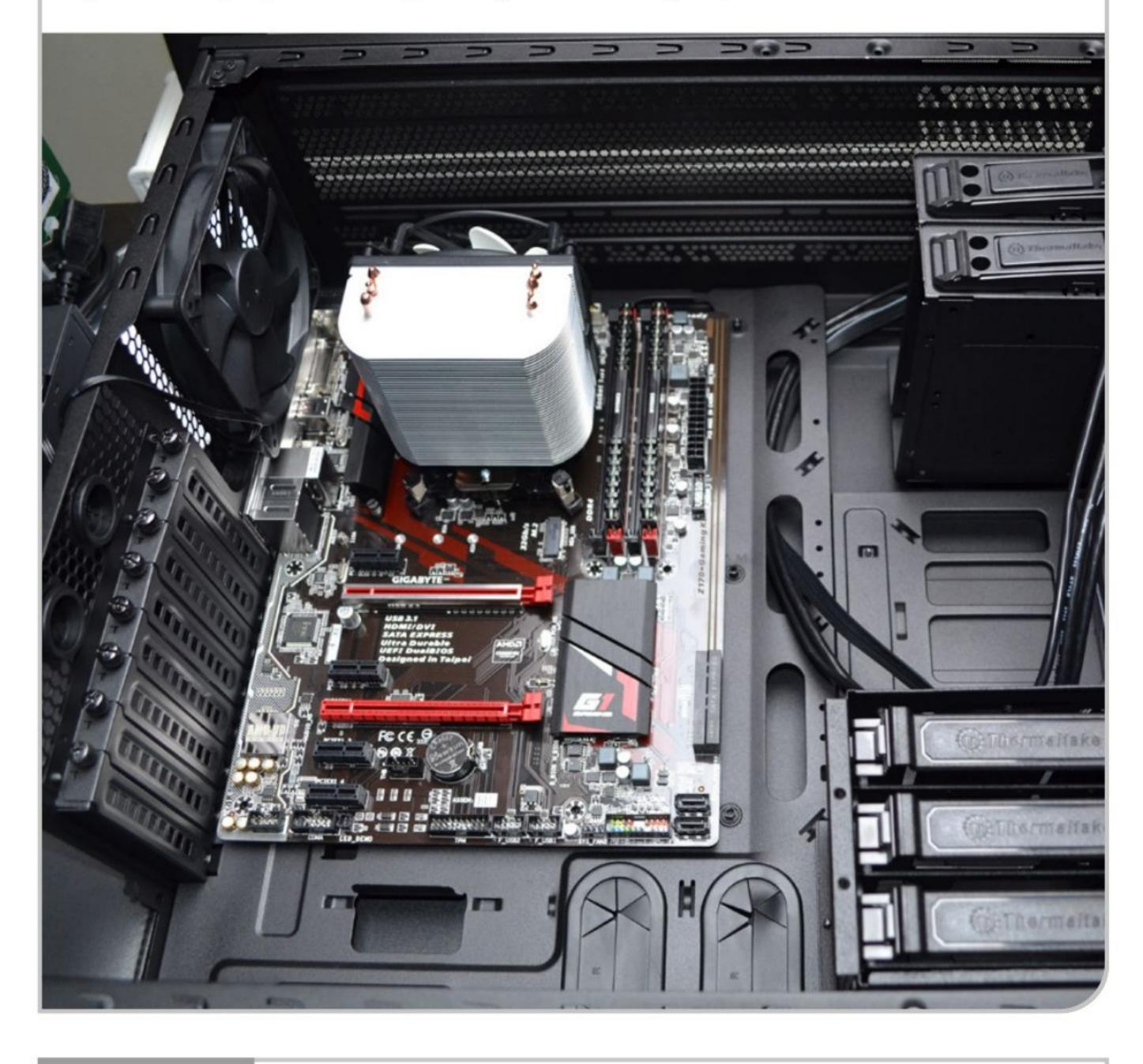
During the preparation of the case, you should have positioned the metal risers in the correct holes based on the form factor of your case and motherboard. Check to see if the holes on the motherboard now line up with your risers and reposition if needed. Identify the motherboard fixing screws that are supplied.
