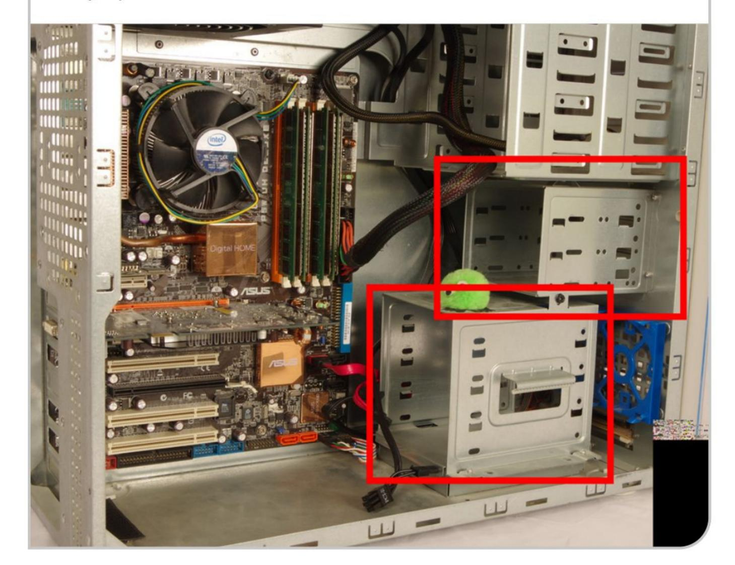
STEP 2 Slide your hard drive onto the rails and line it up with the holes. It needs to have the power and SATA connectors facing out into the case. Use the screws supplied with your case to fix it in place on the open side of the case. You will also need to remove the other case panel, if not already removed and fix it from that side.
