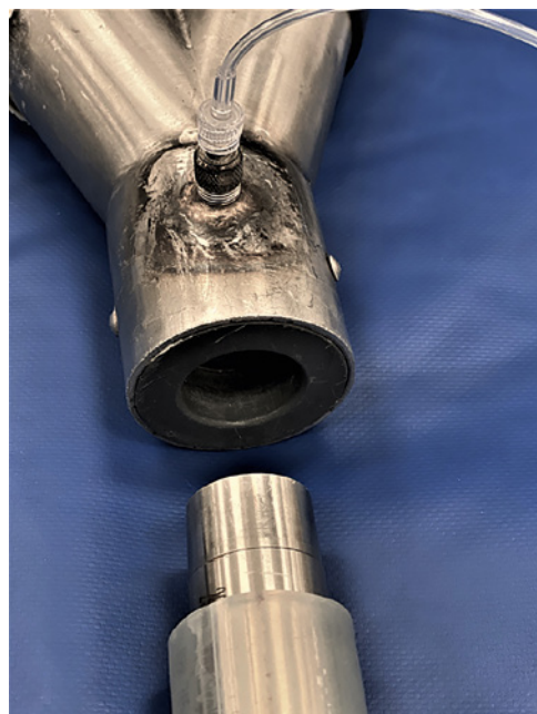
Figure 17.24 Large animal breathing circuit with Bivona insert to facilitate connection to endotracheal tube.
