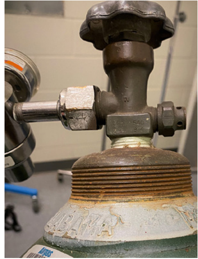
Figure 17.2 Diameter index safety system which is used to ensure connection of correct hose to gas source.
