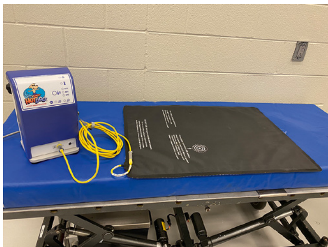
Figure 11.2 HotDog®. A resistive polymer heating device.
