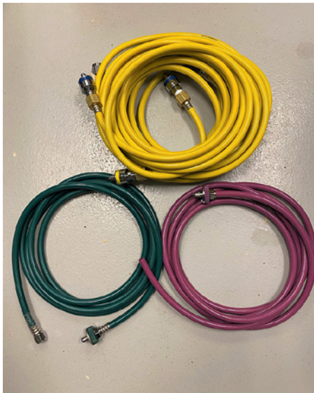
Figure 17.7 Color-coded hosing for gas in the intermediate-pressure zone.
