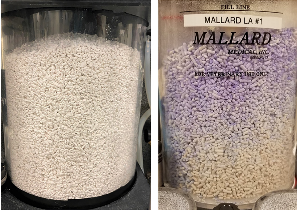
Figure 17.13 Carbon dioxide absorbent in canister. Fresh unused (left) and exhausted with color change (right).
