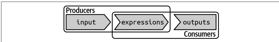
Figure 3-5. Inputs and expressions are reactive producers; expressions and outputs are reactive consumers.
