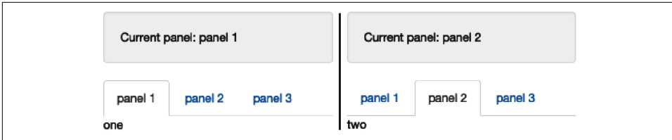
Figure 6-6. A tabset becomes an input when you use the id argument. This allows you to make your app behave differently depending on which tab is currently visible.
