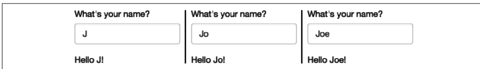
Figure 3-1. Reactivity means that outputs automatically update as inputs change, as in this app where I type: J , o , e . See live at https://hadley.shinyapps.io/ms-connection .
