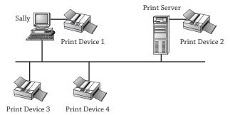
Print device 2 is directly connected to the print server and would be shared by the print server, so it is considered a network printer. Since print devices 3 and 4 are connected directly to the network, they are also considered network printers. Print devices 3 and 4 both must have NICs that can be assigned IP addresses to be accessible on the network.
