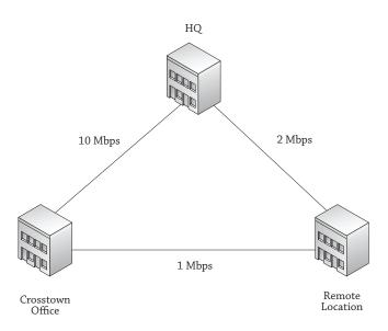
Each physical location is well connected. In other words, all the routers, switches, NICs, and cabling at HQ are capable of transmitting data at 1 Gbps, and all the components at the other two sites support 100 Mbps transfer rates. This is actually the basic definition of a *site*—a group of well-connected hosts or subnets.
