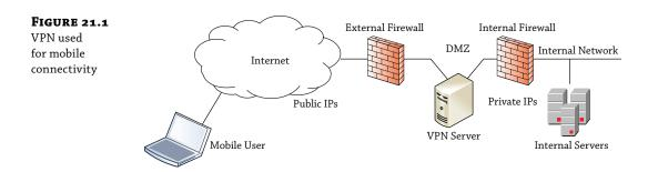
The VPN server has at least two network interface cards (NICs). One NIC has a public IP address and can be reached by any user who has access to the Internet. The other NIC has a private address connected to the internal network.
