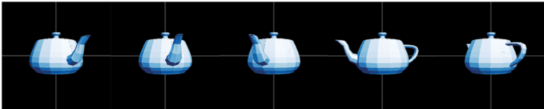
Figure 5.4 The teapot is transformed by a new matrix in every frame, depending on the elapsed time when the frame is drawn.
