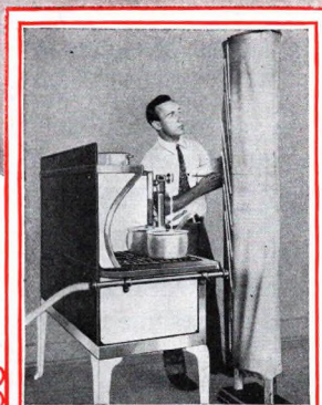
(At left) Thermometer-covered "dummy" proves that open-top ranges cause least heat-discomfort. Picture taken in American Stove Company's Research Laboratory at St. Louis, Mo.
