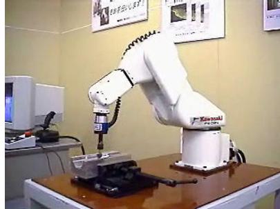
Figure 1.18. Mold-polishing robot developed based on KAWASAKI FS03
