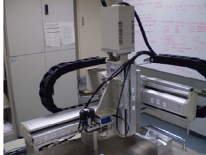
Figure 1.21. Cartesian-type robot with compliant motion capability
