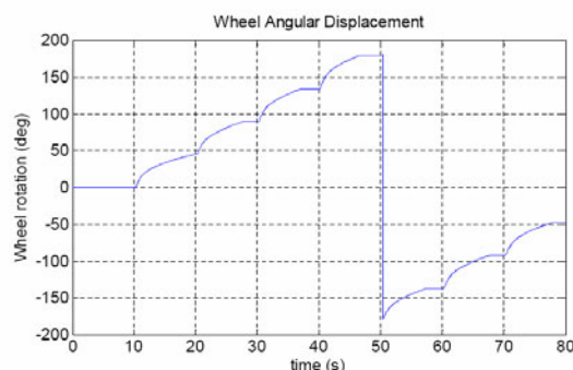
Figure 2.18. Motor shaft angular displacement for a four IPMC stepper motor [MCD 10a]
