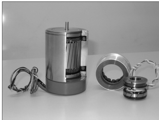
Figure 3.5. Traditional resolver (left) and pancake resolver (right)
