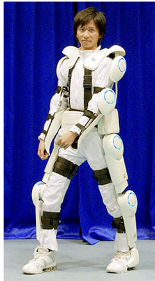
Figure 7.4. A student demonstrating the HAL-5 powered exoskeleton [UBE 07]
