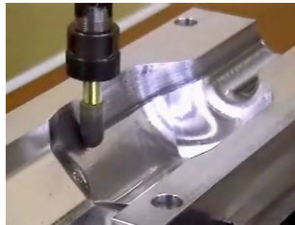
Figure 1.19. Polishing scene of PET bottle mold
