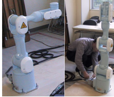
Figure 1.8. Open architecture industrial robot Mitsubishi PA10
