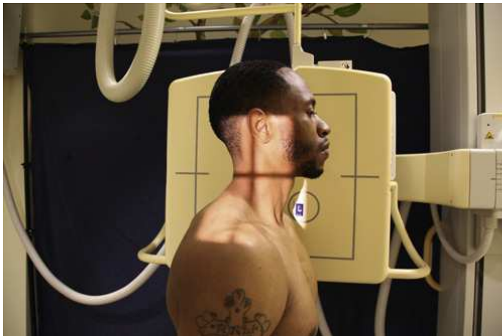
FIG. 1.16 A vertical Bucky unit contains a reciprocating grid to reduce scattered radiation reaching the IR.
