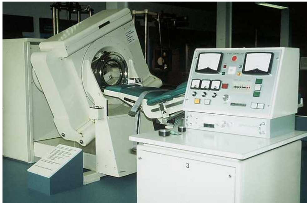
FIG. 25.6 First-generation EMI CT unit: dedicated head scanner. Photograph taken at Reöntgen Museum, Lennep, Germany.
