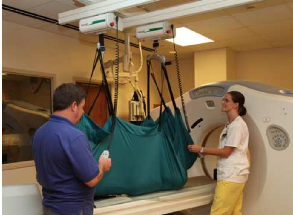
FIG. 1.53 Twin 500-lb capacity power lifts, attached to a ceiling-mounted rail system, allow very large patients to be safely lifted from a bed or a stretcher to the 650-lb capacity CT table. Interdepartmental cooperation is essential because the hoist sling is usually positioned under the patient before transport to the CT suite. Courtesy Department of Radiology, St. Vincent Carmel Hospital, Carmel, IN.
