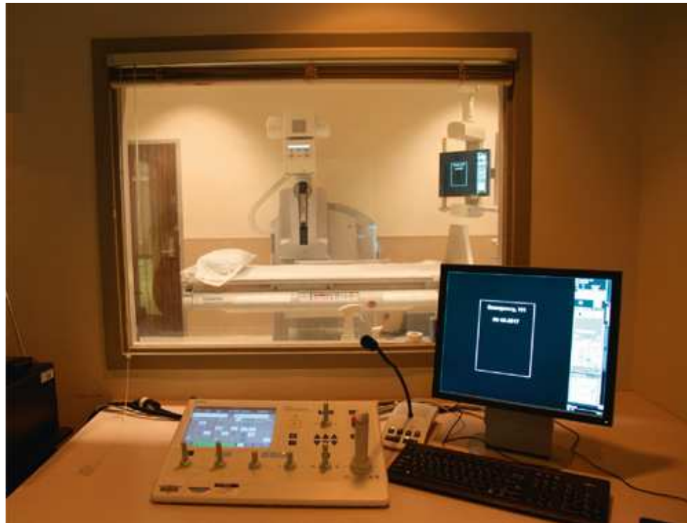
FIG. 15.41 Remote control fluoroscopic room, showing patient fluoroscopic table ( background ) and fluoroscopist's control console ( foreground ). The fluoroscopist views the patient through the large window.
