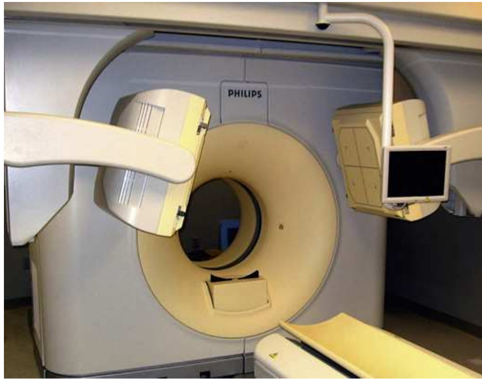
FIG. 29.2 Combined single photon emission computed tomography/computed tomography camera for a blending of imaging function and form.
