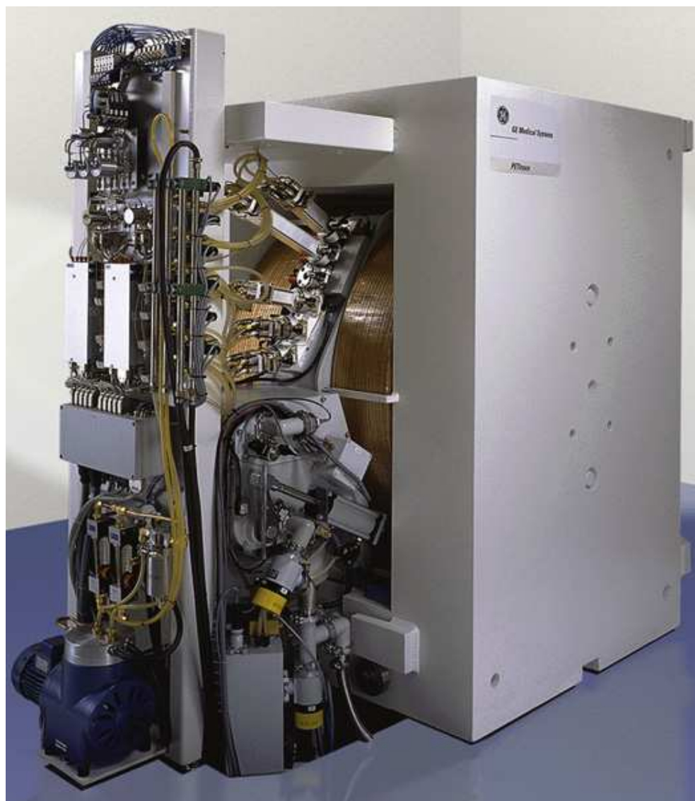
FIG. 29.25 Compact cyclotron (2.2 m high \times 1.5 m wide \times 1.5 m deep) used for routine production of PET isotopes. Cyclotron can be located in a concrete vault, or it can be self-shielded. Particles are accelerated in vertical orbits and impinge on targets located near the top center of the machine. This is an example of a negative-ion cyclotron. Courtesy GE Medical Systems, Milwaukee, WI.
