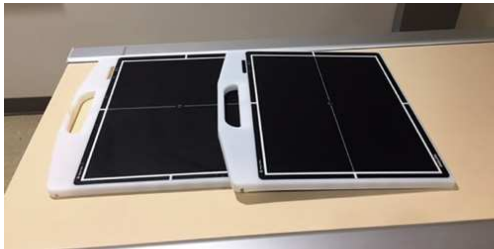
FIG. 20.5 The directions of the grid lines are marked on the front of the grid as either transverse ( short dimension ) or longitudinal ( long dimension ). Focal ranges are clearly identified for proper use.
