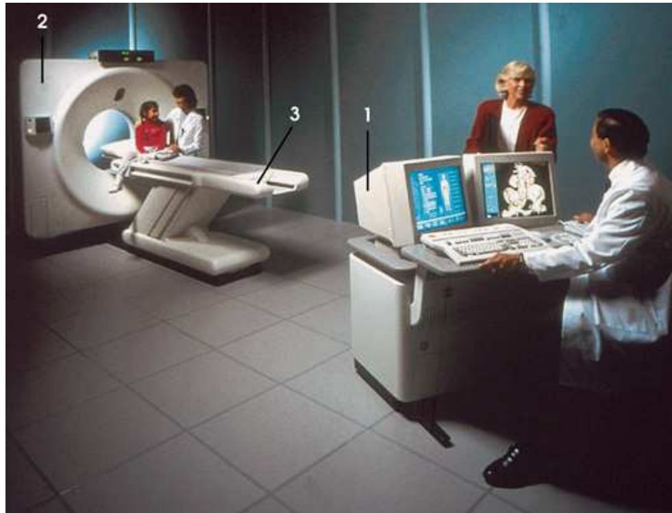
FIG. 25.13 Components of a CT scanner: 1, Computer and operator's console; 2, gantry; 3, patient table. Courtesy GE Medical Systems, Waukesha, WI.
