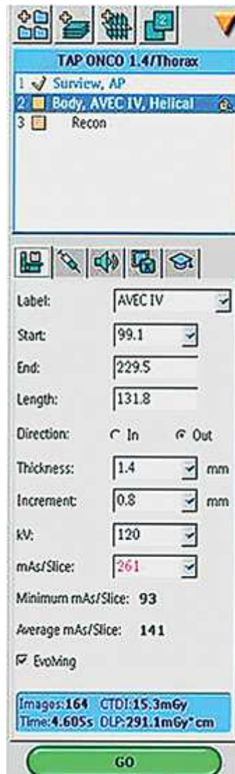
FIG. 25.51 Dose amounts must be reported for every series and protocol performed. Each manufacturer displays information differently. Note CTDI and DLP displayed inside the blue box . Courtesy Philips Medical Systems.
