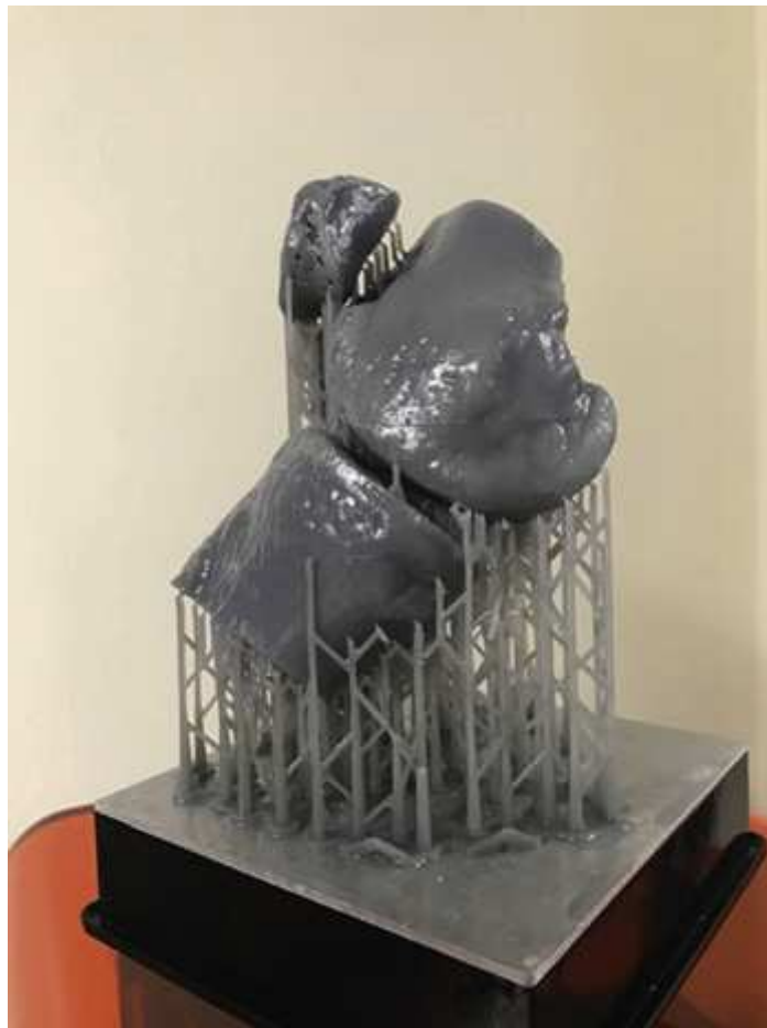
FIG. 24.71 3D printed model of the knee with structural supports still in place. From Weber State University, School of Radiologic Sciences.
