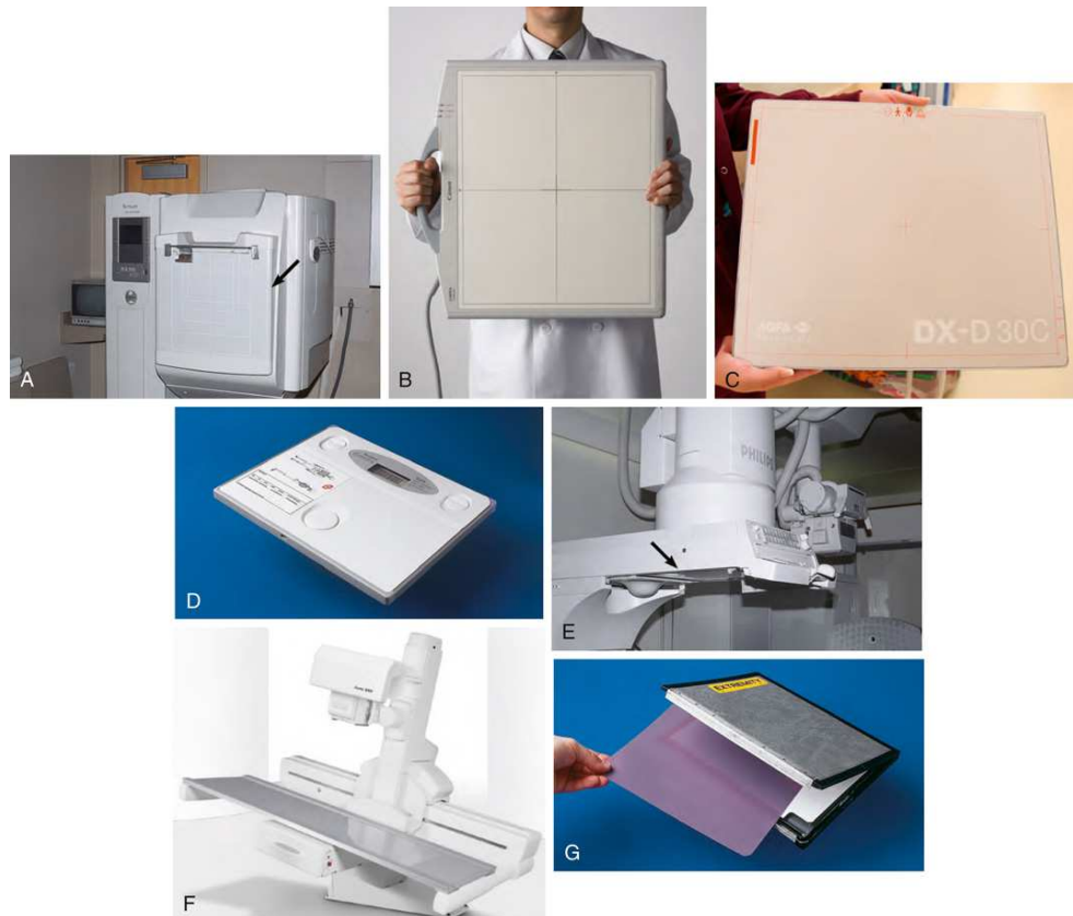
FIG. 1.13 Image receptors. (A) DR upright wall unit. A flat-panel digital detector is located behind the front cover ( arrow ). (B) Tethered portable DR IR. (C) Wireless portable DR IR. (D) CR cassette. This contains a photostimulable storage phosphor image plate that stores the x-ray image. (E) Fluoroscopic image intensifier unit located under fluoroscopic tower ( arrow ) transmits x-ray image to a camera and then to a television for real-time viewing. (F) Fluoroscopic solid-state flat-panel digital detector transmits image directly to viewing monitor without the need for an intermediate video camera. (G) Conventional radiographic cassette, opened and showing a sheet of x-ray film. F, Courtesy Canon USA, Inc. G, Used with permission from Philips Healthcare, Bothell, WA.
