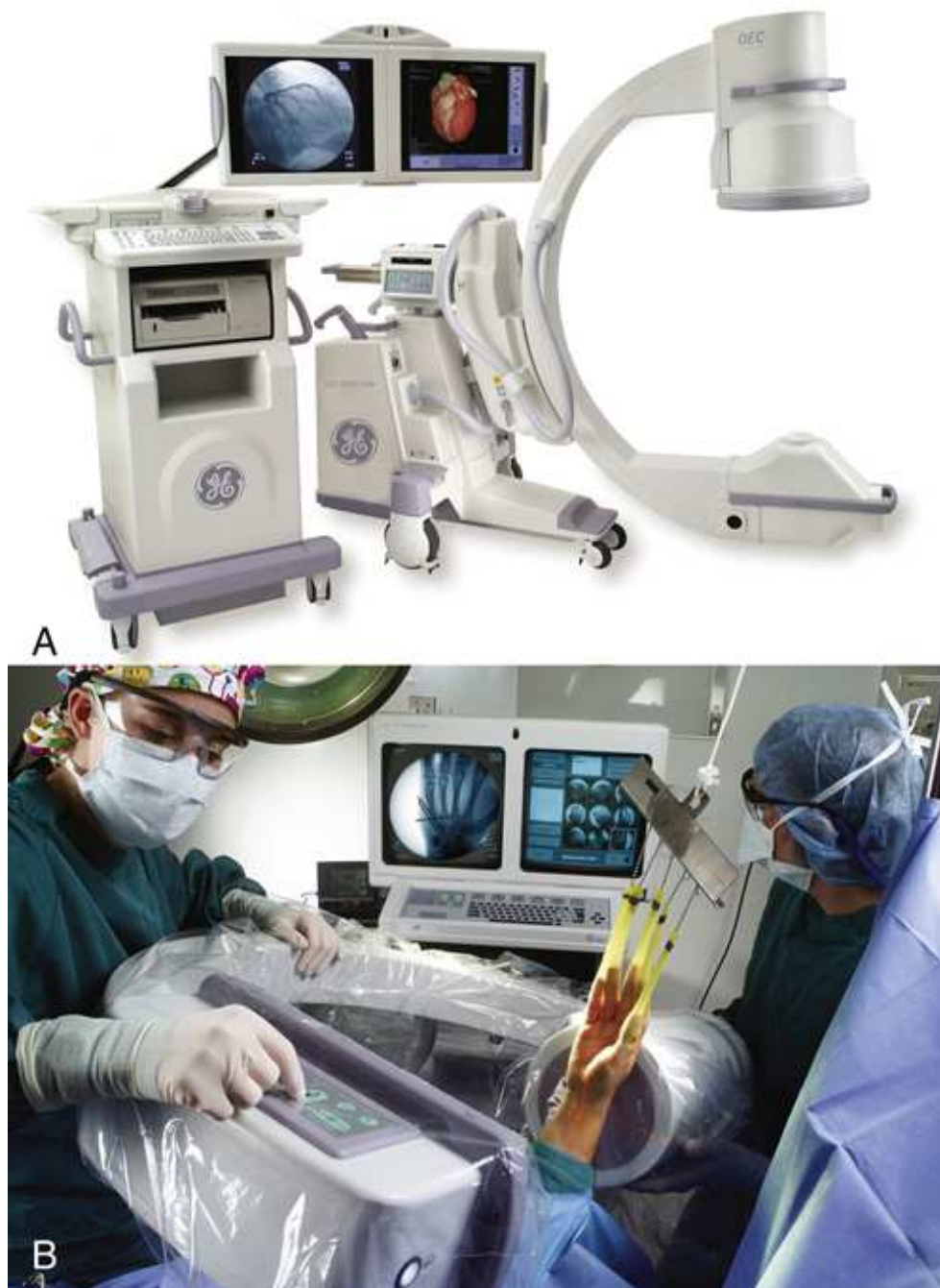
FIG. 21.8 (A) C-arm radiographic/fluoroscopic system used in the OR. (B) Mini-mobile C-arm used for extremity examinations in the OR.
