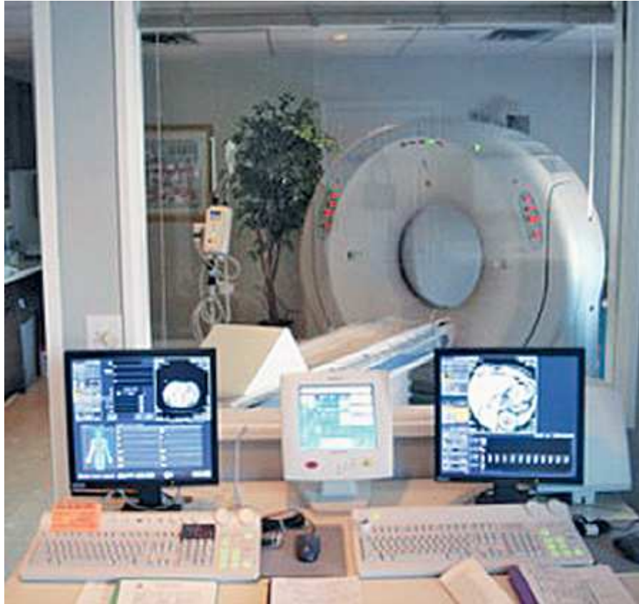
FIG. 25.15 CT operator's console, workstation for three-dimensional image manipulation, and power injector control panel.
