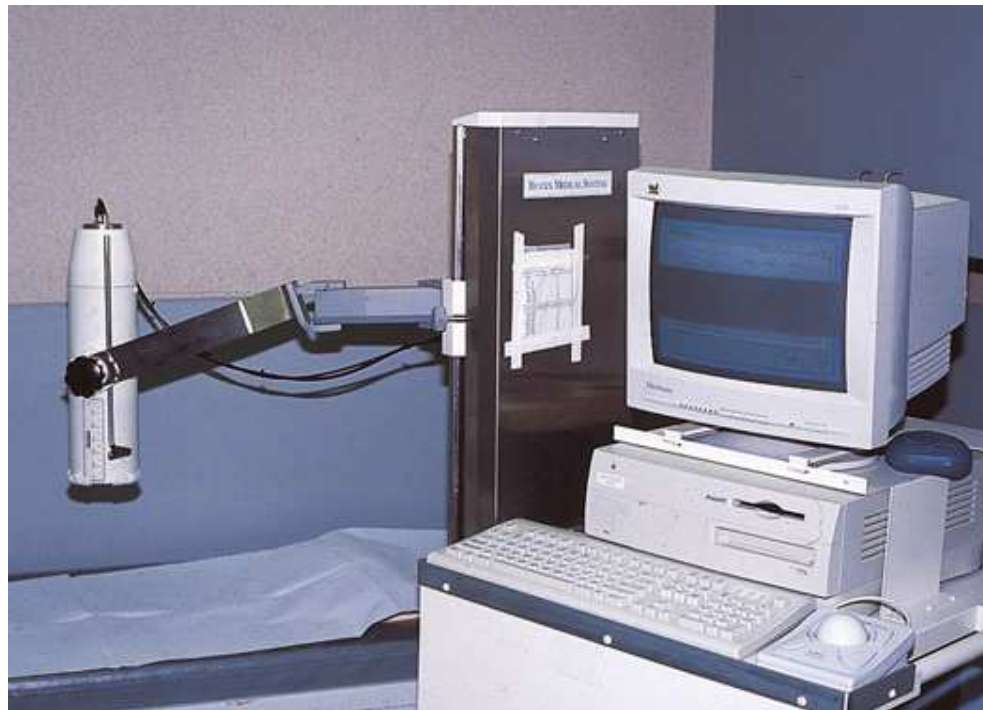
FIG. 29.19 Uptake probe used for thyroid uptake measurements over the extended neck area.
