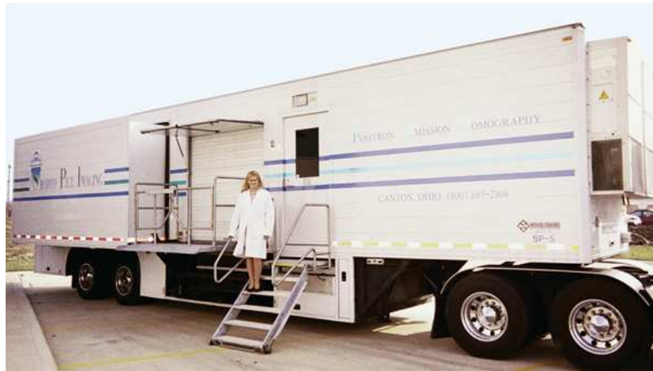
FIG. 29.43 Mobile PET coach showing operator on staff stairs and elevator platform in the elevated position. Elevator used to transport patients from ground level to floor level of the PET scanner unit. Courtesy Shared PET Imaging, LLC.
