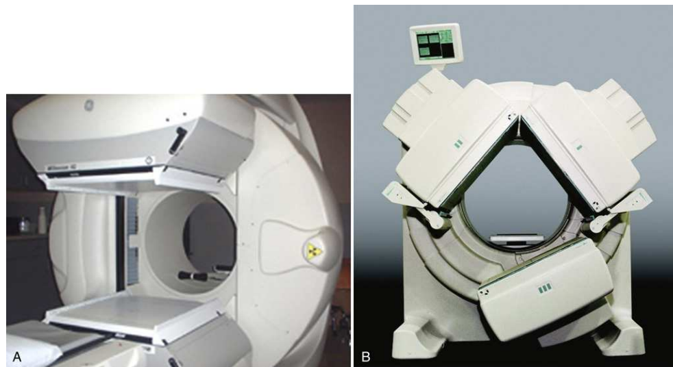
FIG. 29.16 SPECT camera systems. (A) Dual-headed SPECT/CT system. (B) Triple-headed system. B, Courtesy Marconi Medical Systems.
