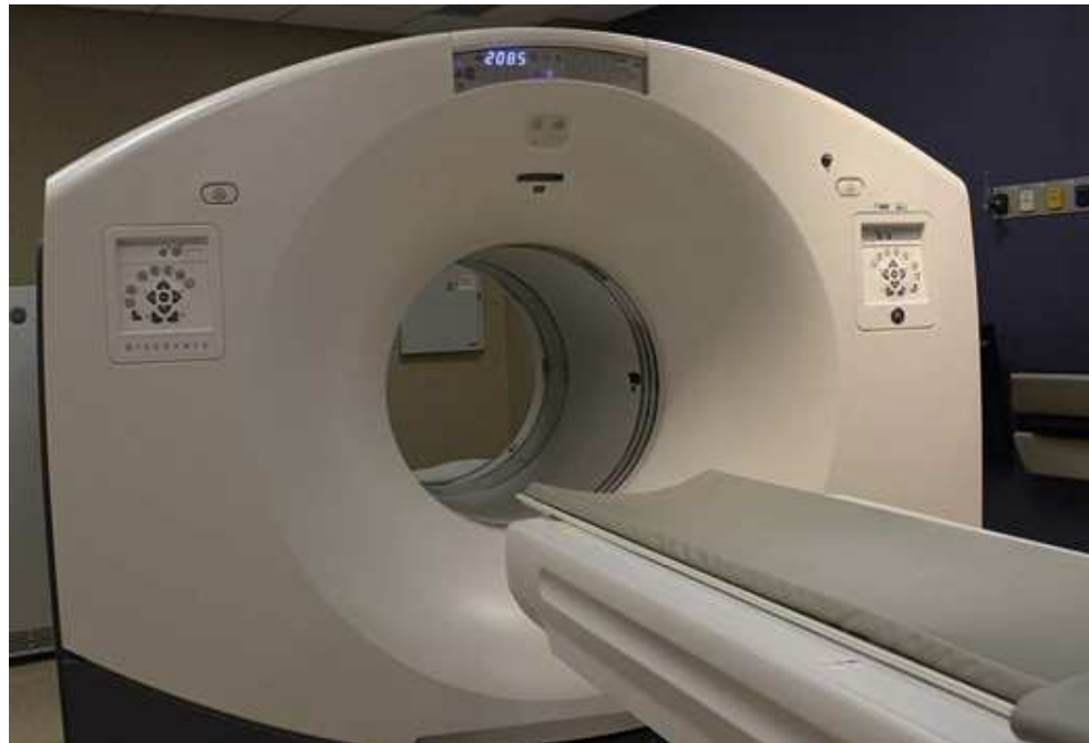
FIG. 29.31 Typical whole-body PET/CT scanner. The bed is capable of moving in and out of the scanner to measure the distribution of PET radiopharmaceuticals throughout the body, and it adjusts to a very low position for easy patient access. Sophisticated computer workstations are required to view and analyze data.
