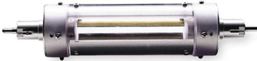
FIG. 19.8 Calibration drum used as internal reference standard in Hologic energy-switching instruments. Different segments represent bone standard, soft tissue standard, and empty segment for air value.
