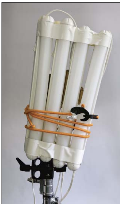
This is my gaffer's-tape and bungie-cord solution to creating a fluorescent light bank. These tubes are "balanced" for tungsten, but that's hardly accurate. I would say they are balanced for green ick.
