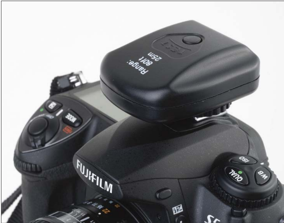
This is an inexpensive radio transmitter used instead of a PC cable to trigger flash units.
