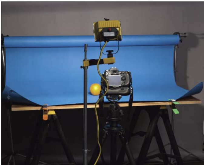
Our main light is positioned right next to our camera and aimed at the orange without modification.
