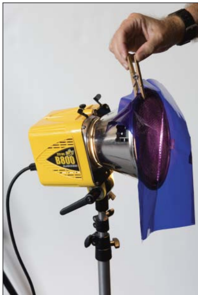
Adding a blue filter to the background light.
