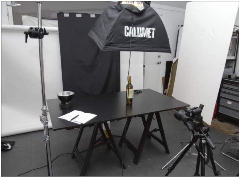
Most product shots begin with a softbox suspended over the top of the set.
