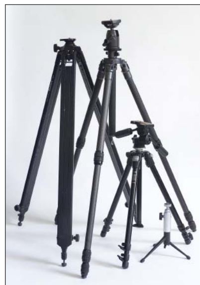
Choose the right tripod for the job. We use the short one when we need to be low and the wooden one when we need something that won't freeze or burn our hands when used outdoors. For everything else we use the Gitzo. It's an old three-series "performance" carbon-fiber model with a cheap Canon ball head on top.
