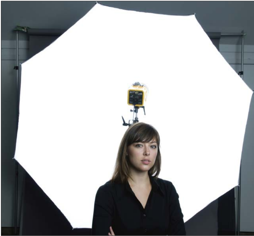
This is my budget answer to the famous Octabank made by Elinchrome. This Lastolite 80-inch softbox comes with its own front diffusion already in place.
