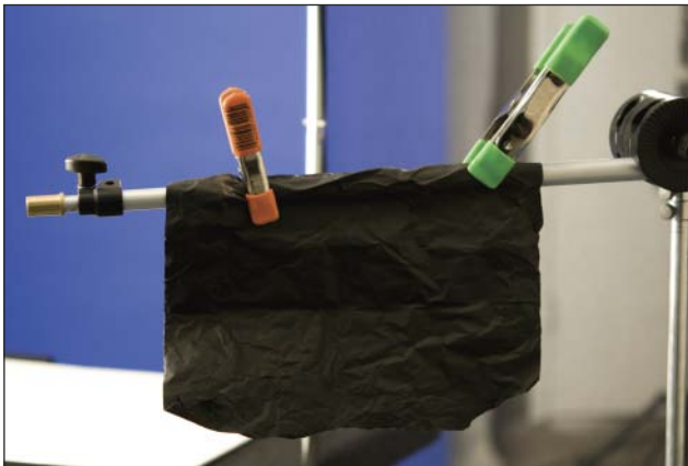
We use black wrap as lens shades, snoots, gobos, and anything else requiring a flexible opaque material.
