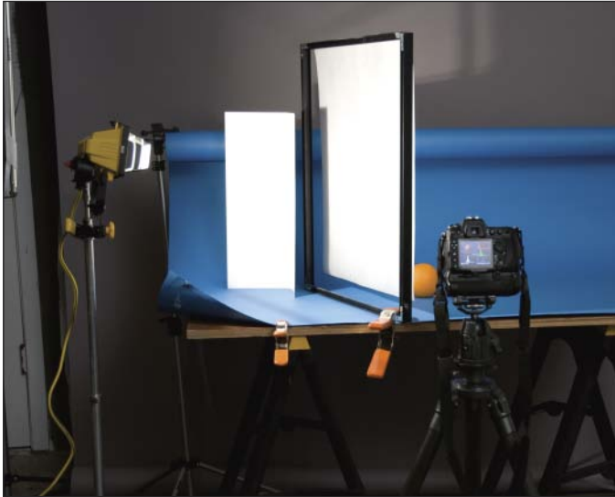
We use pieces of cardboard to block the light sneaking around the edges of the diffusion frame.
