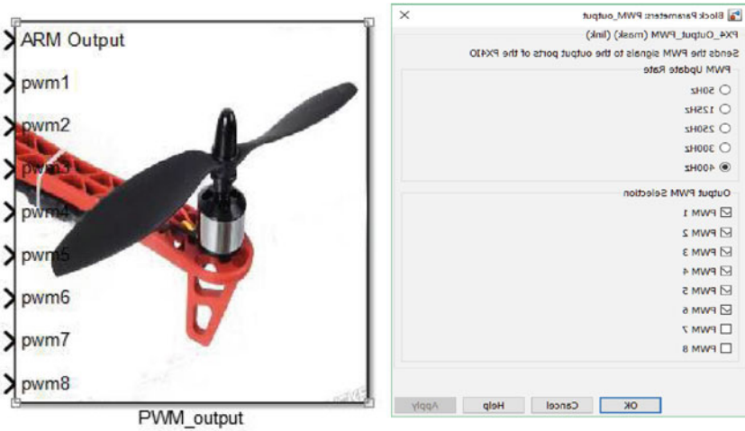
Fig. 21 PWM SIMULIK generator for Pixhawk
