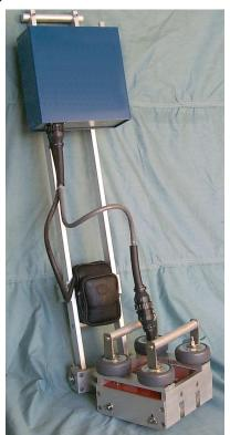
leakage is caused by top or bottom indications. For uncoated materials, the top discontinuities can be verified during a simple visual test. Other methods such as ultrasonic testing are performed for coated floors.
