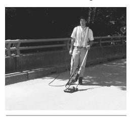
acquisition at consistent intervals. The series of individual waveforms collected along the path of the radar antenna can be viewed collectively as a synthetic aperture. Raw data collected using a ground coupled ground penetrating radar are presented over a two-dimensional synthetic aperture (Fig. 9).
