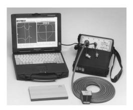
technique. Potential drop testing has been used for crack sizing and crack growth monitoring for underwater applications such as offshore platforms. The alternating current field measurement technique is simple, relying on the measurement of surface magnetic fields instead of surface electric fields, thus requiring no electrical contact. This reliance on magnetic fields allows the technique to be used through coatings up to 6 mm (0.25 in.).<sup>6</sup>
