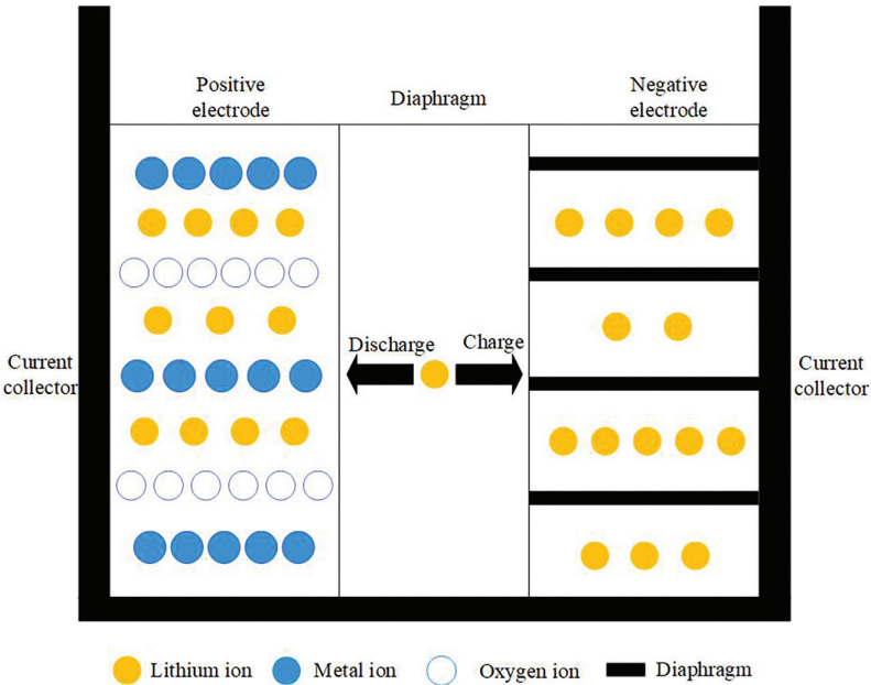
FIGURE 1.1 Schematic diagram of the lithium-ion battery structure.
