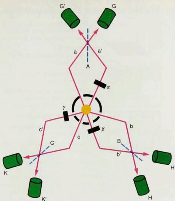
**Three-particle interferometer.** A particle at the center decays into three daughters of equal mass and momentum. Collimation restricts the decay state to beams  $a$ ,  $b$  and  $c$  or  $a'$ ,  $b'$  and  $c'$ . The primed beams pass through phase shifters (black rectangles) with phase shifts  $\alpha$ ,  $\beta$  and  $\gamma$ , respectively, after which the alternative paths are mixed at beam splitters  $A$ ,  $B$  and  $C$  before arriving at three pairs of detectors (green). **Figure 7**
