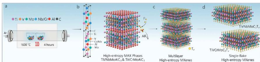
**FIGURE 4.3** (a) Schematic of synthesis process of HE  $(TiVNbMo)AlC_3$  and  $(TiVCrMo)AlC_3$  MAX phases, (b) distribution of atoms on unit cell for the corresponding HE-MAX phases, (c) multilayer HE MXenes with surface functional groups, and (d) single-flake  $(TiVNbMo)C_3$  and  $(TiVCrMo)C_3$  MXenes after delamination by organic molecules.
