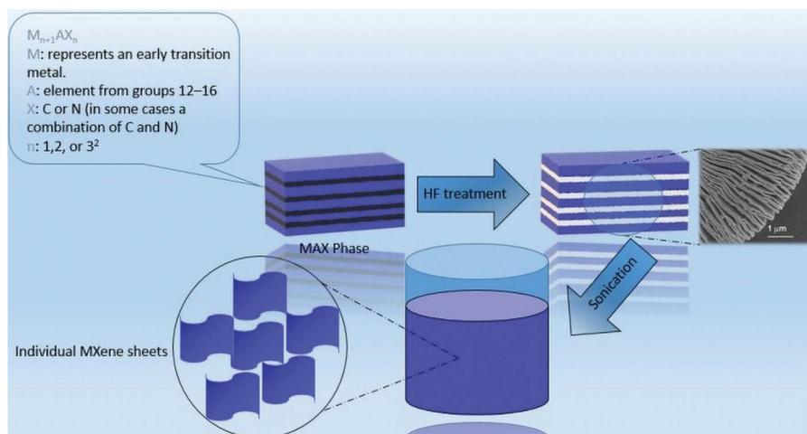
**FIGURE 6.2** Schematic diagram of exfoliation of 'A' layer from MAX phase to obtain MXene using the HF treatment.
