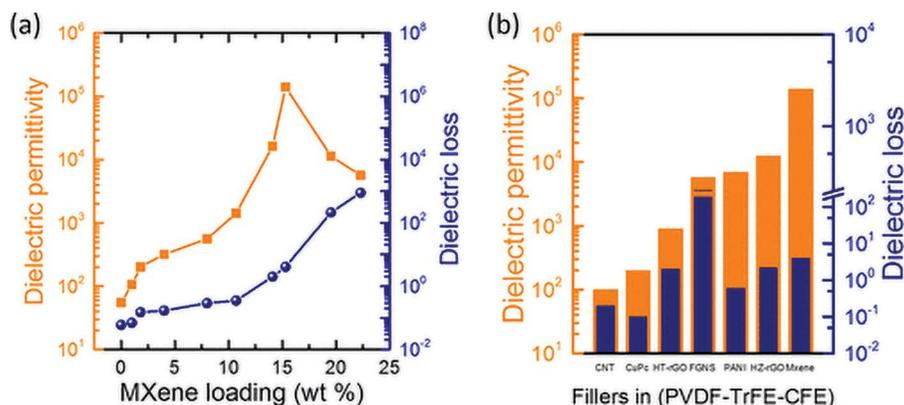
**FIGURE 5.5** (a) Permittivity and dielectric loss of MXene/P(VDF-TrFE-CFE) at room temperature and 1 kHz; (b) bar charts comparing maximum dielectric permittivity and dielectric loss for P(VDF-TrFE-CFE) with different conductive fillers.
