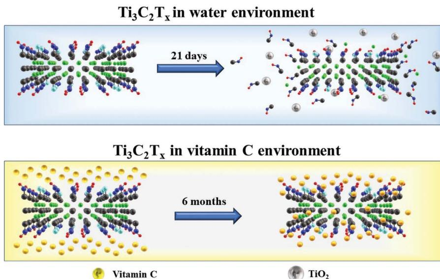
**FIGURE 3.4** The mechanisms of Ti<sub>3</sub>C<sub>2</sub>T<sub>x</sub> MXene protection with L-ascorbic acid antioxidant.
