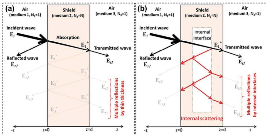
**FIGURE 7.3** Mechanisms of EMI shielding of MXenes. (a) An ultrathin shield thickness and (b) induced inclusions or interfaces inside the shield playing as scattering sites within the shield.
