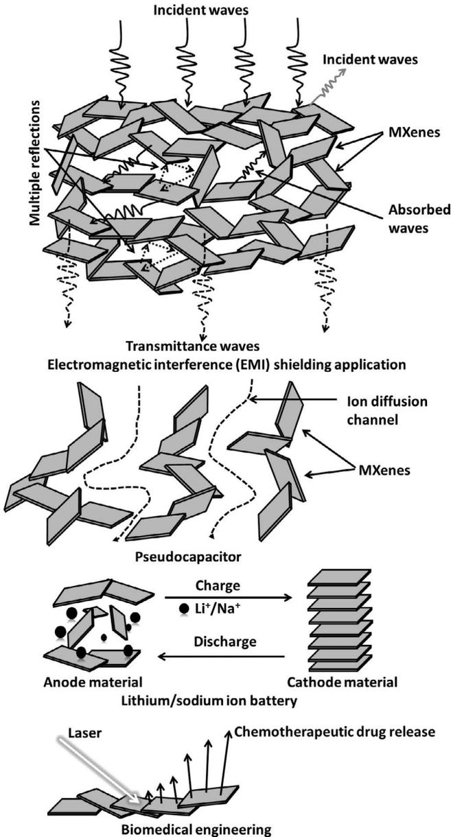
**FIGURE 8.1** Various applications of MXenes-based porous structures.
