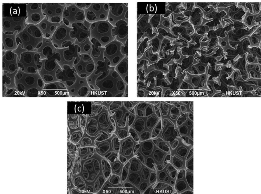
**FIGURE 11.2** Scanning electron microscopic (SEM) images of (a) non-auxetic PU (NAPU), (b) APU and (c) OPU.
