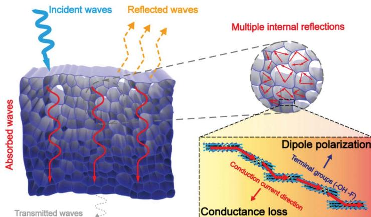
**FIGURE 8.12** Hybrid aerogel's plausible EMI shielding mechanism.
