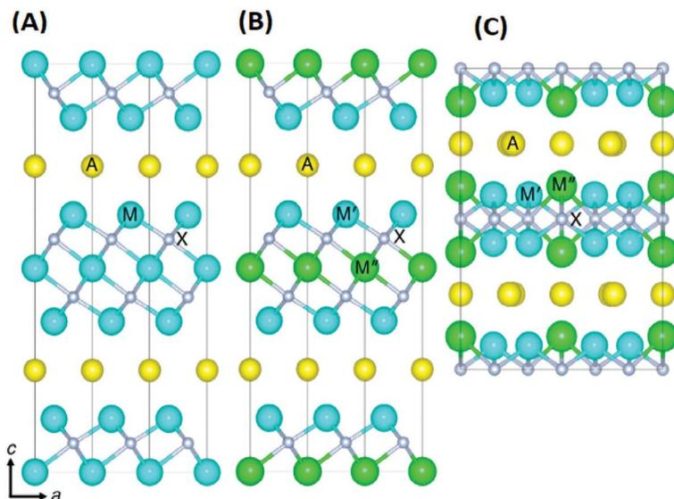
**FIGURE 1.3** Crystal structure of (A)  $M_3AX_2$ , (B) out-of-plane ordered double-transition metal  $M'_2M''AX_2$  and (C) in-plane ordered double-transition metal  $(M'_{2/3}M''_{1/3})_2AX$ . Solid line indicates the border of the unit cell.
