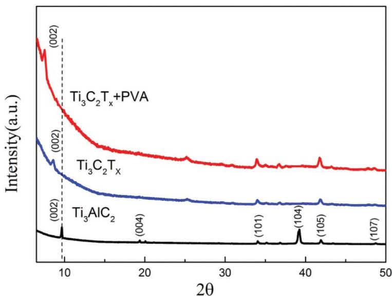
**FIGURE 6.5 (b)** XRD patterns of  $\text{Ti}_3\text{AlC}_2$ ,  $\text{Ti}_3\text{C}_2\text{T}_x$  flakes and  $\text{Ti}_3\text{C}_2\text{T}_x/\text{PVA}$  NCs.
