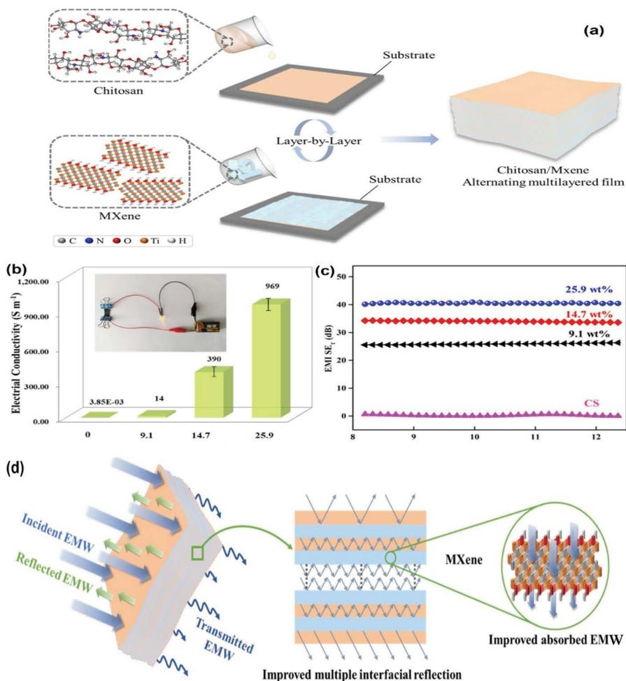
**FIGURE 12.8** (a) Schematic representation of the fabrication process of CS/MXene multilayered film using LBL assembly strategy; (b) electrical conductivity of CS/MXene films with the change of MXene fraction; (c) EMI shielding curves of neat CS and CS/MXene films in X band; (d) schematic illustration of the EMI shielding mechanism.
