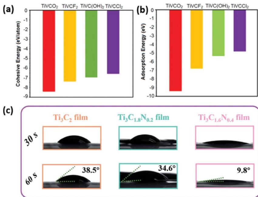
**FIGURE 4.5** (a) and (b) DFT calculated cohesive energies and adsorption energies for TiVC MXene functionalized by O, F, OH, and Cl. (Reproduced with permission from Ref. [33], © (2020) American Chemical Society.) (c) shows the contact angle of 1 M KOH electrolyte with Ti<sub>3</sub>C<sub>2</sub>, Ti<sub>3</sub>C<sub>1.8</sub>N<sub>0.2</sub>, and Ti<sub>3</sub>C<sub>1.6</sub>N<sub>0.4</sub> MXenes films and reveals that film becomes hydrophilic when N concentration increases [42].
