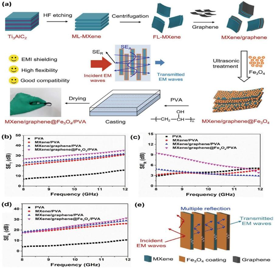
**FIGURE 12.5** (a) Schematic of synthesis and mechanism of EMI shielding of MXene/graphene@Fe<sub>3</sub>O<sub>4</sub>/PVA film; (b) SE<sub>T</sub>, (c) SE<sub>R</sub>, (d) SE<sub>A</sub> of PVA and PVA composite films; (e) illustration of shielding mechanism in MXene/graphene@Fe<sub>3</sub>O<sub>4</sub> ternary composites.
