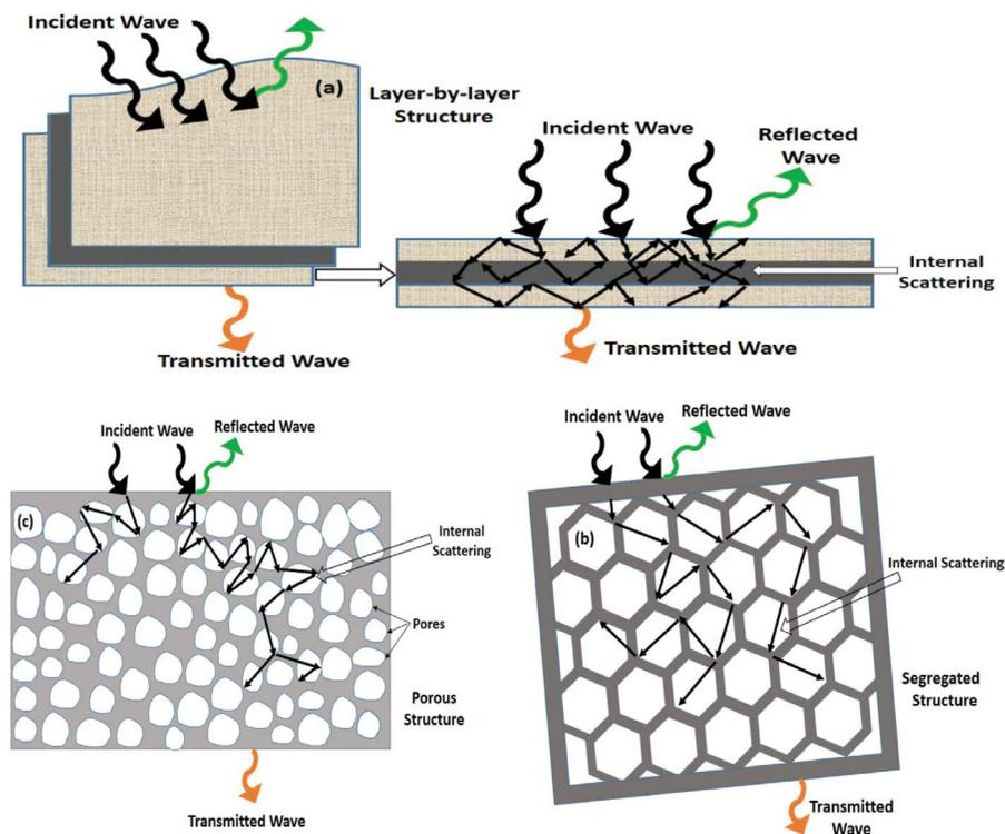
**FIGURE 12.3** Architectures for MXene composites and hybrids that promote the internal multiple scattering: (a) layer-by-layer structure, (b) segregated structure, (c) porous structure.
