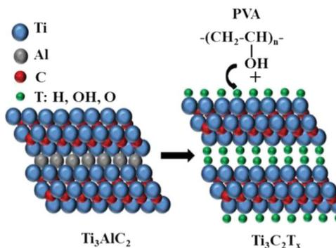
**FIGURE 6.5 (a)** Schematic illustration of synthesis process of  $\text{Ti}_3\text{C}_2\text{T}_x/\text{PVA}$  NCs.
