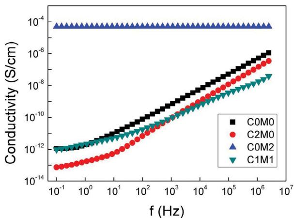
**FIGURE 6.6** Graph of DC conductivity vs. frequency at 20°C for the  $\text{Ti}_3\text{C}_2\text{T}_x/\text{CNC}/\text{PVA}$  samples with varying ratios and compositions.
