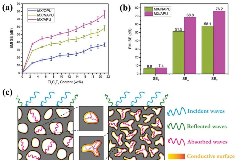
**FIGURE 11.3** (a) EMI shielding efficiency study of MX/APU, MX/NAPU and MX/OPU; (b) comparison of different components ( $SE_A$ ,  $SE_R$ ) of total EMI shielding efficiency ( $SE_T$ ) for MX/NAPU and MX/APU; (c) attenuation of EMI shielding performance of foam composites with different pore structures.
