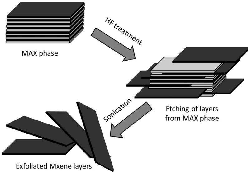
**FIGURE 2.1** Schematic illustration of MXenes synthesis via HF etching method.
