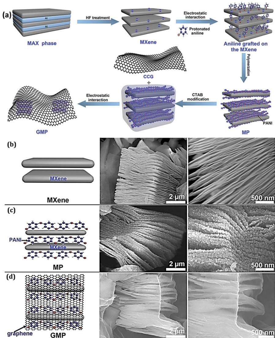
**FIGURE 5.6** (a) The overall process of producing GMP as a diagram. Schematic illustrations and SEM images of (b) MXene Ti<sub>2</sub>CTx, (c) MP, and (d) GMP.
