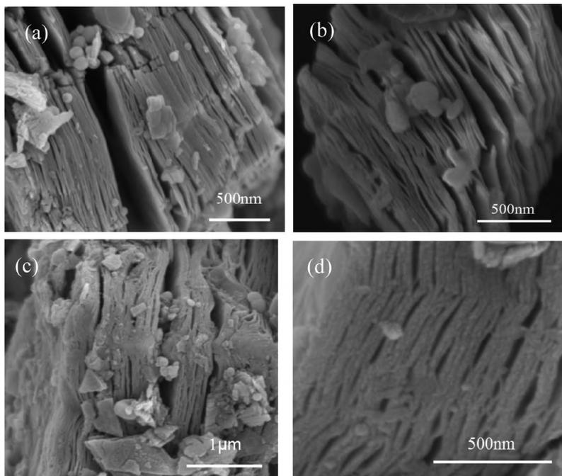
**FIGURE 6.7** SEM images of (a)  $\text{Ti}_3\text{C}_2\text{T}_x$  MXene, (b) zoomed in view of  $\text{Ti}_3\text{C}_2\text{T}_x$ , (c)  $\text{Ti}_3\text{C}_2\text{T}_x/\text{PVA}$ , (d) zoomed in view of  $\text{Ti}_3\text{C}_2\text{T}_x/\text{PVA}$ .
