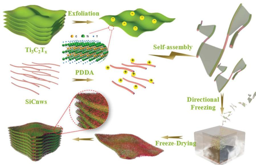
**FIGURE 8.3** Diagram depicting the production of f- $\text{Ti}_3\text{C}_2\text{T}_x/\text{SiC}$  nanowire hybrid foams in three dimensions.
