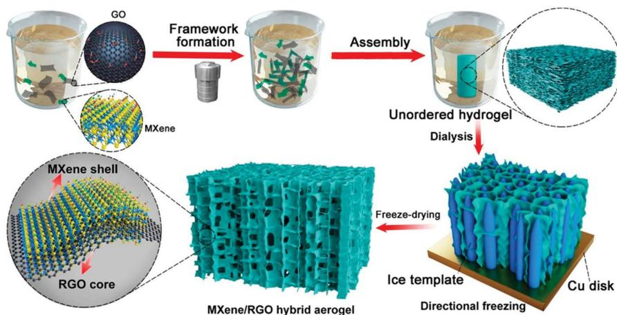
**FIGURE 5.3** Schematic showing  $\text{Ti}_3\text{C}_2\text{T}_x$  MXene/RGO hybrid aerogel fabrication via GO-assisted hydrothermal assembly, directional freezing, and freeze-drying.
