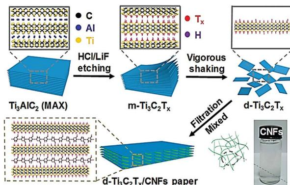
**FIGURE 5.4** HCl and LiF etch Ti<sub>3</sub>AlC<sub>2</sub> (MAX) to produce m-Ti<sub>3</sub>C<sub>2</sub>T<sub>x</sub>. Under vigorous shaking, m-Ti<sub>3</sub>C<sub>2</sub>T<sub>x</sub> sediment is disseminated in deionized water to produce d-Ti<sub>3</sub>C<sub>2</sub>T<sub>x</sub> nanosheets. Then CNFs are added to d-Ti<sub>3</sub>C<sub>2</sub>T<sub>x</sub>. The d-Ti<sub>3</sub>C<sub>2</sub>T<sub>x</sub>/CNF composite paper is made from a 24-h-stirred suspension.
