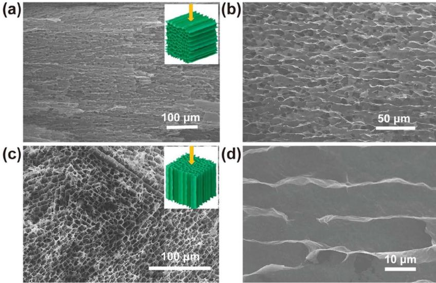
**FIGURE 11.5** (a, b, d) Side view of SEM images of the aerogel MS 74, (c) top view of the SEM images of the aerogel MS 74.
