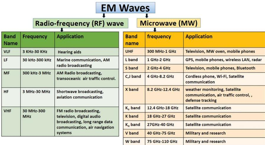
FIGURE 12.1 Application of different RF and MW frequency ranges of EM radiation.
