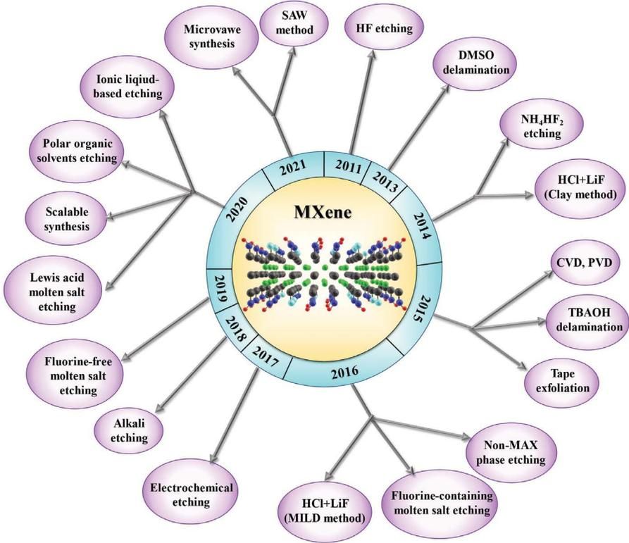
**FIGURE 3.2** A schematic presenting an outstanding effort to develop the universal synthesis and delamination technique for the most recognized  $Ti_3C_2Tx$  MXene phase.
