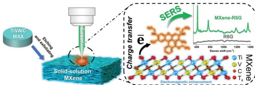
**FIGURE 4.8** A schematic of producing TiVC MXenes from their parent MAX phase and then using these MXenes as a substrate for R6G SERS measurement using a laser of 532 nm wavelength. Raman spectra show a huge enhancement in the intensity when MXene was used as a substrate for R6G.
