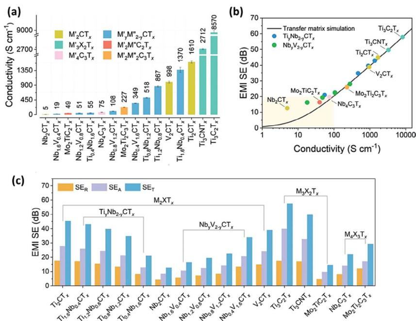
**FIGURE 7.4** (a) Electrical conductivity of different MXenes; (b) comparison of the EMI SE of different MXene films, each of 5 μm of thickness; (c) average EMI SE values of different MXene films over the 8.2–12.4 GHz frequency range.
