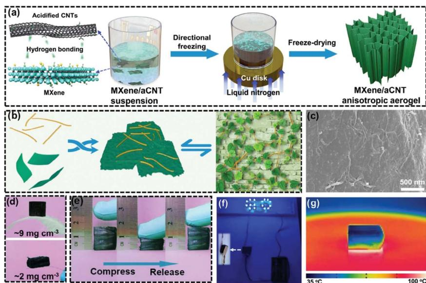
**FIGURE 8.5** (a) Preparation of an MXene/aCNT aerogel; (b) MXene nanosheets and aCNTs bionic assembly; (c) MXene/aCNT microstructure in SEM picture of MCA; (d) MCA on feather (top) and strand of hair (bottom); (e) 50% strain reversible MCA-1 compression–release method; (f) electrically conductive MCA-1 LEDs; (g) thermographic picture of a 9 mm cuboid MCA-1 heated to  $100^\circ\text{C}$ .
