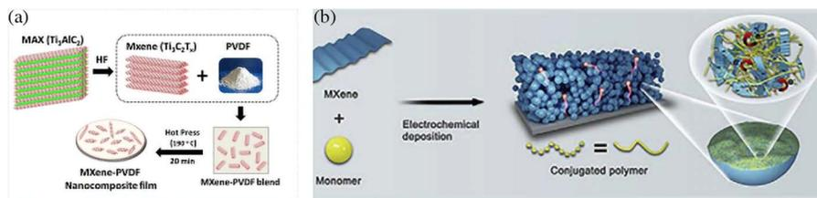
**FIGURE 9.3** (a) Schematic representation of 2D bulk MXene facial exfoliation and MXene/PVDF nanocomposite film preparation using the solvent-assisted mixed compaction method. (Reproduced with the permission from Ref. 46, © 2020, Elsevier.) (b) Schematic illustration of the electrochemical polymerization of conjugated polymer-MXene composite nanosphere. (Ref. 47, © 2022, Elsevier.)
