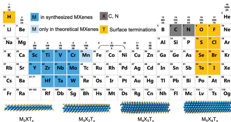
**FIGURE 1.1** Periodic table showing elements used to build MXene. The schematics of four typical structures of MXene are shown at the bottom.
