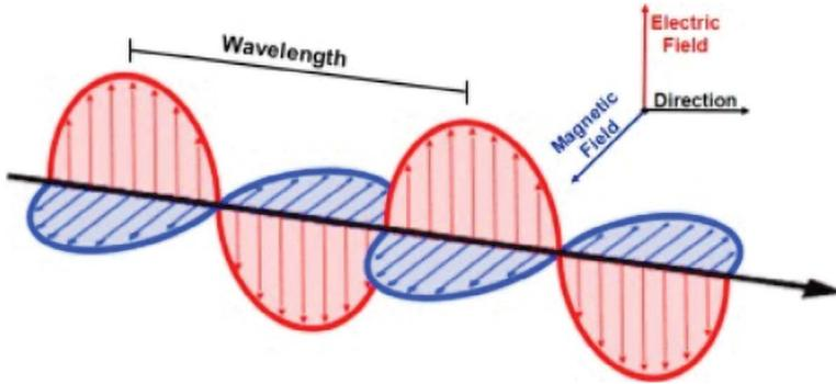
**FIGURE 9.10** Schematic representation of EM wave.
