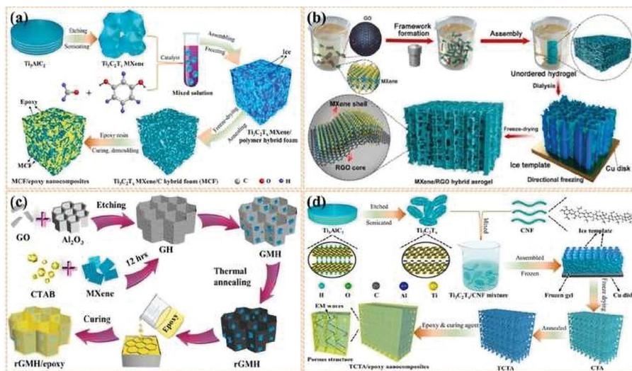
**FIGURE 9.5** (a) The fabrication for the MCF/epoxy EMI composites. (Ref. 55, © 2019, Elsevier.) (b) Schematic diagram showing the preparation of  $Ti_3C_2T_x$ /RGO hybrid aerogels. (Ref. 54, © 2018, American Chemical Society.) (c) Fabrication of rGMH/epoxy nanocomposites. (Ref. 56, © 2020, Elsevier.) (d) The fabrication of MXene/CNF/epoxy nanocomposites [57].
