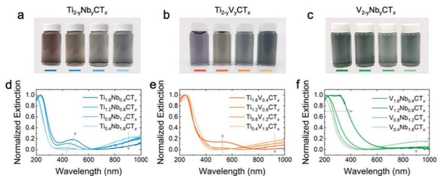
**FIGURE 4.7** (a, b, and c) Digital photograph of  $(\text{Ti}_{2-y}\text{Nb}_y)\text{C}$ ,  $(\text{Ti}_{2-y}\text{V}_y)\text{C}$ , and  $(\text{V}_{2-y}\text{Nb}_y)\text{C}$  MXenes colloidal solution in deionized water shows a change in color with a change in compositions. (d, e, and f) show the UV-vis spectrum of the corresponding MXenes normalized to a maximum excitation of 1. It reveals multiple types of features with a nonlinear change from UV to NIR with a change in composition.
