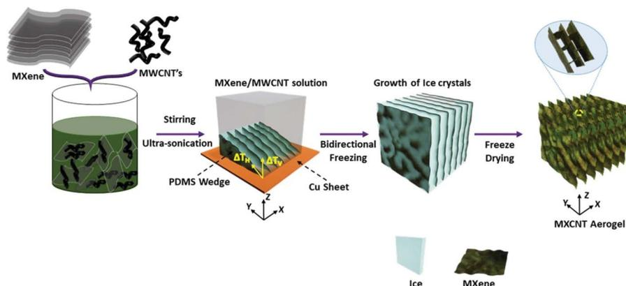
**FIGURE 8.10** Bidirectional freezing method for  $\text{Ti}_3\text{C}_2\text{T}_x/\text{CNT}$  hybrid aerogel fabrication.
