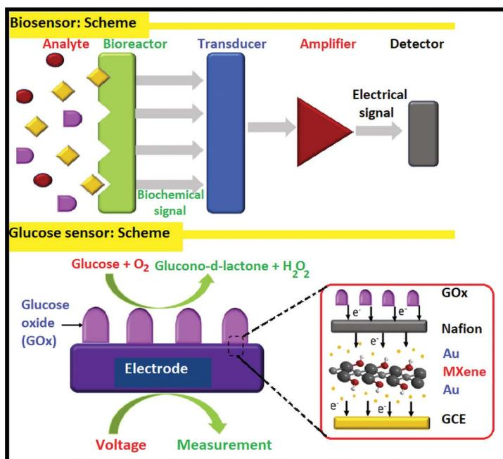
**FIGURE 10.2** Schematic representation of the working of a biosensor and glucose biosensor.
