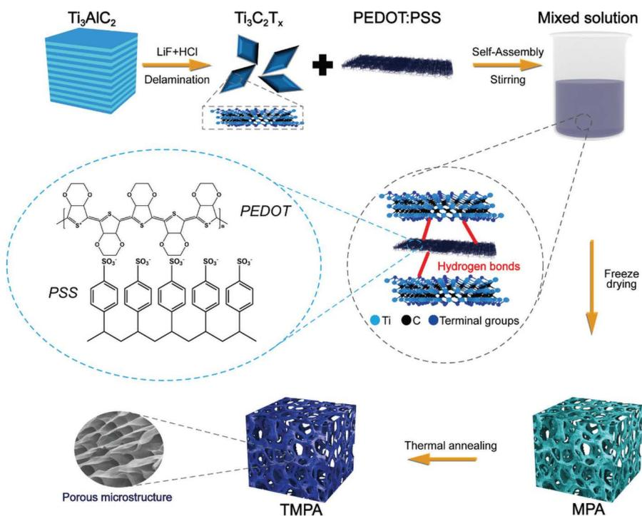
**FIGURE 8.11** The diagram illustrates the preparation of  $\text{Ti}_3\text{C}_2\text{T}_x/\text{PEDOT:PSS}$  hybrid aerogel (MPA) and thermally treated MPA (TMPA).
