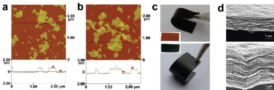
**FIGURE 6.1** Characterisation images of GO and rGO nanosheets and paper. AFM images of (a) GO and (b) rGO layers; (c) images of flexible and freestanding GO and rGO paper (top and bottom respectively); (d) SEM measurements of thickness of GO and rGO.
