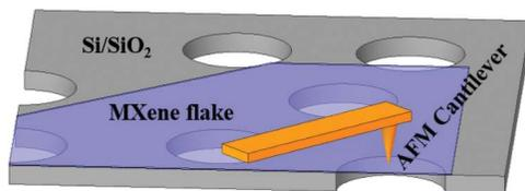
**FIGURE 4.9** A schematic of nanoindentation technique using AFM cantilever tip to calculate Young's modulus and fracture strength. A monolayer of MXene flake is deposited on a pre-micro holes Si/SiO<sub>2</sub> substrate and a force-indentation experiment is carried out for mechanical properties analysis.
