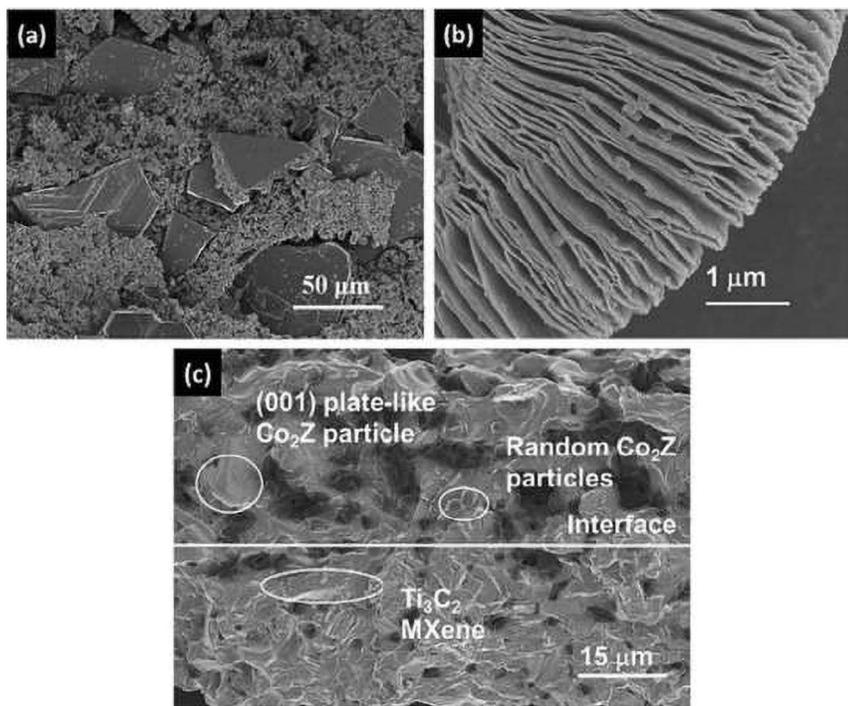
**FIGURE 9.8** SEM images of (a)  $\text{Co}_2\text{Z}$  powder, (b)  $\text{Co}_2\text{Z}$  plate-like oriented powder blend  $\text{Ti}_3\text{C}_2$  MXene; and (c) synthesized PVB/ $\text{Co}_2\text{Z}$ / $\text{Ti}_3\text{C}_2$  composite.
