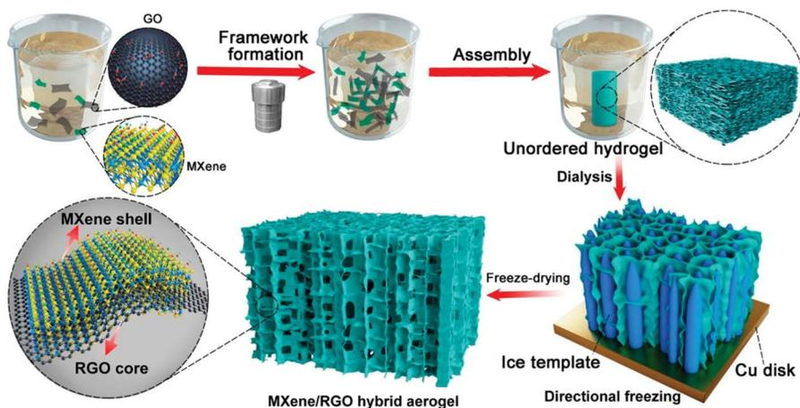
**FIGURE 8.6** GO-assisted hydrothermal assemblies, directional freezing, and freeze-drying of a  $\text{Ti}_3\text{C}_2\text{T}_x$  MXene/RGO hybrid aerogel.
