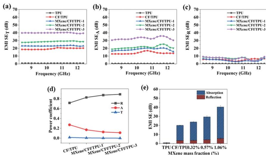
**FIGURE 11.4** (a) Total EMI SE ( $SE_T$ ) of the composites within the frequency range of X-band; (b) EMI SE ( $SE_A$ ) values of the composites within the frequency range of X-band; (c) EMI SE ( $SE_R$ ) values of the composites within the frequency range of X-band; (d) power coefficient values of different composites; (e) contribution of absorption/reflection to the total EMI shielding values of the composites with increase in MXene wt%.
