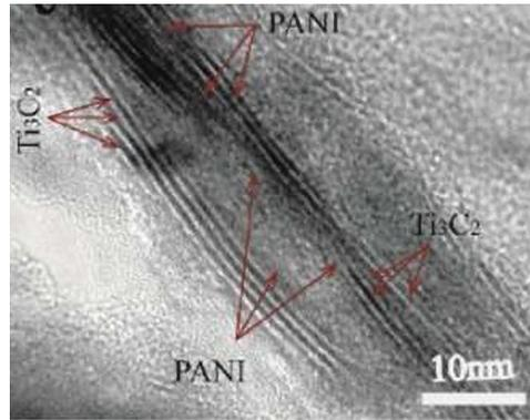
**FIGURE 9.9**  $\text{Ti}_3\text{C}_2\text{T}_x$  MXene/PANI composites TEM image.
