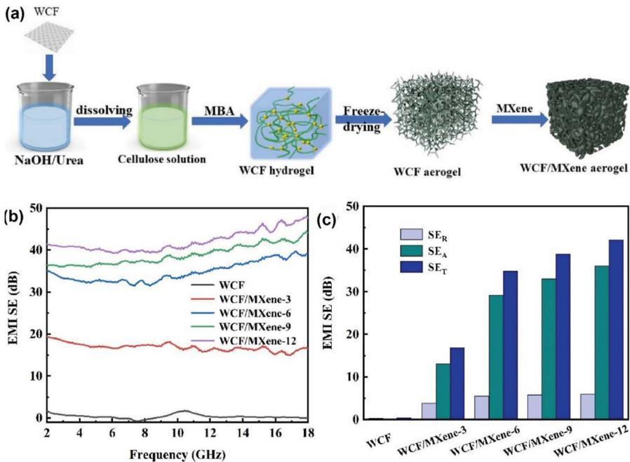
**FIGURE 12.10** (a) Schematic illustration of the fabrication of WCF/MXene composite aerogels through facile freezing-drying and dip-coating method; (b) EMI SE of WCF and WCF/MXene aerogels in the frequency limit of 2–18 GHz; (c) average value of SE<sub>A</sub>, SE<sub>R</sub>, and SE<sub>T</sub> of WCF and WCF/MXene aerogels.
