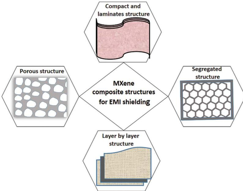
**FIGURE 12.4** Schematic diagram of different types of MXene composite structures applicable in EMI shielding.
