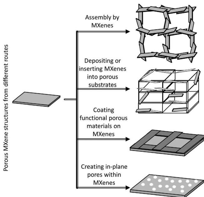
**FIGURE 8.2** Various fabrication approaches for preparing porous MXenes.
