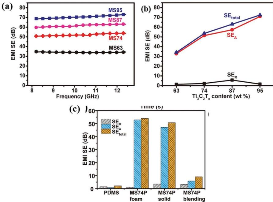
**FIGURE 11.6** (a) Total EMI shielding efficiency of the MXene-SA based aerogels; (b) change in the values of  $SE_{total}$ ,  $SE_A$ ,  $SE_R$  of the MXene-SA based aerogels with the MXene content; (c) total EMI SE of PDMS, MS74P foam, MS74P solid and MS74P blending.
