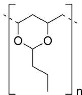
**FIGURE 9.7** Structure of polyvinyl butyral (PVB). It is a clear, colorless, amorphous thermoplastic resin with the general formula  $(\text{C}_8\text{H}_{14}\text{O}_2)_n$ .
