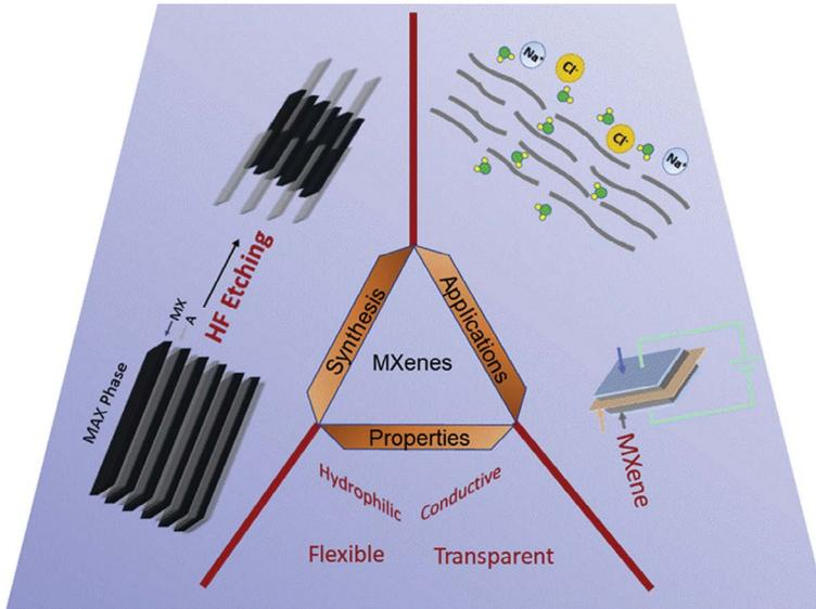
**FIGURE 9.2** The different stages involved in fabrication of MXenes from its precursor MAX phase, which also includes the properties and various applications of MXene.
