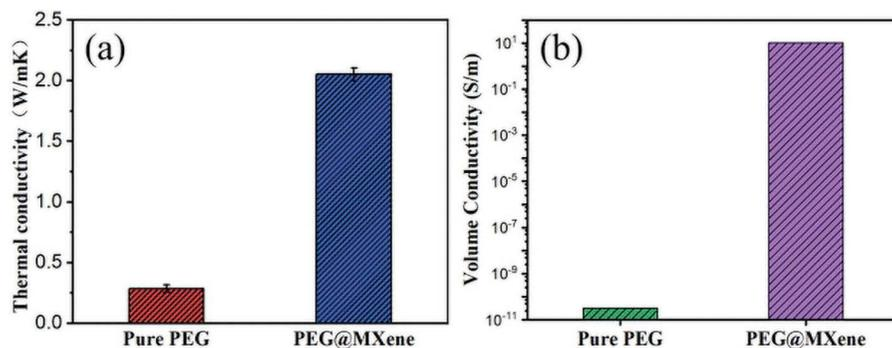
**FIGURE 6.10** Bar graphs demonstrating thermal conductivity and volume conductivity of pristine PEG and PEG@MXene.
