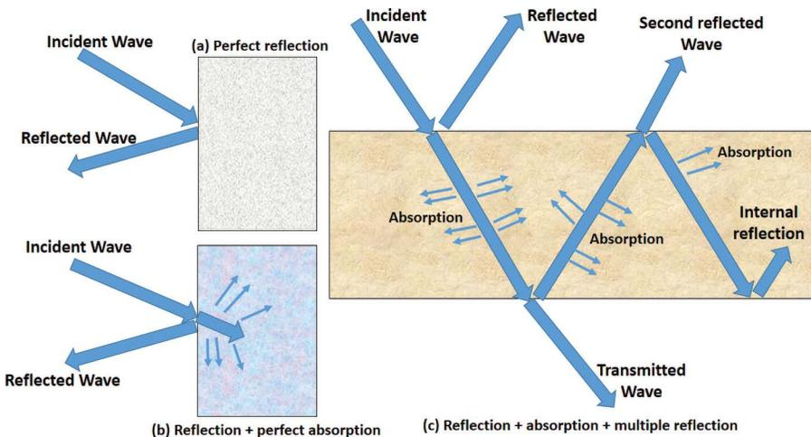
**FIGURE 12.2** Mechanism of EMI shielding from compact and/or laminated structures when interacting with EM waves: (a) perfect reflection, (b) reflection + perfect absorption, (c) reflection + absorption + multiple reflection.
