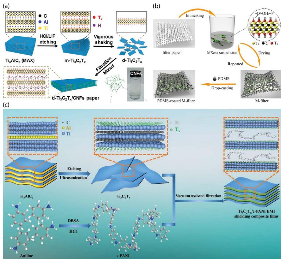
**FIGURE 9.6** (a) Represents the fabrication of the  $d\text{-Ti}_3\text{C}_2\text{T}_x/\text{CNF}$  composite papers prepared by the self-assembly by the filtration which vacuum assisted. (Ref. 58, © 2018, American Chemical Society.) (b) Illustration of the preparation of freestanding nanocomposites process. (c) Synthesis of  $\text{Ti}_3\text{C}_2\text{T}_x/\text{PANI}$  composite films. (Ref. 66, © 2019, Elsevier.)
