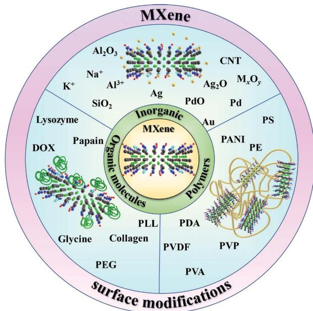
**FIGURE 3.1** A schematic presenting a plethora of possibilities to modify MXenes for EMI shielding applications.
