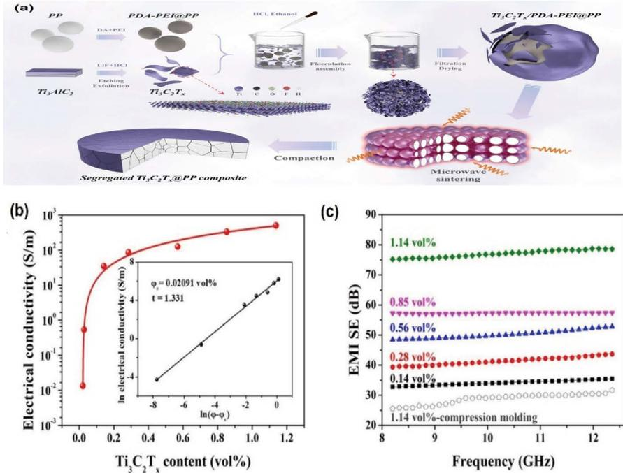
**FIGURE 12.12** (a) Schematic diagram of the fabrication of the segregated  $Ti_3C_2T_x@PP$  composite through the self-assembly and microwave selective sintering route; (b) electrical conductivity versus  $Ti_3C_2T_x$  content for the segregated  $Ti_3C_2T_x/PDA-PEI@PP$  composites (inset shows  $\ln$  conductivity versus  $\ln(\phi-\phi_c)$  line fitted by least square fitting); (c) EMI SE of segregated  $Ti_3C_2T_x/PDA-PEI@PP$  composites as the function of  $Ti_3C_2T_x$  content.
