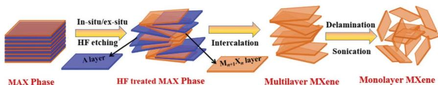
**FIGURE 4.1** A schematic to prepare monolayer MXene from MAX phase by in situ/ex situ HF treatment followed by intercalation and delamination.
