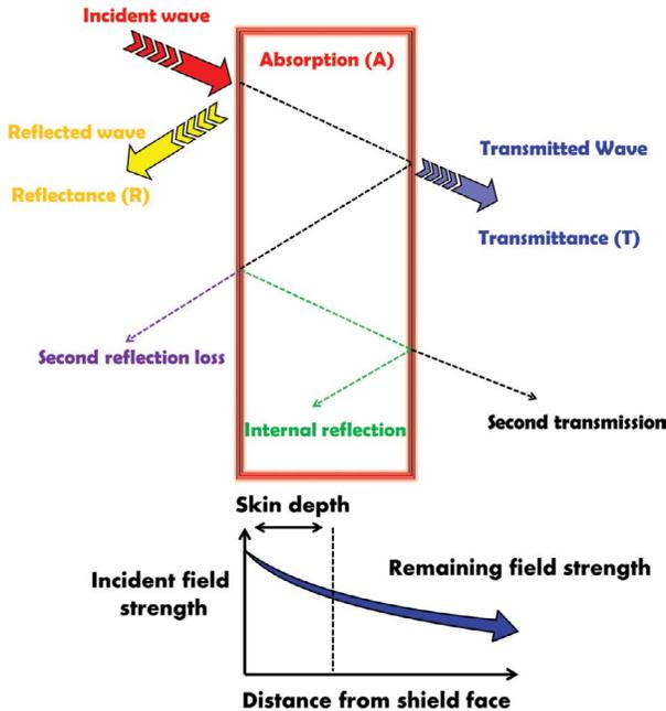
FIGURE 7.1 A schematic depiction of EMI shielding mechanism.
