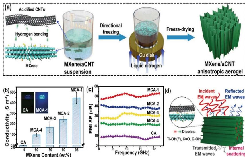
**FIGURE 12.6** (a) Schematic representation of the preparation of the MXene/aCNT aerogel; (b) electrical conductivity vs MXene content for MCAs; (c) plots of EMI shielding effectiveness of MCAs; (d) schematic of EMI shielding mechanisms of MCA.
