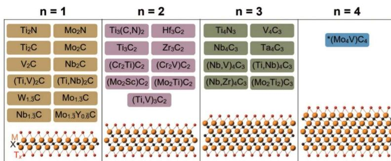
**FIGURE 1.4** MXene compositions reported to date. MXenes discovered to date include mono-M MXenes, ordered double-transition-metal MXenes, solid-solution MXenes and ordered divacancy MXenes.
