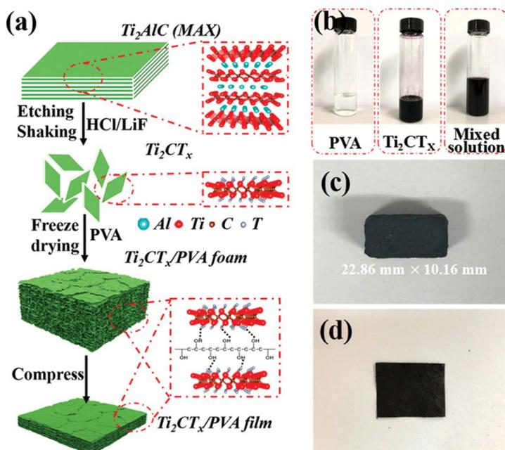
**FIGURE 5.2** (a) Illustration of the preparation process of f-Ti<sub>2</sub>CT<sub>x</sub>/PVA composite foam and film. (b) Bottle of PVA solution that is nearly transparent, bottle of f-Ti<sub>2</sub>CT<sub>x</sub> solution with pure black color, and bottle of f-Ti<sub>2</sub>CT<sub>x</sub>/PVA solution. (c) Photograph of f-Ti<sub>2</sub>CT<sub>x</sub>/PVA foam. (d) Typical photograph of f-Ti<sub>2</sub>CT<sub>x</sub>/PVA film.
