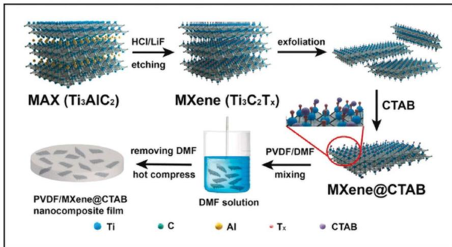
**FIGURE 6.11 (a)** Schematic illustration depicting preparation process of PVDF/MXene@CTAB NC films.
