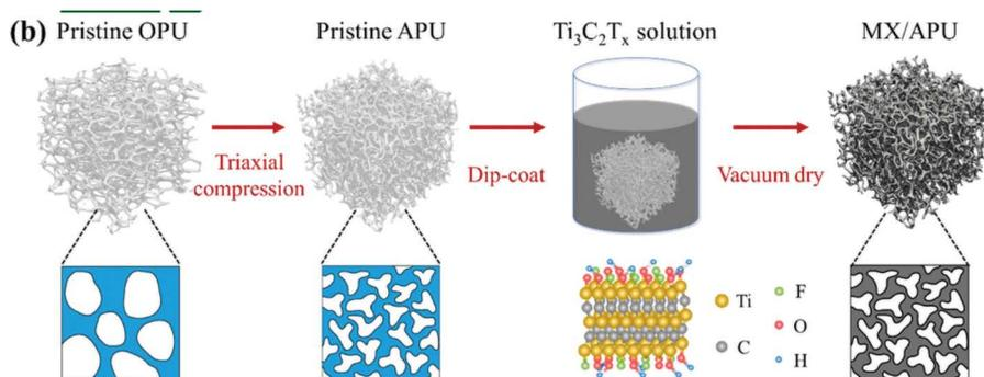
**FIGURE 11.1** Schematic representation of fabrication of MX/APU foam composite.
