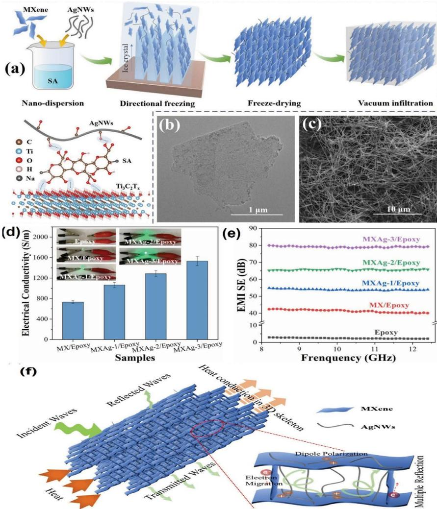
**FIGURE 12.11** (a) Schematic illustration of the fabrication of MXene/AgNWs/epoxy composites; (b) TEM image of  $Ti_3C_2T_x$  MXene; (c) SEM image of AgNWs; (d) electrical conductivity of MXene/AgNWs/epoxy composites; (e) EMI SE of MXene/AgNWs/epoxy composites with a thickness of 2 mm; (f) schematic illustration of possible mechanism EMI shielding and heat conduction in MXene/AgNWs/epoxy nanocomposites.
