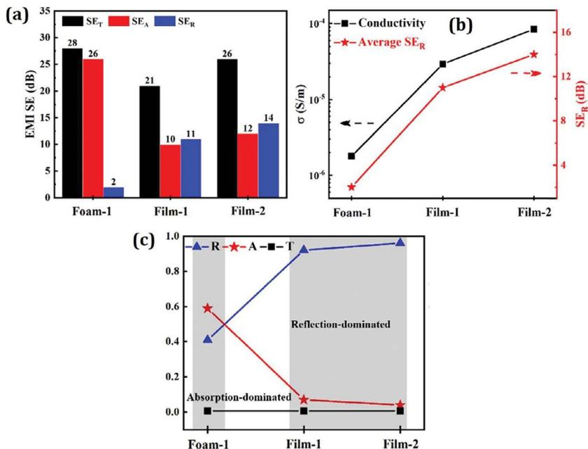
**FIGURE 8.9** (a) EMI shielding values of f-Ti<sub>2</sub>CT<sub>x</sub>/PVA foam; (b) conductivity and shielding comparison of f-Ti<sub>2</sub>CT<sub>x</sub>/PVA foam; (c) composite f-Ti<sub>2</sub>CT<sub>x</sub>/PVA reflectance (R), absorption (A), and transmission (T).
