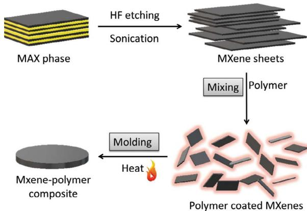
**FIGURE 5.1** Schematic illustration of MXene-based physical mixing method for composite preparation.
