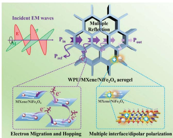
**FIGURE 8.7** Schematic illustration of waterborne PU aerogel fabrication for EMI shielding applications.
