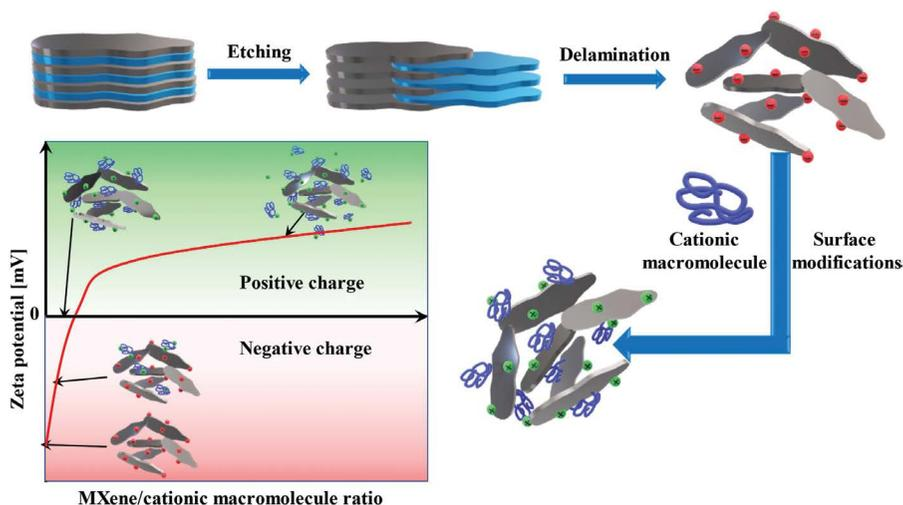
**FIGURE 3.3** Schematic image presenting the synthesis and surface modification of MXenes with cationic molecules into MXene/molecule hybrids, as well as in-operando tracking approach, developed for the adsorption of macromolecules on MXene's surface.
