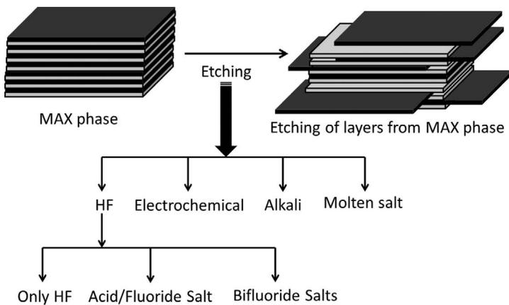
**FIGURE 2.2** Classifications of different types of etching methods for preparing the MXenes.
