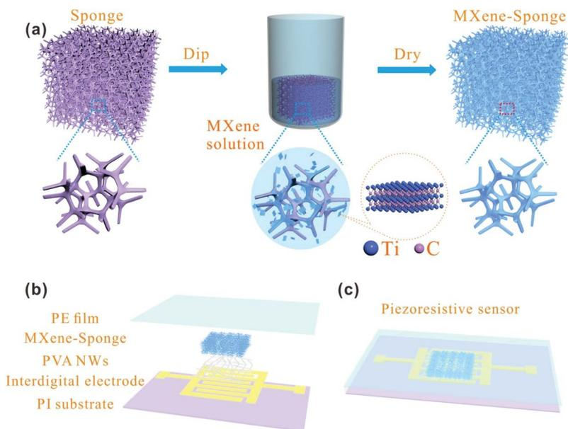
**FIGURE 8.4** (a) Schematic depiction of the MXene-sponge manufacturing process; (b, c) schematic representation of the construction of a sensor based on MXene-Sponge/PVA NWs.
