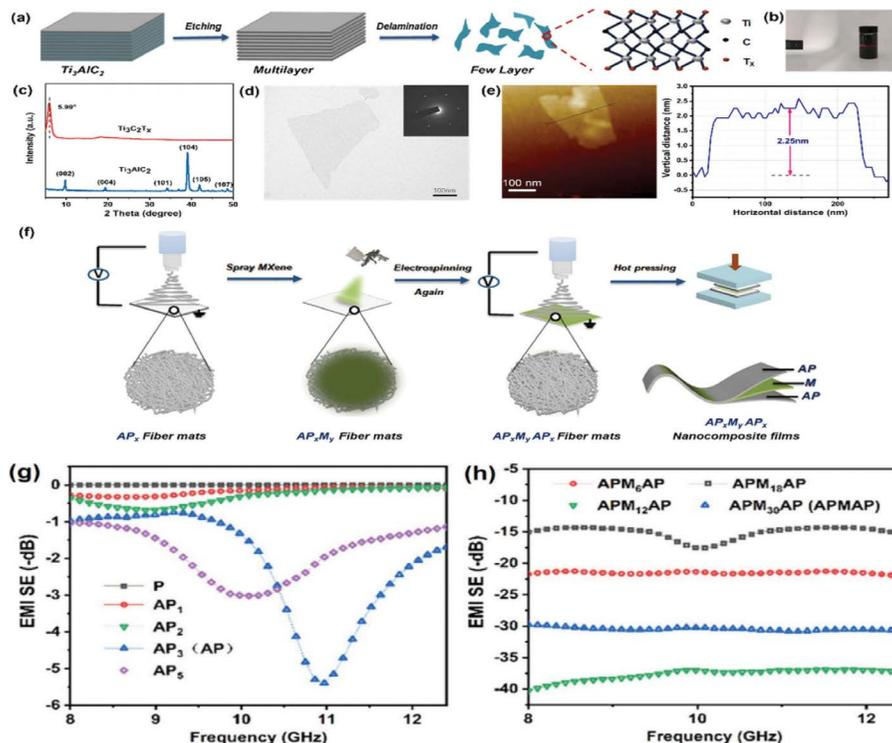
**FIGURE 12.7** (a) Preparation of few-layered  $Ti_3C_2T_x$  nanosheets by wet chemical etching method; (b) the Tyndall effect was observed in  $Ti_3C_2T_x$  MXene solution under laser pointer irradiation; (c) XRD patterns of  $Ti_3AlC_2$  and  $Ti_3C_2T_x$ ; (d) TEM images of  $Ti_3C_2T_x$ ; (e) AFM images and the thickness of  $Ti_3C_2T_x$ ; (g) EMI SE of the AP film with different AgNW contents; (h) EMI SE of  $APM_xAP$  at different MXene loadings.
