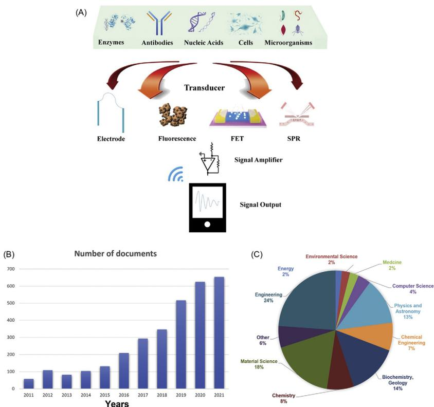
**FIG. 3.1** (A) Typical biosensor is generally defined as an analytical system which schematically consists of a biorecognition element, a transducer element, a signal transmission and amplifier element.<sup>16</sup> Reprinted with permission from Elsevier. (B) The analysis of Scopus search results related to the wearable biosensors from 2011 to September 2021. (C) The subject areas of wearable biosensors during the same period.
