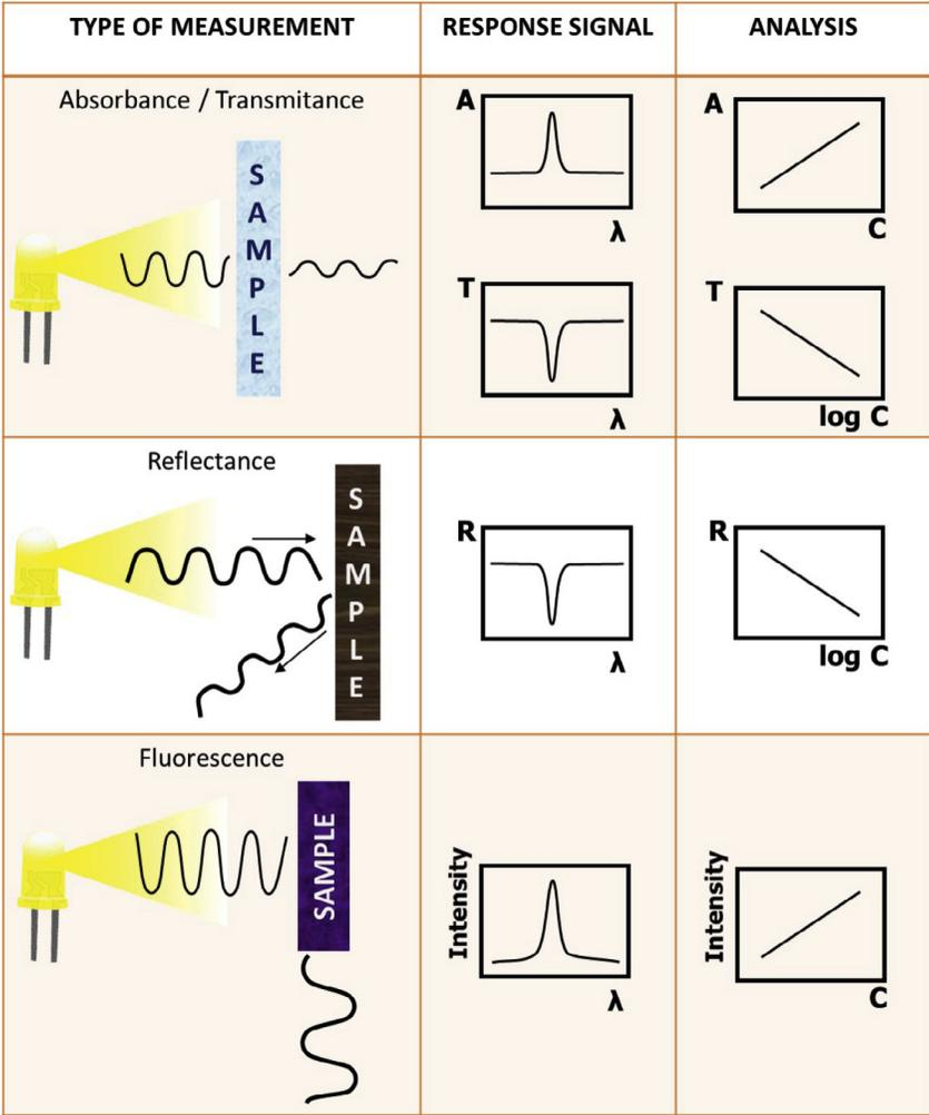
**FIG. 4.1** Scheme of the excitation signal, response signal and analysis response for the main optical detection techniques in wearable devices (adapted from 18).
