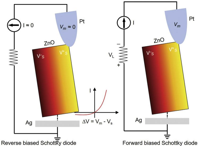
**FIG. 7.4 Working principle of PENG.** The AFM conductive tip comes into contact with the semiconductor ZnO NW at two reversed local contact potentials. The inset shows the Schottky rectifying behavior of the reverse- and forward-biased Schottky diode.<sup>32</sup>
