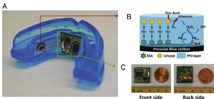
**FIG. 3.4** (A) Photograph of the mouthguard biosensor integrated with wireless amperometric circuit board. (B) Reagent layer of the chemically modified printed Prussian-blue carbon working electrode containing uricase for UA biosensor. (C) Image of the wireless amperometric circuit board: front side (left) and back side (right).<sup>125</sup> Reprinted with permission from Elsevier.
