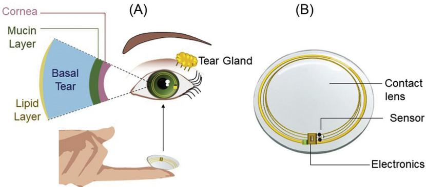
**FIG. 8.5 Contact lens as a tear-based wearable platform.** (A) Contact lens measures tear analytes from the basal tear, permanent fluid present in the eye. (B) The chemosensor and electronics can be enclosed inside the contact lens structure. The signal can be acquired electrochemically and sent via the wireless system, or optically via a smartphone application-based image analysis.
