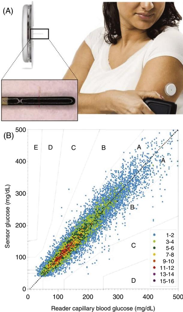
**FIG. 9.4** (A) Photo of the Abbott FreeStyle Libre Flash Glucose Monitoring System. *Adapted with permission from reference,<sup>3</sup> Copyright 2019, Springer Nature.* (B) Consensus error grid analysis of data collected using the FreeStyle Libre Flash device with blood glucose readings. *Adapted with permission from reference,<sup>15</sup> Copyright 2015, Mary Ann Liebert, Inc.*
