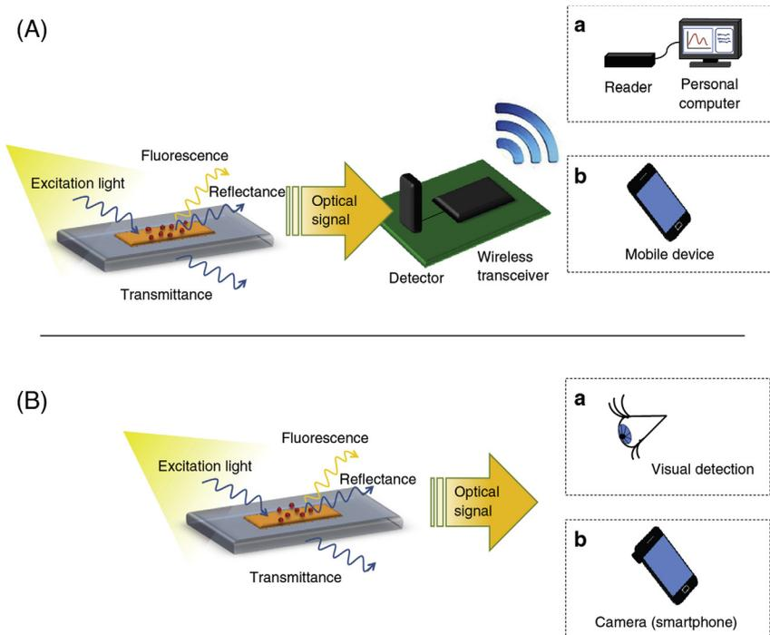
**FIG. 4.2** (A) Schematics of a wireless optical (bio)chemical sensor, sending data to a personal computer (a) or a mobile device (b). (B) Optical sensor with wireless visual readout (a) or using remote camera (b), without radio communication. *Reprinted from 19, 2018 Walter de Gruyter GmbH.*
