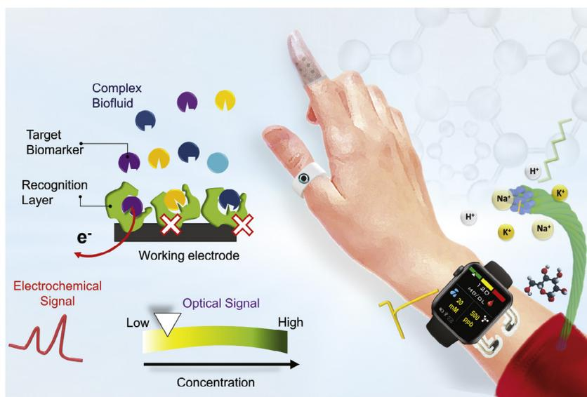
**FIG. 8.1** Wearable chemosensors used to continuously monitor the body's real-time chemical information. An electrochemical transducer (working electrode) is modified with a target selective (bio)recognition layer to translate the chemical interaction into a readable electrical signal. A colorimetric or optical transducer relies on the visual color or intensity changes of optically active molecules for qualitative, semi-quantitative or quantitative analysis.
