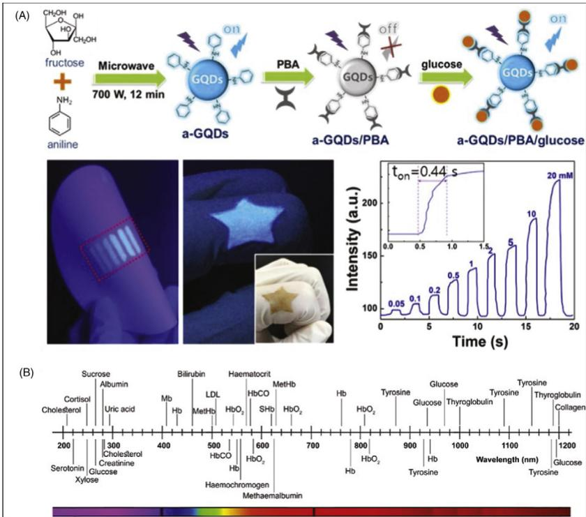
**FIG. 2.4** (A) Synthesis procedure of a-GQDs, its application for glucose detection on a latex glove under daylight and UV-light, and fiber optic-based fluorescence spectra for different glucose concentrations (Reproduced with permission from Tam et al. ©Elsevier, 2021); (B) the absorption peak for important biomarkers (Reproduced with permission from Dhanabalan et al. ©Wiley-VCH GmbH, 2020).
