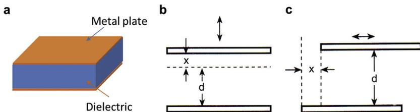
**FIG. 7.6** Working principle of wearable physical sensors based on capacitive effect. (A) Setup and materials of a capacitive sensor. (B) Mechanism of a vertical movement. (C) Mechanism of a lateral movement.
