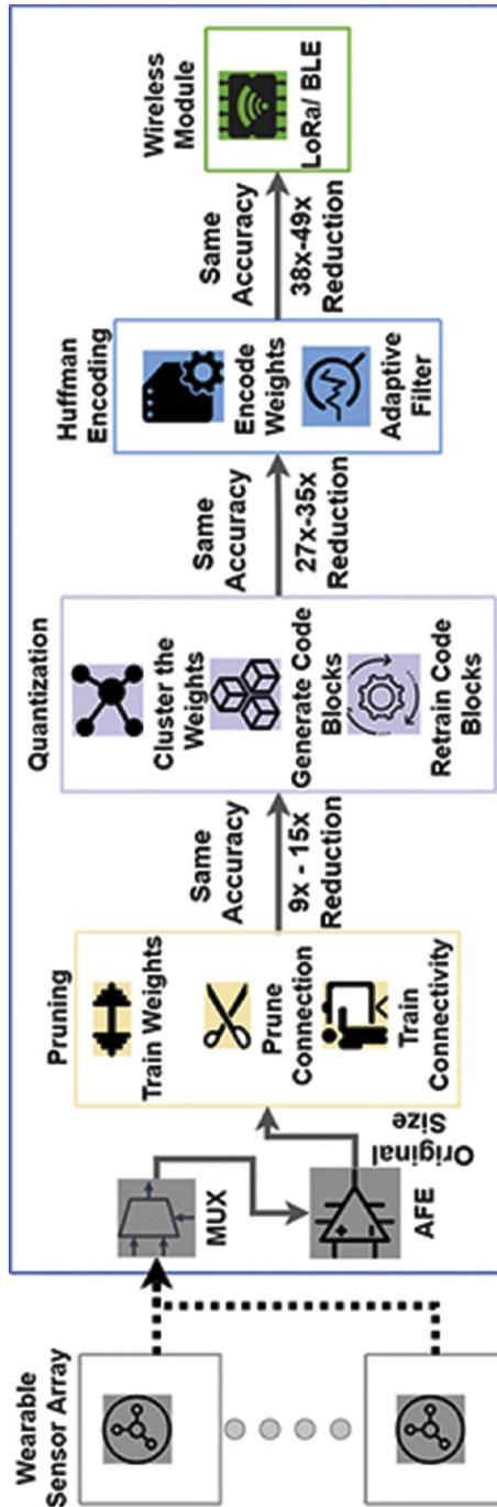
FIG. 6.1 Edge AI-based data compression technique.
