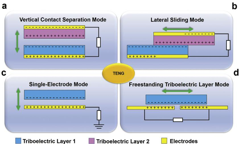
**FIG. 7.2** Four working modes of TENG. (A) Vertical contact separation mode. (B) Lateral sliding mode. (C) Single-electrode mode. (D) Free-standing triboelectric layer mode.
