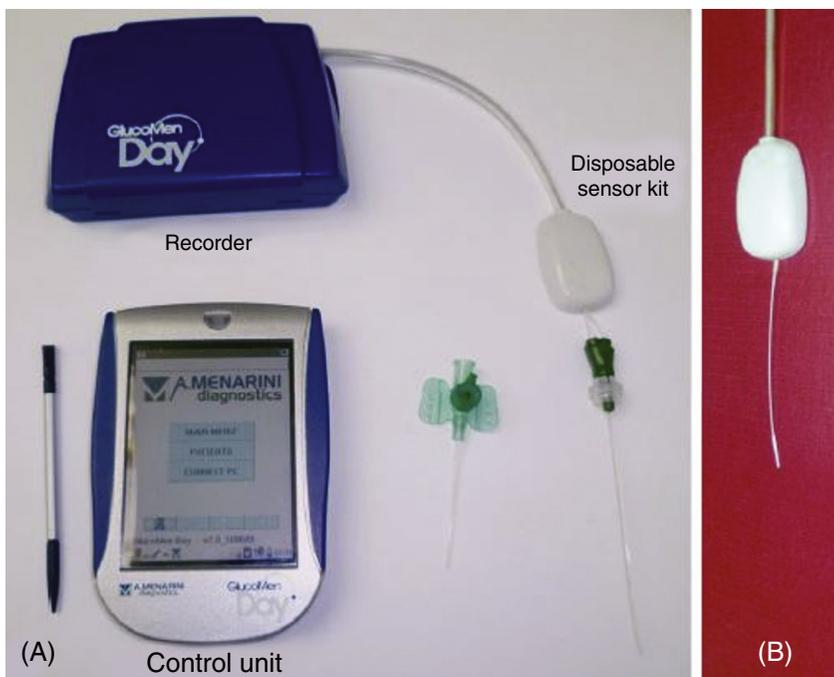
**FIG. 9.7** (A) Device components that make up the GlucoMen Day continuous glucose monitoring system. Adapted with permission from reference,<sup>22</sup> Copyright 2012, SAGE. (B) Disposable sensor kit for interstitial fluid. Adapted with permission from reference,<sup>22</sup> Copyright 2012, SAGE.
