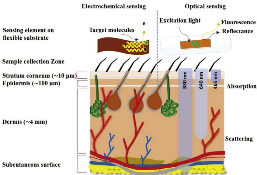
**FIG. 2.1** The basic design and working of wearable biosensors on a soft substrate for health monitoring.
