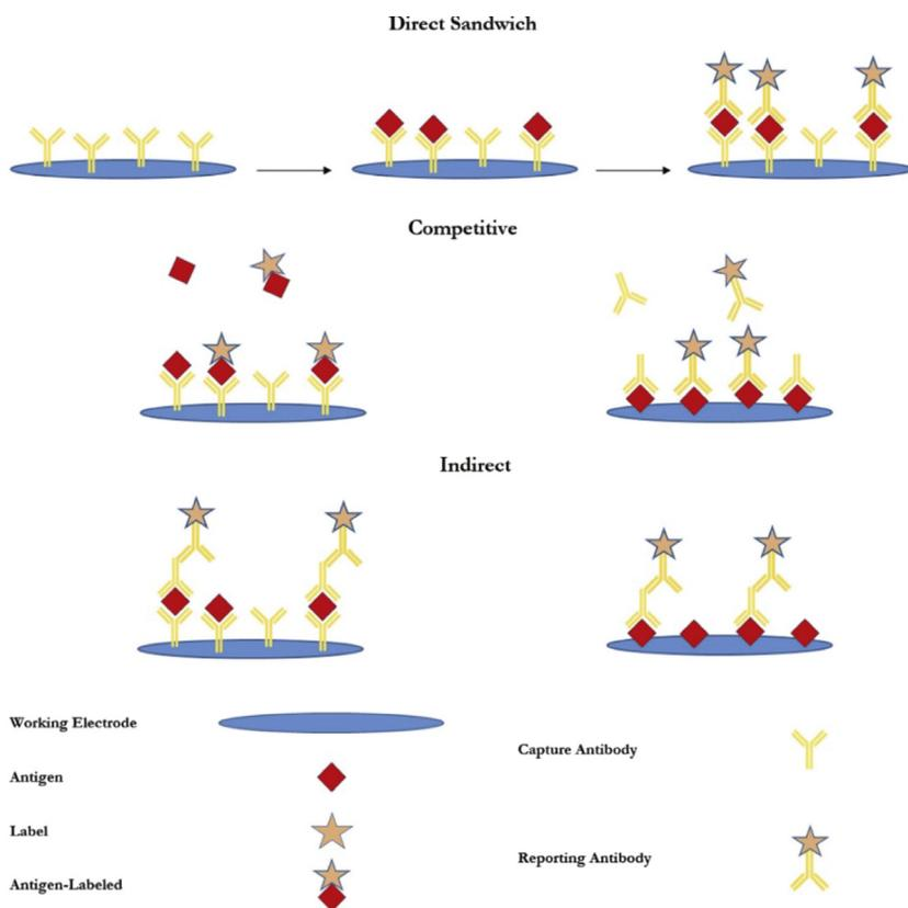
**FIG. 3.2** Schematic illustration of different conventional (direct sandwich, competitive, and indirect) configurations in immunosensors.<sup>23</sup> Reprinted with permission from Elsevier.
