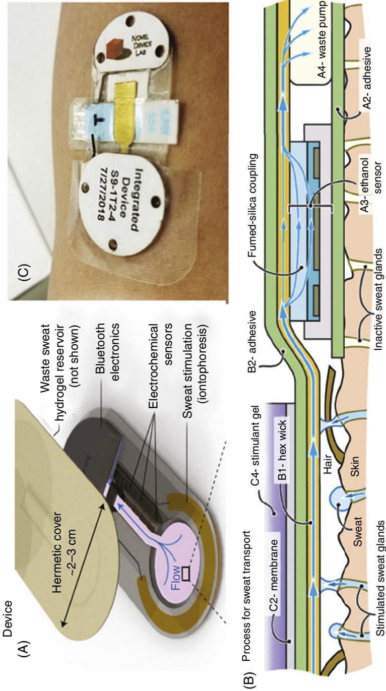
**FIG. 9.2** (A) Diagram of a proposed wearable sweat biosensing device. Adapted with permission from reference.<sup>3</sup> Copyright 2019, Springer Nature. (B) Diagram of the process of sweat transport. Adapted with permission from reference.<sup>10</sup> Copyright 2018, RSC. (C) Photo of an integrated device with all components, except the wireless electronics and battery for *in-vivo* test. Adapted with permission from reference.<sup>10</sup> Copyright 2018, RSC.
