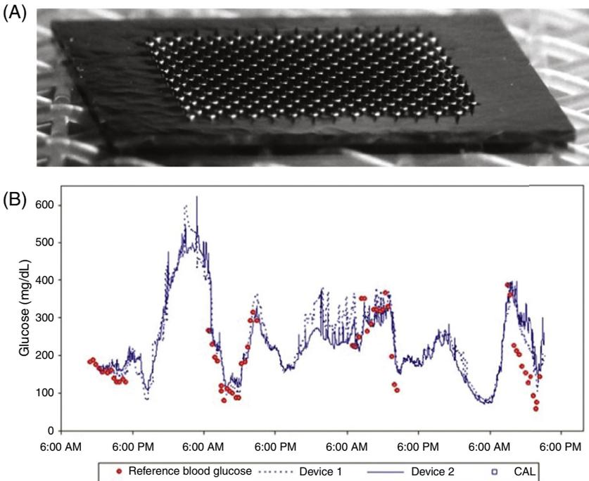
**FIG. 9.6** (A) Photo of ArKal Medical microneedle array. Adapted with permission from reference,<sup>17</sup> Copyright 2014, SAGE. (B) Data generated using the ArKal Medical microneedle array device. This plot displays blood glucose measurements as well as data from two devices which were worn simultaneously by one subject to demonstrate device accuracy and precision. Adapted with permission from reference,<sup>17</sup> Copyright 2014, SAGE.
