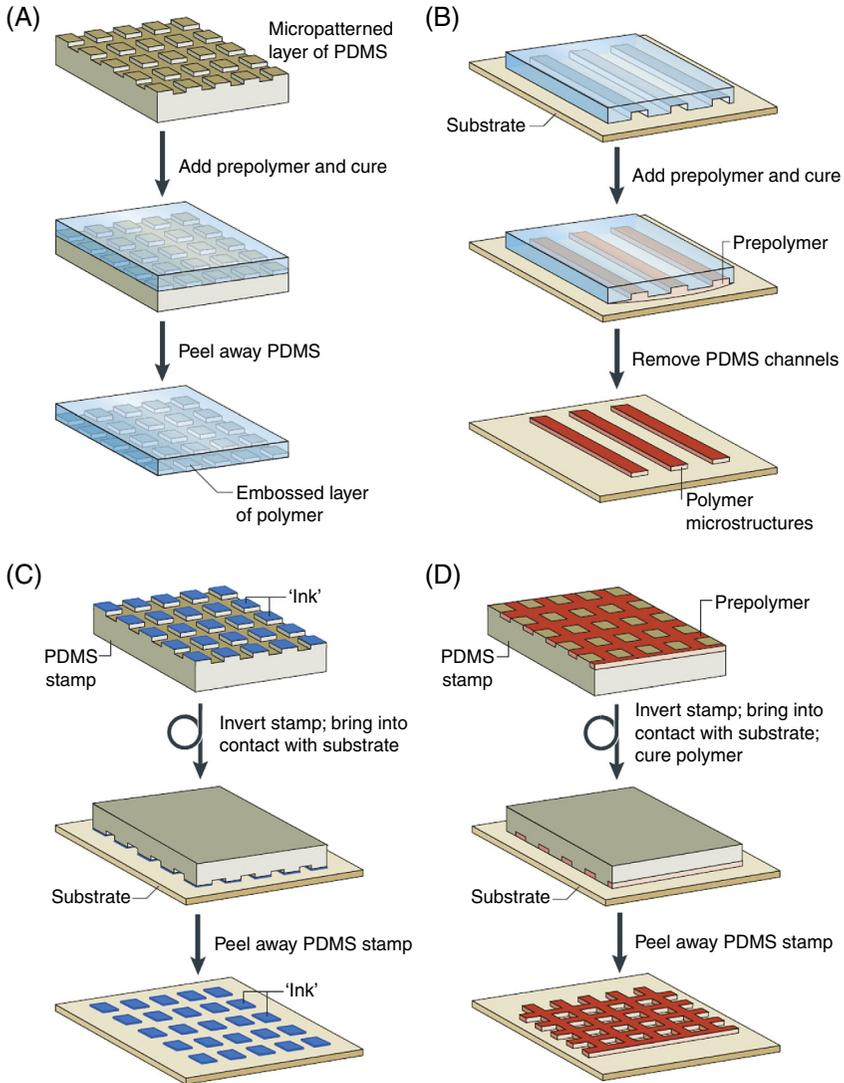
**FIG. 5.1** Key microfluidic patterning techniques used in soft lithography. (A) Replica molding, (B) micromolding in capillaries, (C) microcontact printing, and (D) microtransfer molding (reproduced with permission from ref.<sup>15</sup> copyright 2007, Springer Nature Publishing).
