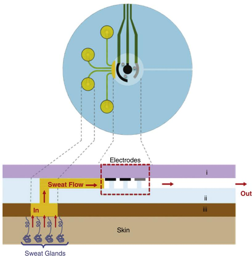
**FIG. 5.2** Cross-sectional schematic of microfluidics in a wearable device (reprinted with permission from ref.<sup>52</sup> copyright 2017, American Chemical Society).
