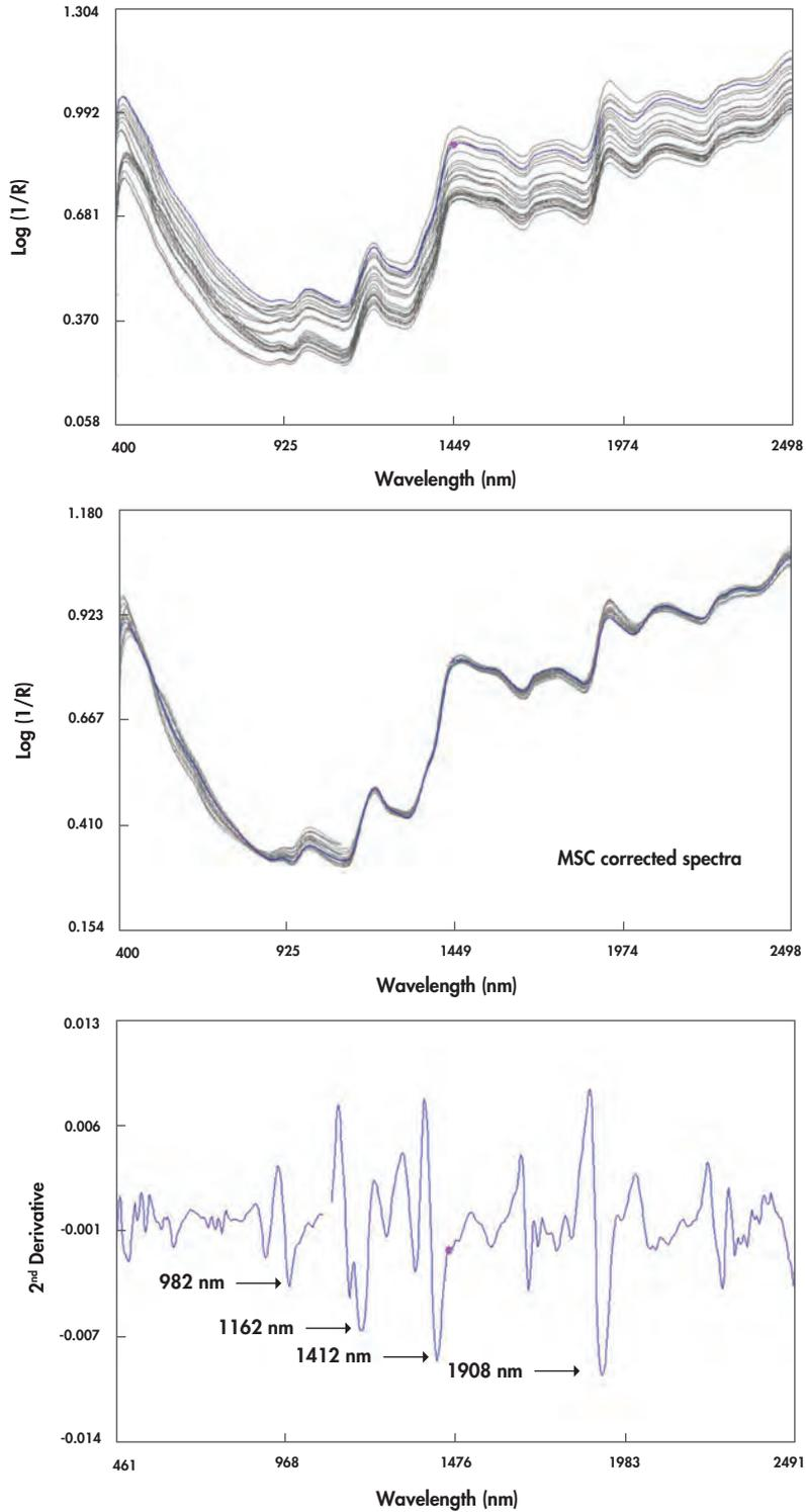
**Figure 5.4** Raw log 1/R spectral of whole wheat of different kernel texture and the effect of applying MSC, SNV and de-trend to the raw spectral data.
