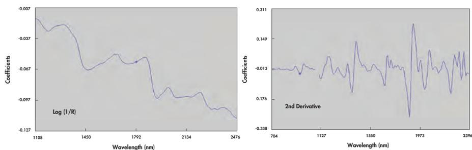
**Figure 10.8** First PLS factor or loadings line plot for prediction of PSI in ground wheat. Calibrations have been developed with log 1/R and 2<sup>nd</sup> derivative (2 4 4 1) spectra.
