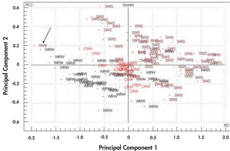
**Figure 10.5** The same PCA scores plot as in Figure 10.4, labelled according to the category variable 'wheat class' (SWS = soft white spring; CRW = Central red spring; WRW = Western red spring). One SWS sample appeared in the same group as WRW.
