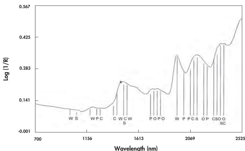
**Figure 10.13** Spectrum of ground oats showing areas where major constituents absorb (C = cellulose or fibre; O = oil; P = protein; S = starch; W = water).
