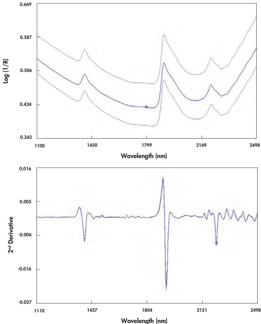
**Figure 11.9** Log 1/R and 2<sup>nd</sup> derivative (2 4 4 1) NIR spectra of three dried soils.
