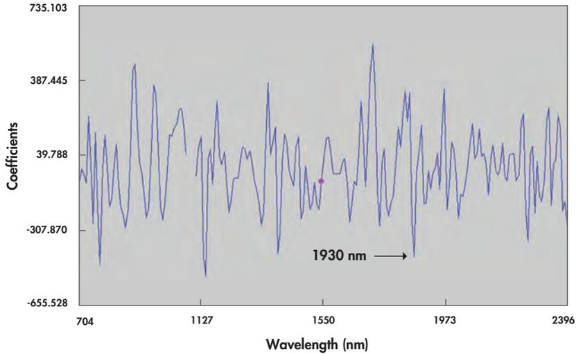
**Figure 10.11** Regression coefficients (b) for prediction of moisture content of whole maize. Calibration has been developed with 2nd derivative (2 4 4 1) spectra. The 'valley' at 1930 nm can be assigned to O-H (water) which absorb at that wavelength.
