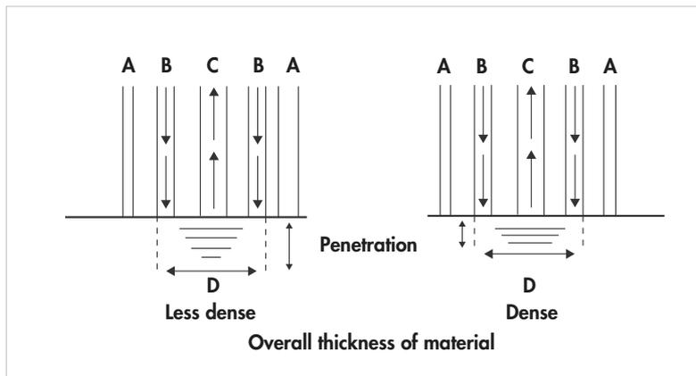
**Figure 6.6** Illustrating the interactance principle. A = outer wall of cable; B = incoming radiation energy; C = diffusely-reflected energy; D = area of material scanned.
