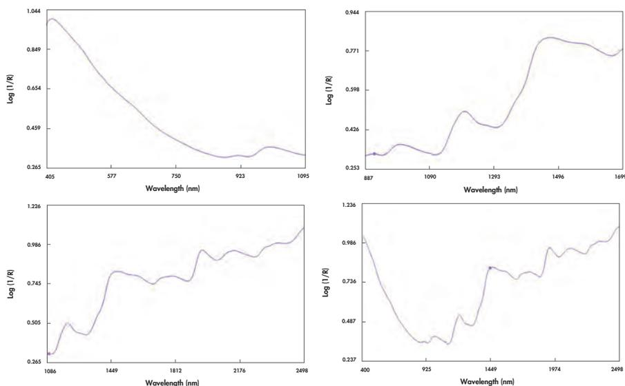
**Figure 9.1** Log 1/R spectra of whole wheat at different wavelength ranges: 400–1100 nm; 900–1700 nm; 1100–2500 nm; and 400–2500 nm.
