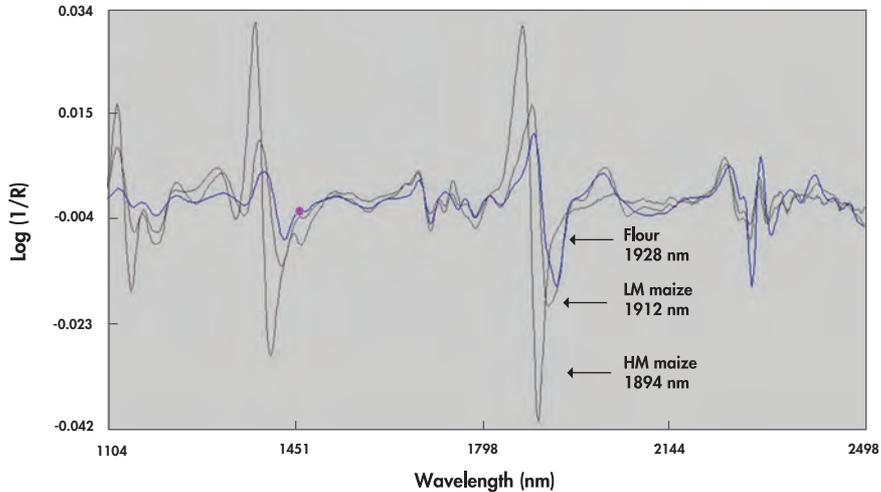
**Figure 2.3** Changes in position of water absorption bands (LM = low moisture; HM = high moisture).
