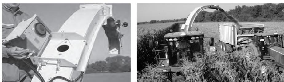
**Figure 11.1** An NIRS instrument on the spout of a forage harvester (left) and in action in the field.
