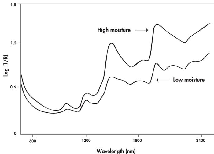
**Figure 8.3** Spectra of high (54%) and low (12%) moisture maize.
