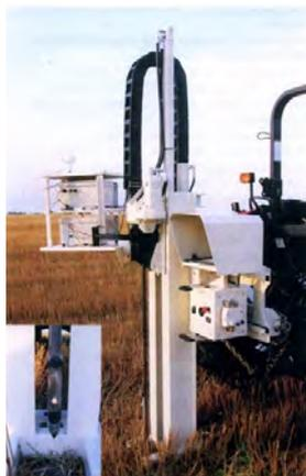
**Figure 11.10** The Veris NIRS soil probe
