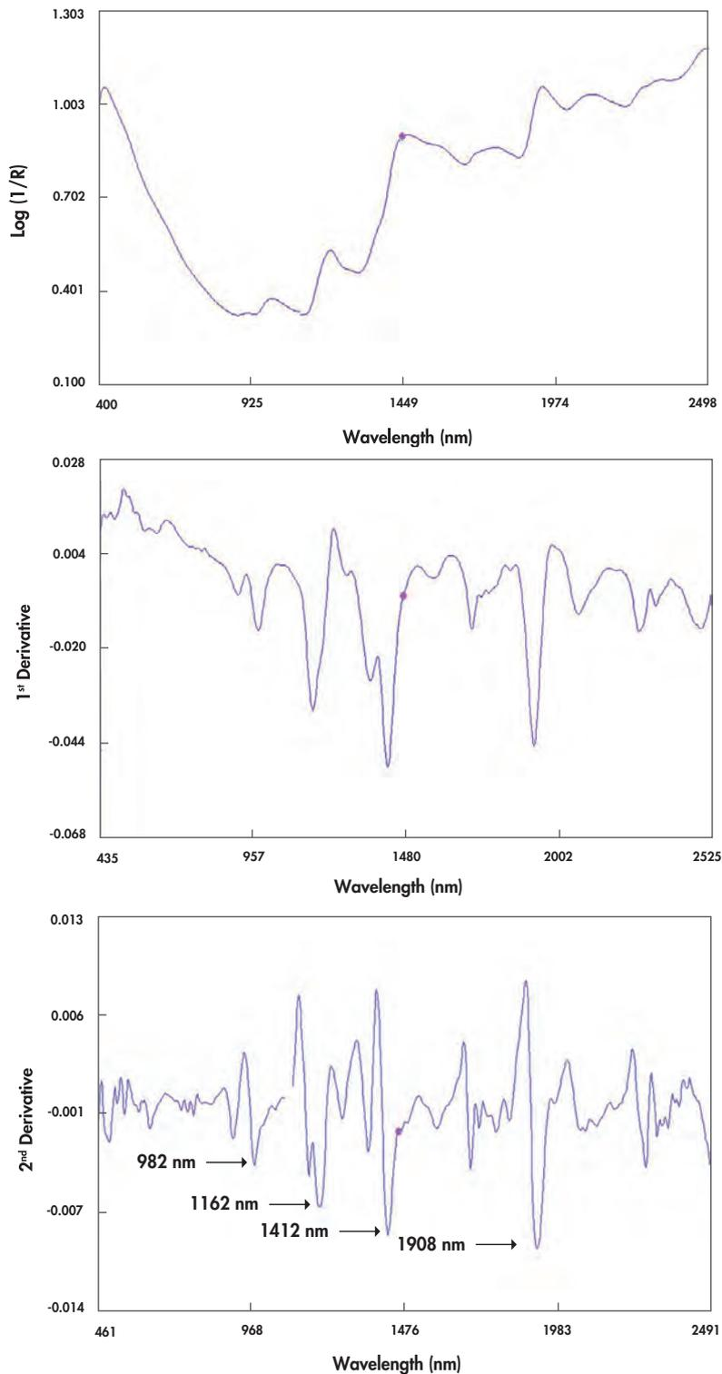
**Figure 5.3** Log 1/R spectrum of whole wheat and the influence of the 1<sup>st</sup> derivative (1 4 4 1) and 2<sup>nd</sup> derivative (2 4 4 1) on the NIR spectrum, with moisture bands indicated.
