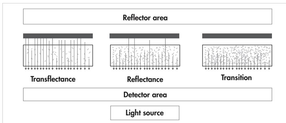
**Figure 7.3** Illustrating transition from transmittance to total reflectance (transition).
