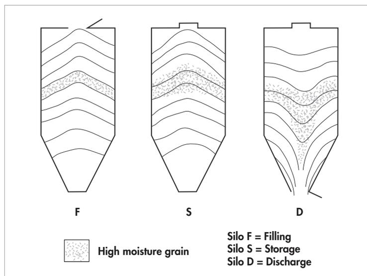
**Figure 7.1** Spread and dispersal of a single delivery of high moisture grain to a silo.
