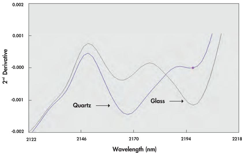
**Figure 6.8** Differences in 2<sup>nd</sup> derivative (2 4 4 1) spectra of glass and quartz.
