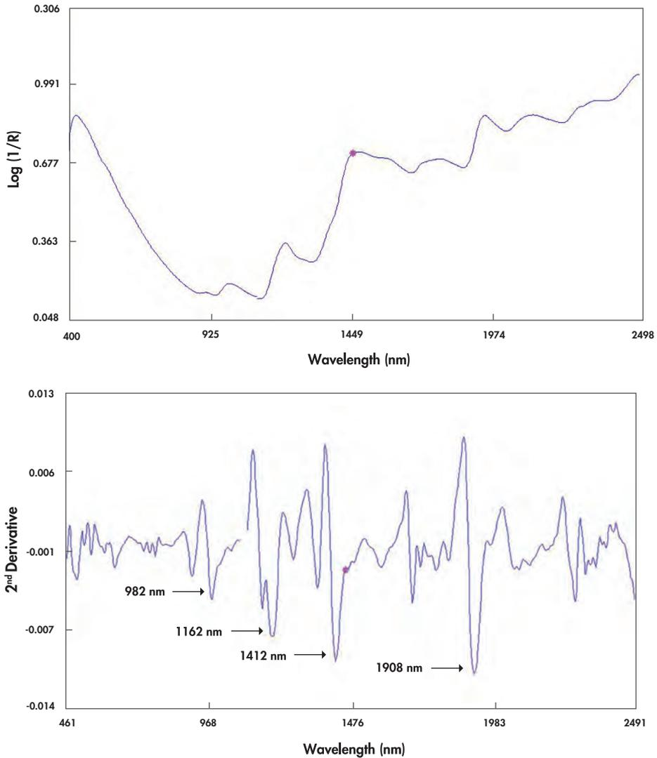
**Figure 1.4** Log 1/R spectrum of whole wheat and the 2<sup>nd</sup> derivative (2 4 4 1) spectrum of the same wheat showing overtones (1412, 1162 and 982 nm) of the moisture band at 1908 nm.
