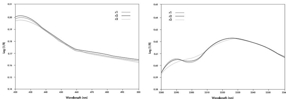
**Figure 5.1** Effect of smoothing between 420–500 nm (left) and 2280–2360 nm on flour spectra. The straightest spectrum in each plot has been smoothed over 10 wavelength points.
