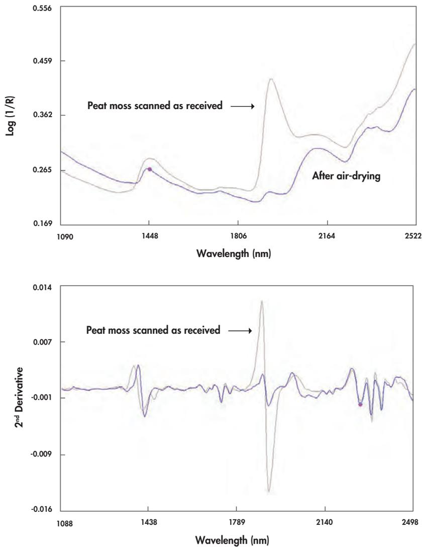
**Figure 11.11** Log 1/R and 2<sup>nd</sup> derivative (2 4 4 1) spectra NIR spectra of peat moss as received and after air-drying.
