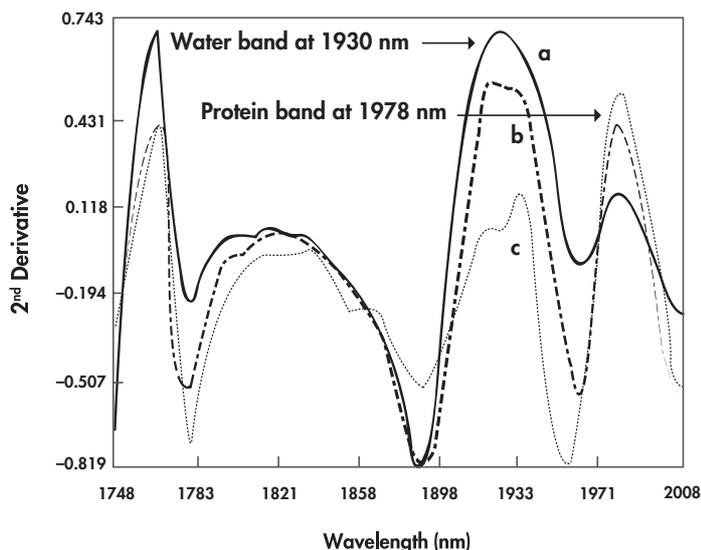
**Figure 8.8** NIRS spectra of soybeans: a) whole as-is; b) after drying and grinding; and c) after grinding and drying.
