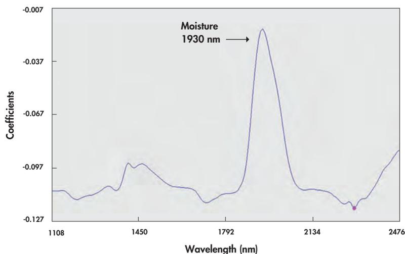
**Figure 10.9** Second PLS factor or loadings line plot for prediction of PSI in ground wheat. Calibration have been developed with log 1/R spectra.
