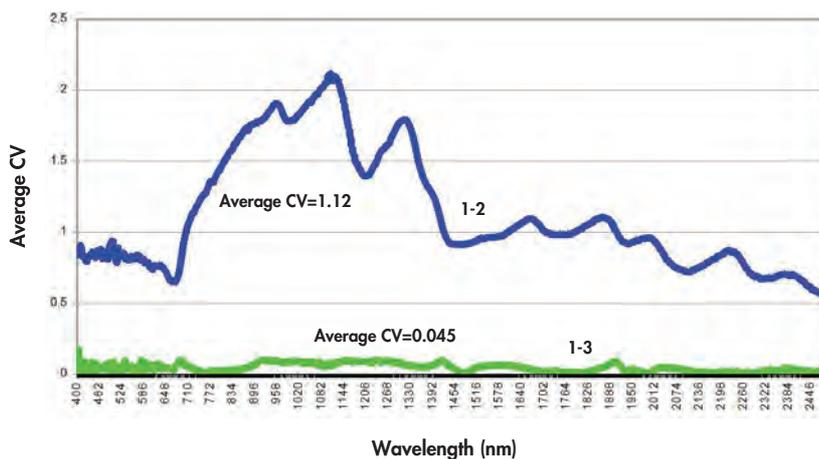
**Figure 11.5** Influence of efficient mixing on the standard deviation (SD) of spectral data of a feed mix. The coefficient of variance (CV) of the dry total mixed ration (TMR) has been used. Upper line = before mixing and the lower line = after mixing.
