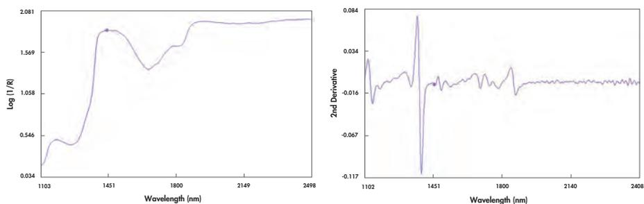
**Figure 8.4** Log 1/R spectrum of fresh chicken breast and the 2<sup>nd</sup> derivative (2 4 4 1) spectrum of the same sample (gap and segment of 4 wavelength points).
