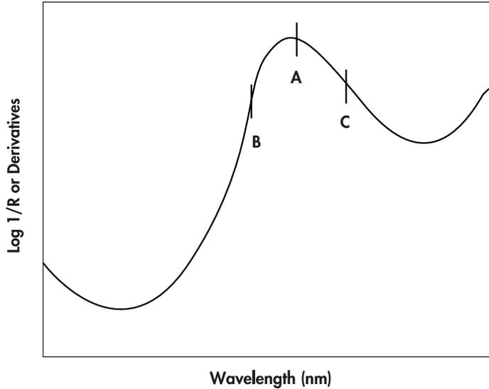
**Figure 5.2** Illustration of the principle of derivatives. Point A is the log 1/R. Points B and C are the wavelength points used in computing the derivatives.
