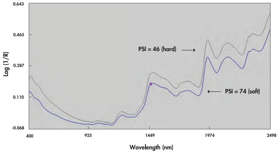
**Figure 1.2** NIR spectra of hard and soft ground wheat (PSI = particle size index).
