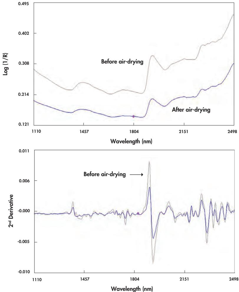
**Figure 11.12** Log 1/R and 2<sup>nd</sup> derivative (2 4 4 1) spectra NIR spectra of beef cattle compost before and after air-drying.
