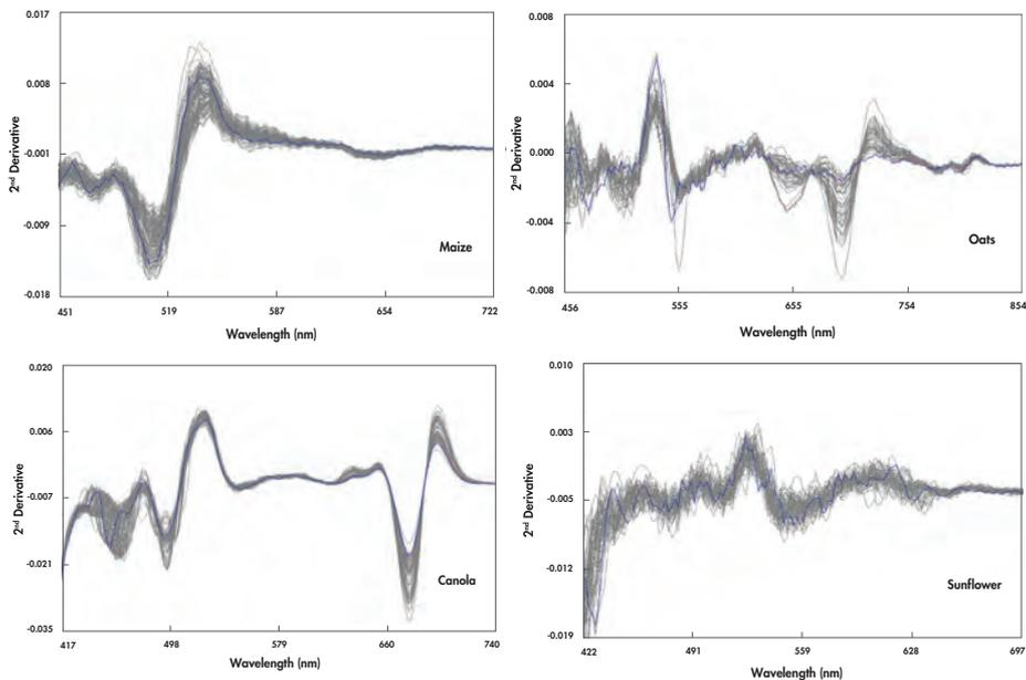
**Figure 6.10** Noise in 2<sup>nd</sup> derivative (2 4 4 1) spectra in the low wavelength range.
