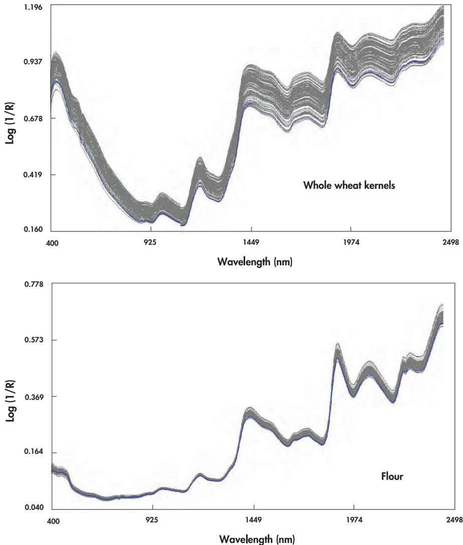
**Figure 2.2** Spectra of hard red spring whole kernels and flour, milled from the same wheat samples.
