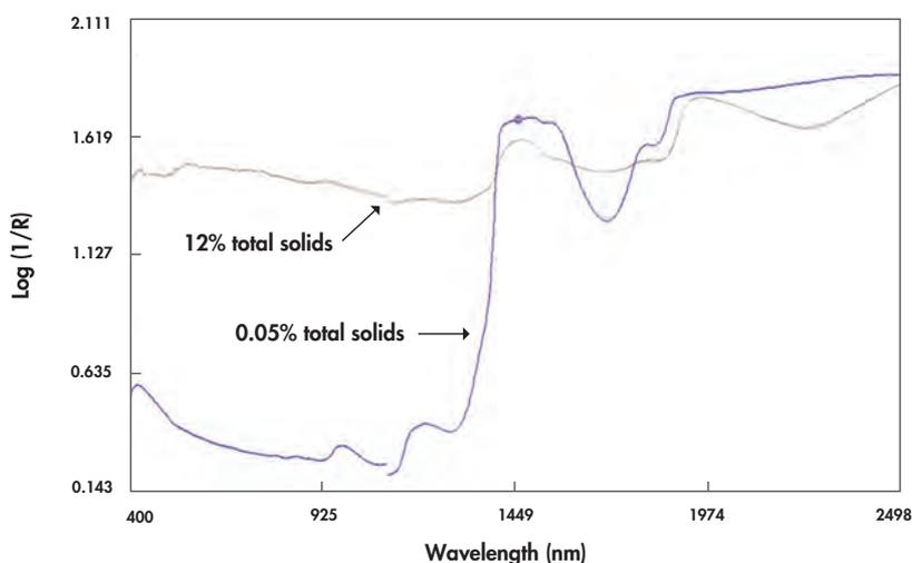
**Figure 8.7** Log 1/R spectra of thin (0.05% total solids) and viscous (12% total solids) liquid hog manure.
