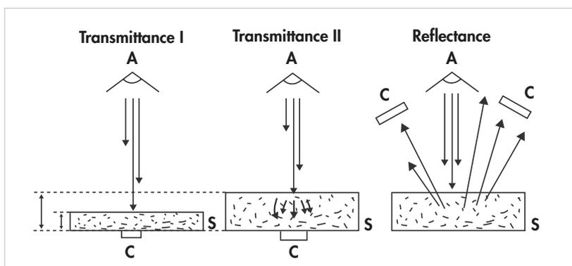
**Figure 6.2** Illustrating differences in sample thickness between transmittance and reflectance instruments. A = light source; C = detector; S = sample.
