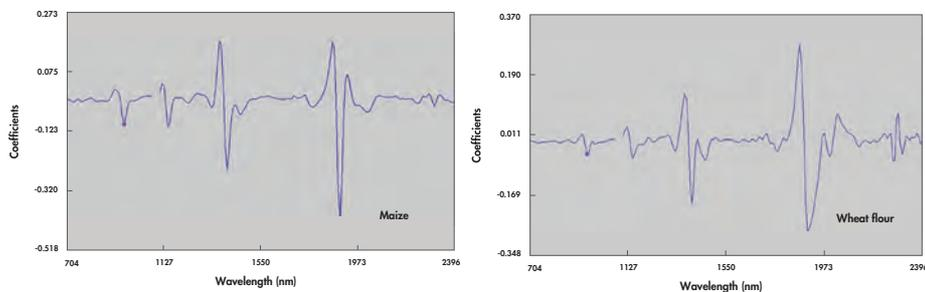
**Figure 10.7** First PLS factors loadings line plots for prediction of moisture in maize and wheat flour. Calibration has been developed with 2<sup>nd</sup> derivative (2 4 4 1) spectra.
