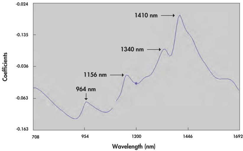
**Figure 10.10** Third PLS factor or loadings line plot for prediction of whole-grain barley moisture content. Calibration have been developed with log 1/R spectra.
