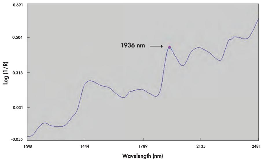
**Figure 1.1** Spectrum of ground wheat with the characteristic moisture absorption band indicated at 1936 nm.
