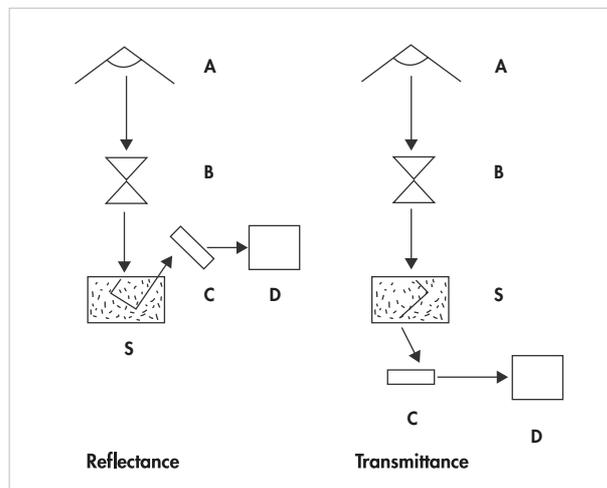
**Figure 6.1** Basic instrument design. A = light source; B = wavelength selection system; C = detector; D = computer; S = sample, including sample presentation system.
