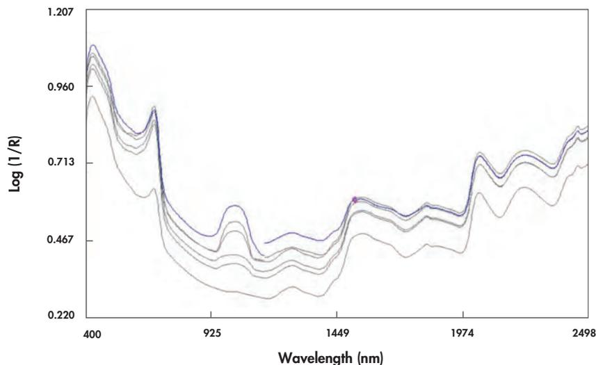
**Figure 9.2** Abnormal and normal spectra of straw. Note the distortion around 1000 nm.
