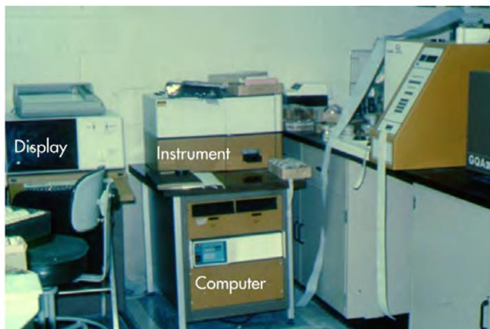
The first computerised scanning NIR spectrophotometer, the Pacific Scientific Model 6350, introduced by Neotec in 1978.
