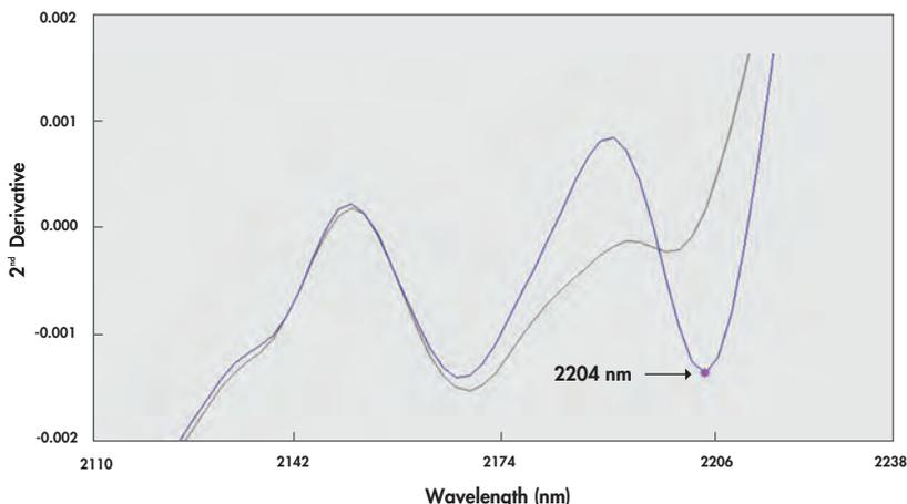
**Figure 6.9** Differences at around 2204 nm between 2<sup>nd</sup> derivative (2 4 4 1) spectra of two quartz windows.
