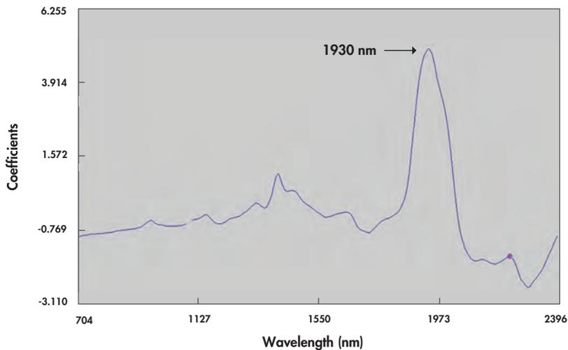
**Figure 10.12** Regression coefficients (b) for prediction of wheat flour moisture. Calibration has been developed with log 1/R spectra.
