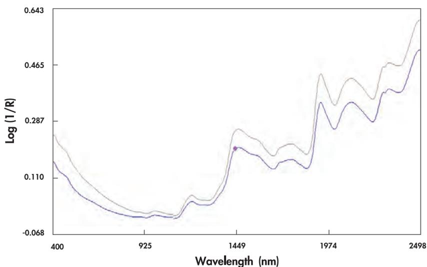
**Figure 7.2** Spectra of the same wheat sample, ground on two Cyclone grinders both fitted with 1.0 mm screens.
