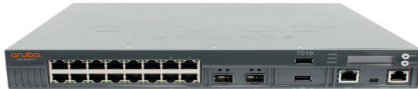
Figure 6.20 – Aruba 7010 mobility controller
