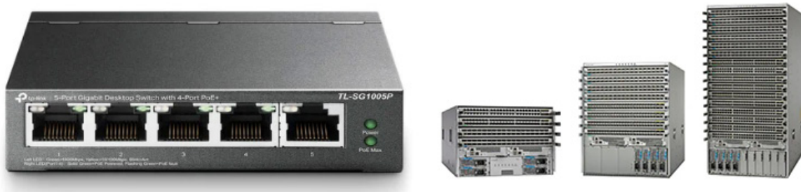
Figure 6.14 – A five-port tp-link unmanaged switch for home use (left) and Cisco Nexus 9000 series data center switches (right)
