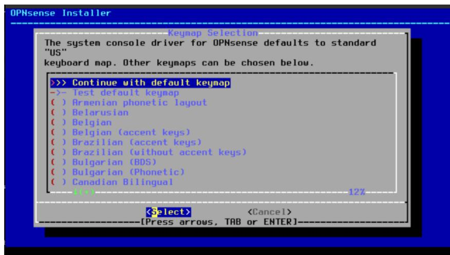
Figure 29 – Keyboard Mapping Configuration
