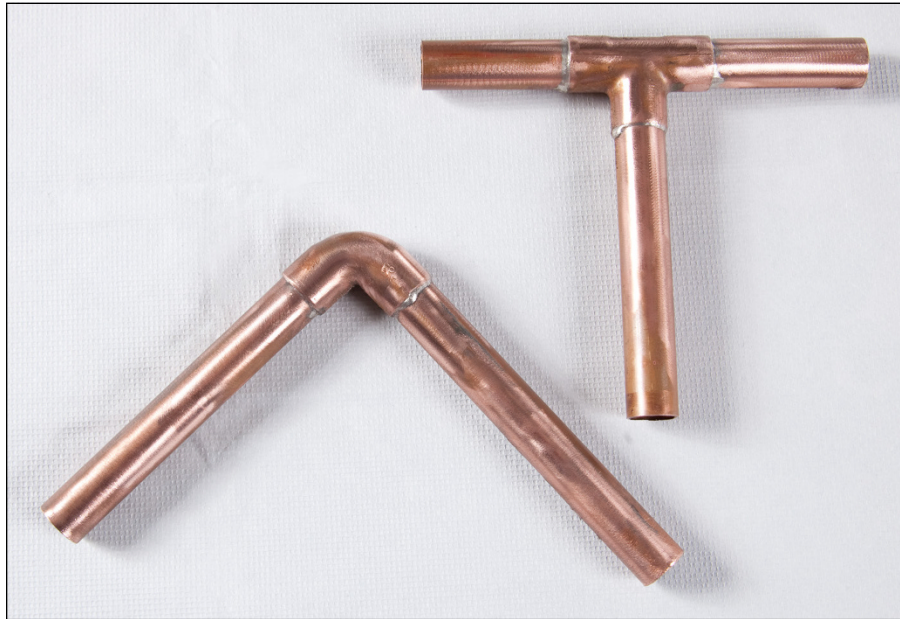
FIGURE 13-6: A soldered copper joint.
