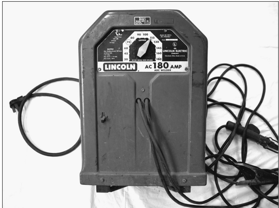
FIGURE 5-2: Transformer buzz box.
