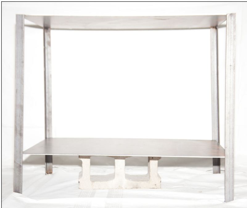
FIGURE 16-8: The partially constructed table lifted off the floor with spacers.
