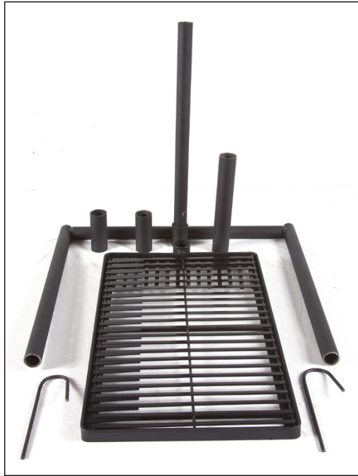
FIGURE 17-5: Partially constructed campfire grill.
