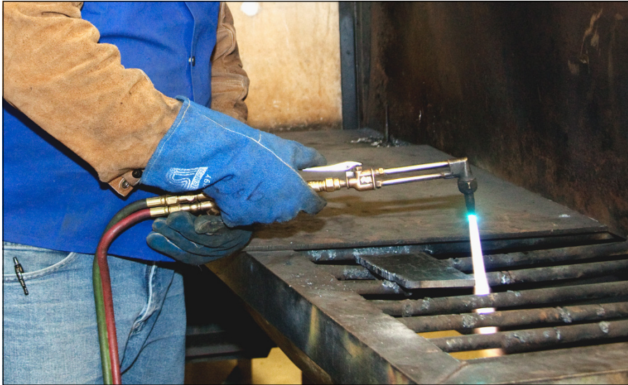
FIGURE 12-4: Operating an oxyfuel cutting torch.
