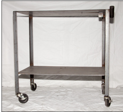
FIGURE 16-5: A completed portable welding table.
