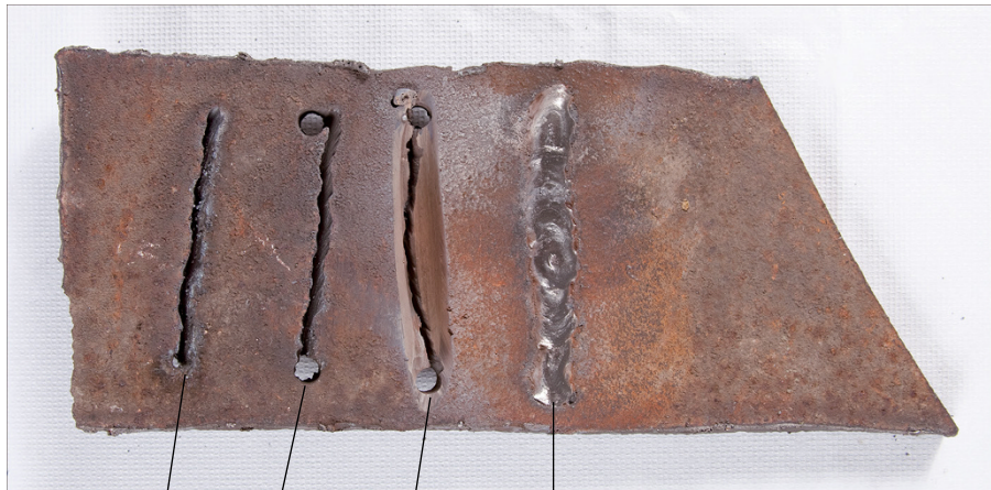
Crack Holes drilled in ends at crack Ground groove in preparation for welding Finished weld
