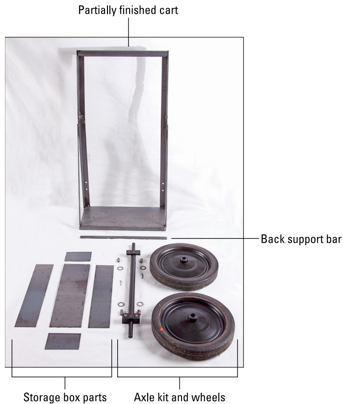
FIGURE 16-3: The partially welded torch cart.
