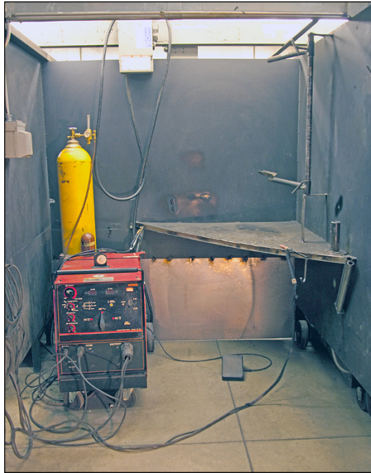
FIGURE 7-1: A tig welding setup.
