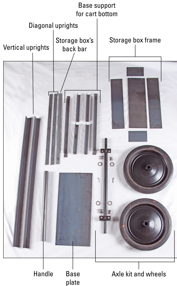
FIGURE 16-2: The steel pieces you need to build your torch cart.
