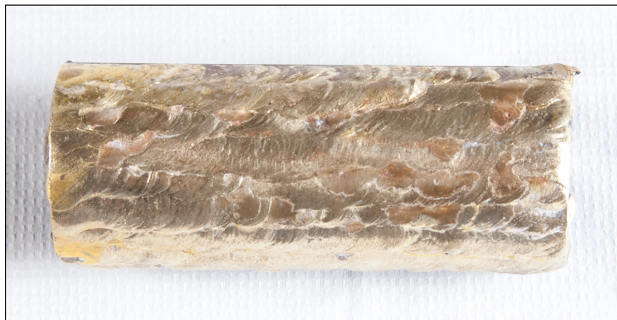
FIGURE 13-3: An example of a brazed corncob.
