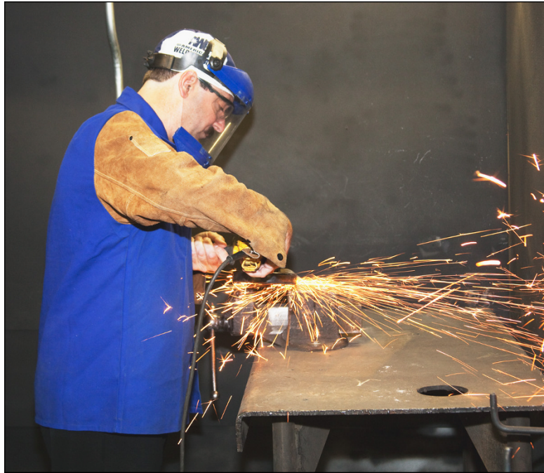
FIGURE 2-3: Cleaning steel with an angle grinder.
