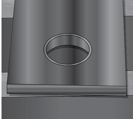
FIGURE 12-2: Perfect circle cut in aluminum.
