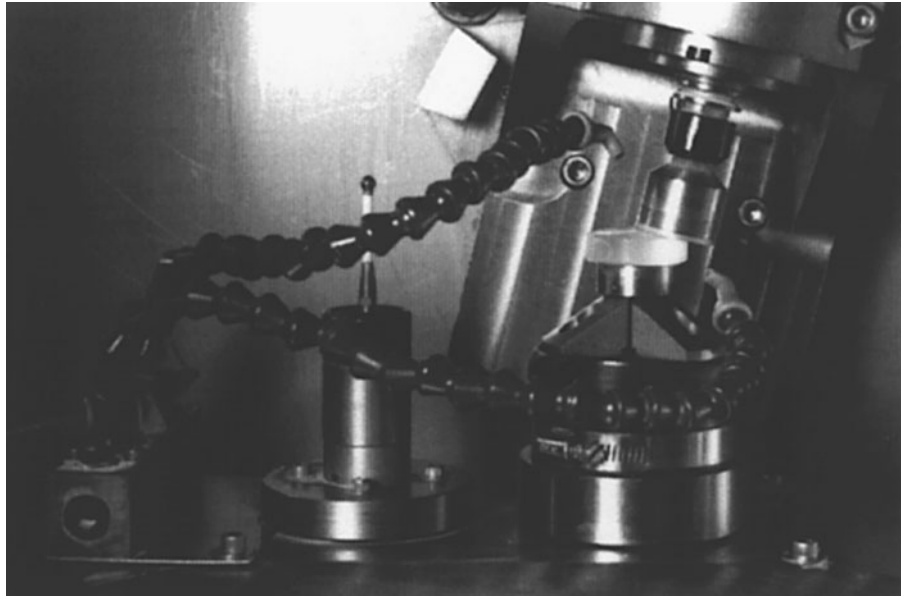
Figure 18.6 Deterministic Grinding with CNC Machine
