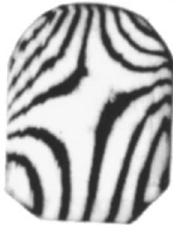
interferogram of thin aluminum mirror with astigmatism or saddle
