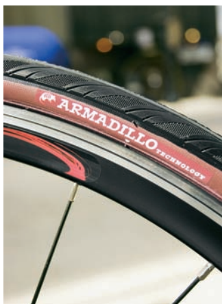
Armadillo bicycle tires reinforced with Kevlar are hard to pierce with sharp objects, so a cyclist rarely gets a flat tire.
