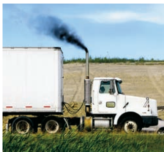
The sooty exhaust from trucks and buses contains PAHs such as benzo[ a ]pyrene.
