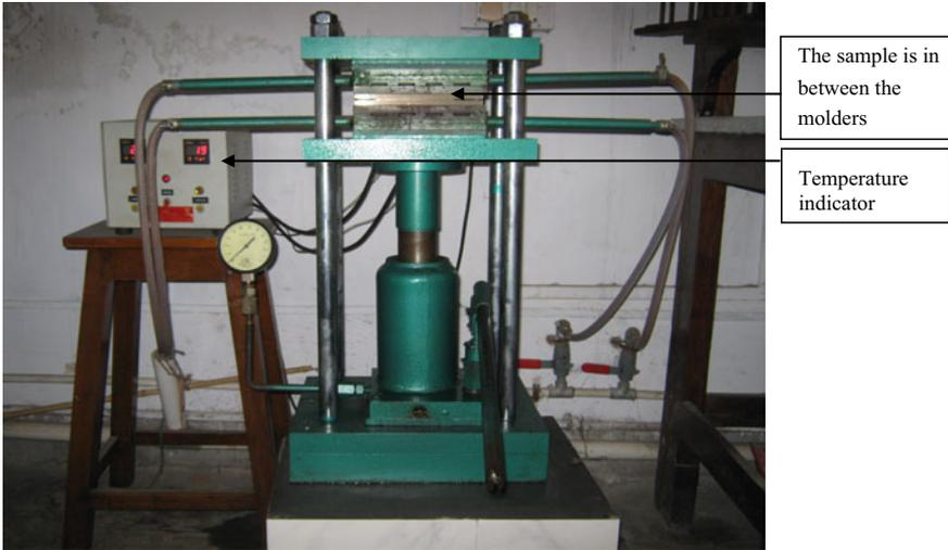
Fig. 3.2 Compression hot molding with temperature digital panel meter and pressure indicator
