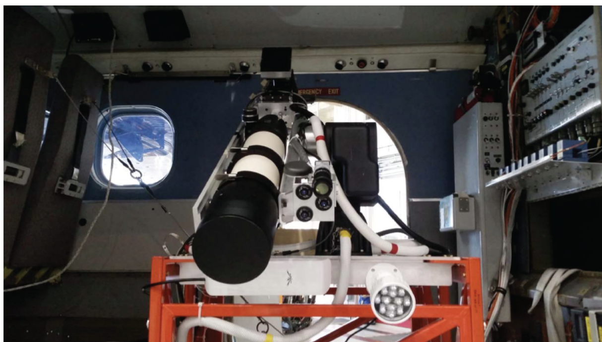
Figure 25.5 The receiver apparatus facing out the port-side door of the NRC Twin Otter research aircraft.
