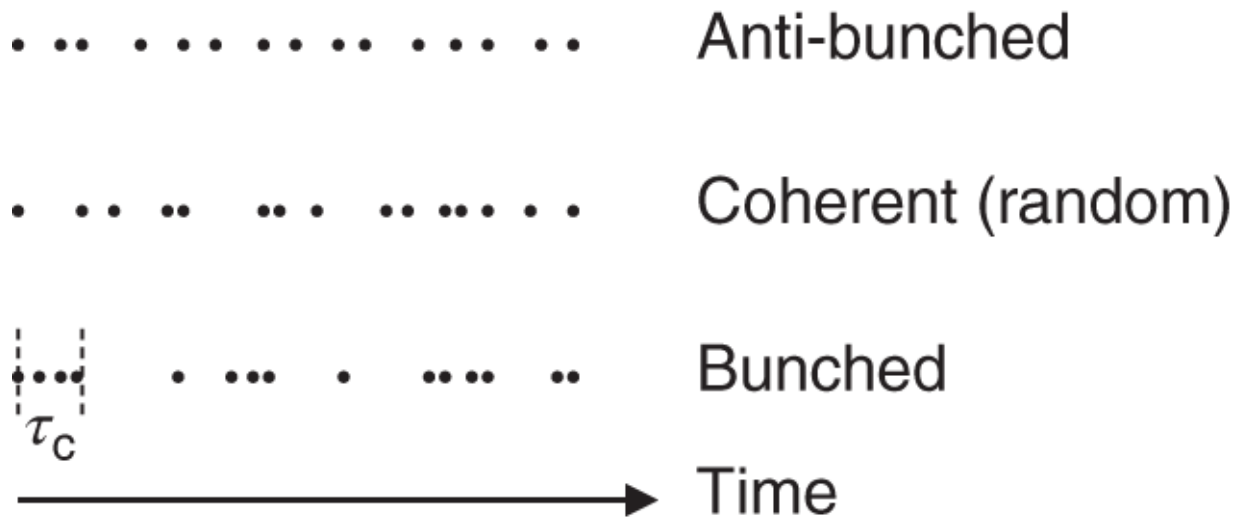
Figure 3.1 Schematic illustration of photon anti-bunching compared to coherent and bunched light. \tau_c is the coherence time of the bunched light.
