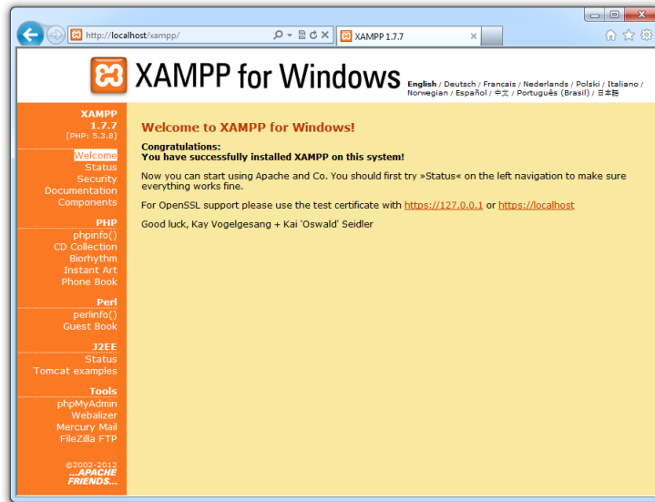
Figure 1.7. The admin page provided by XAMPP confirms your Apache web server is running
