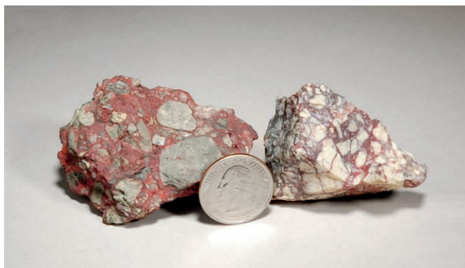
FIGURE 17.15 This is a piece of breccia, a sedimentary rock that formed from the consolidation of large angular fragments into a solid rock. This sample with gravel-sized and smaller fragments is from Colorado. Source: © Dr. Parvinder Sethi.
