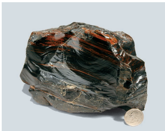
FIGURE 17.14 This is a piece of obsidian, which has the same chemical composition as the granite shown in Figure 17.12. Obsidian has a different texture because it does not have crystals and is a volcanic glass. The curved fracture surface is common in noncrystalline substances such as glass. Source: © Dr. Parvinder Sethi.
