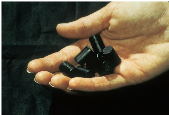
FIGURE 13.16 (A) These are uranium oxide fuel pellets that are stacked inside fuel rods, which are then locked together in a fuel rod assembly. (B) A fuel rod assembly. See also Figure 13.19, which shows a fuel rod assembly being loaded into a reactor. Source: a & b: © Arizona Public Service Company.
