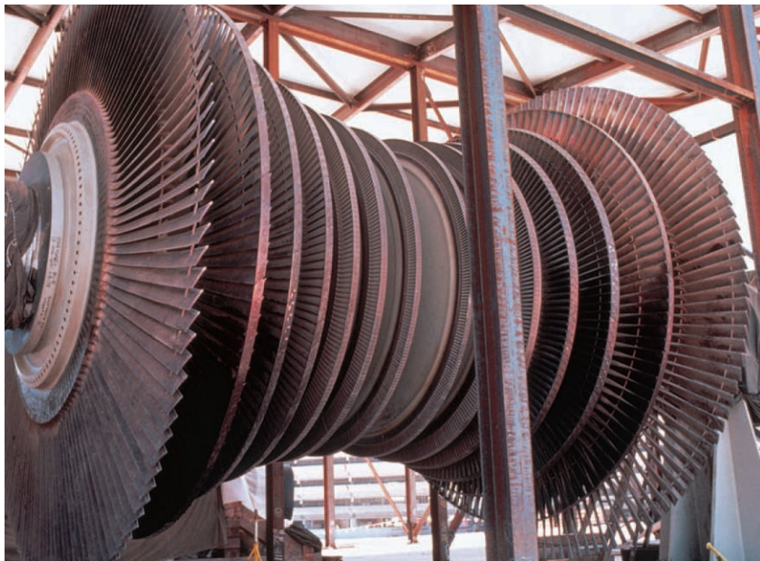
FIGURE 3.15 The blades of a steam turbine. In a power plant, chemical or nuclear energy is used to heat water to steam, which is directed against the turbine blades. The mechanical energy of the turbine turns an electric generator. Thus, a power plant converts chemical or nuclear energy to mechanical energy, which is then converted to electrical energy. Source: © Arizona Public Service Company.
