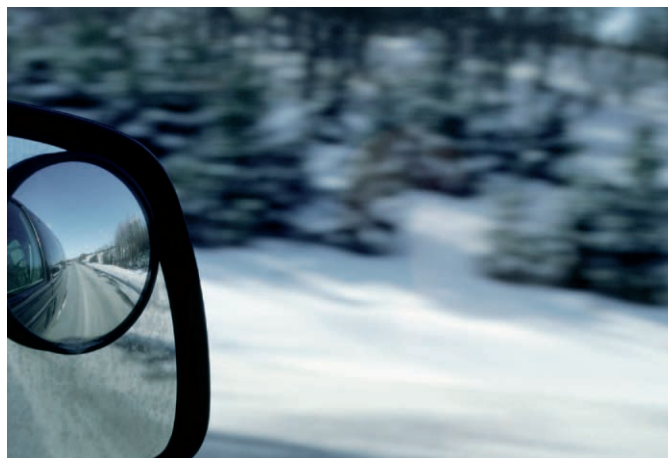
FIGURE 7.13 This convex mirror provides a wide-angle view, increasing your field of vision. Source: © image 100/Alamy, RF.
