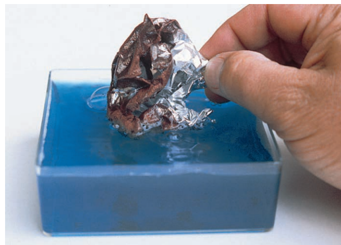
FIGURE 10.13 This shows a reaction between metallic aluminum and the blue solution of copper(II) chloride. Aluminum is above copper in the activity series, and aluminum replaces the copper ions from the solution as copper is deposited as a metal. The aluminum loses electrons to the copper and forms aluminum ions in solution.
