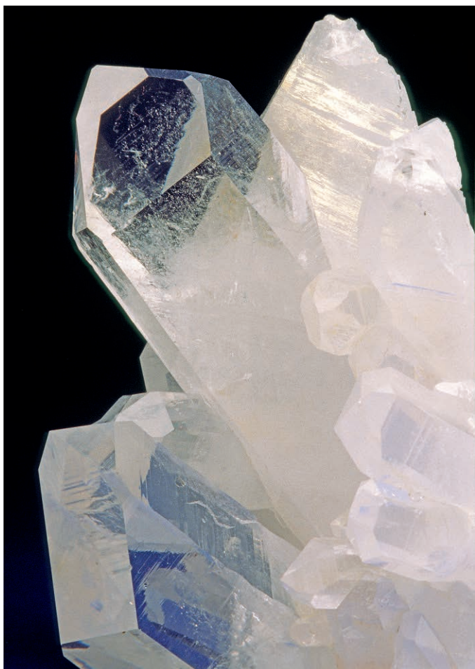
FIGURE 17.10 (A) Gypsum, with a hardness of 2, is easily scratched. (B) Quartz, with a hardness of 7, is so hard that even a metal file will not scratch it. Source: a & b: © Doug Sherman/Geofile.
