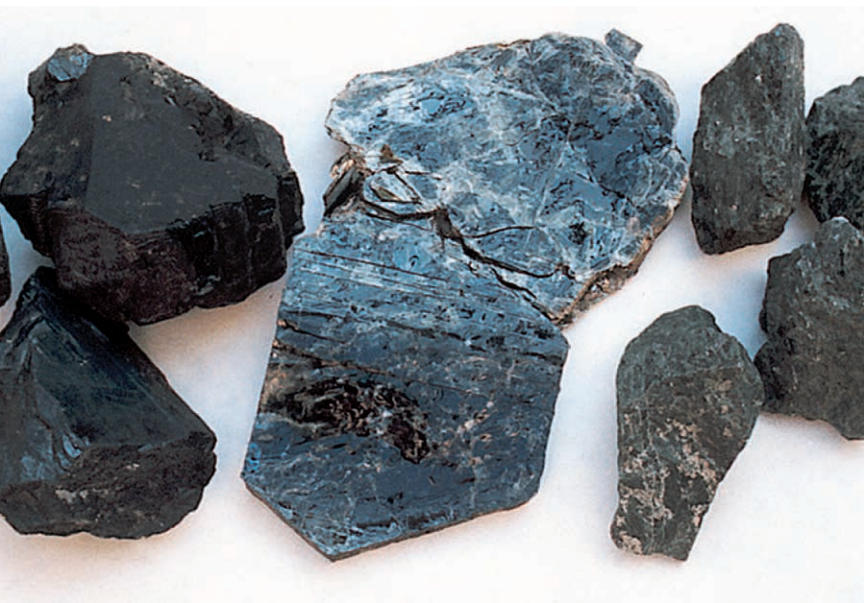
FIGURE 17.8 Compare the dark colors of the ferromagnesian silicates augite (right), hornblende (left), and biotite to the light-colored nonferromagnesian silicates in Figure 17.9. Source: © Bill W. Tillery.
