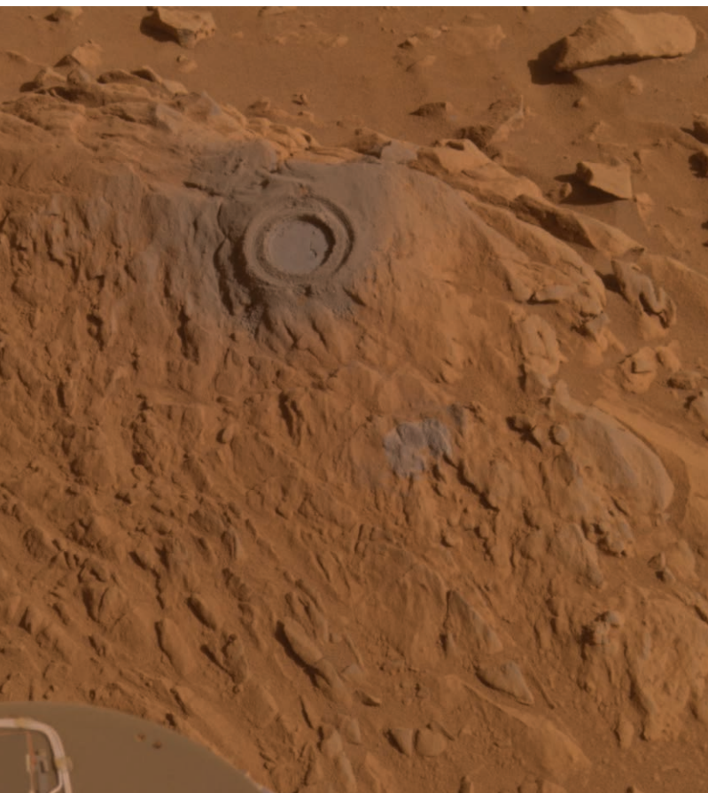
FIGURE 15.6 Researchers used the rover Spirit's rock abrasion tool to help them study a rock dubbed “Uchben” in the “Colombia Hills” of Mars. The tool ground into the rock, creating a shallow hole 4.5 cm (1.8 in) in diameter in the central upper portion of this image. It also used wire bristles to brush a portion of the surface below and to the right of the hole. Spirit used its panoramic camera during the rover’s 293rd Martian day (October 29, 2004) to take the frames combined into this approximately true-color image. Source: NASA.
