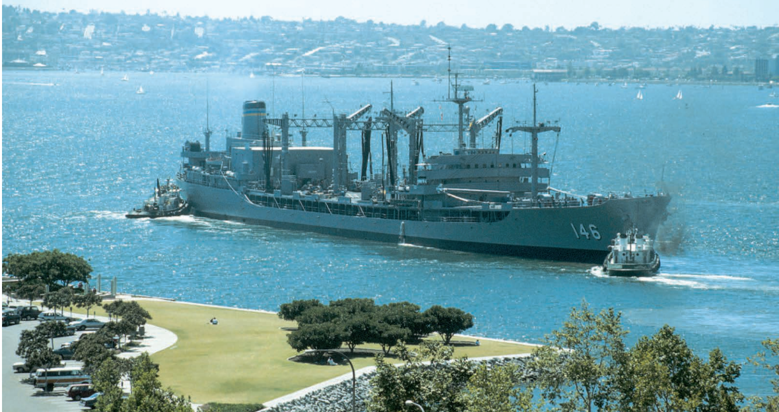
FIGURE 2.7 The rate of movement and the direction of movement of this ship are determined by a combination of direction and size of force from each of the tugboats. In which direction are the two tugboats pushing? What evidence would indicate that one tugboat is pushing with a greater force? If the tugboat by the numbers is pushing with a greater force and the back tugboat is keeping the back of the ship from moving, what will happen? Source: © Bill W. Tillery.
