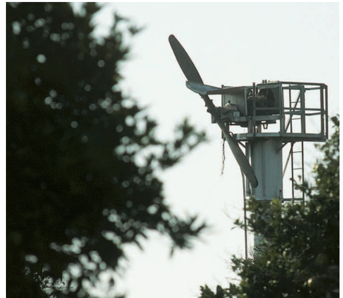
FIGURE 22.16 Fans like this one are used to mix the warmer, upper layers of air with the cooling air in the orchard on nights when frost is likely to form. Source: © Bill W. Tillery.
