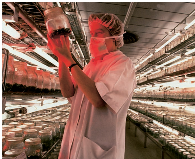
FIGURE 8.12 These fluorescent lights emit light as electrons of mercury atoms inside the tubes gain energy from the electric current. As soon as they can, the electrons drop back to a lower-energy orbit, emitting photons with ultraviolet frequencies. Ultraviolet radiation strikes the fluorescent chemical coating inside the tube, stimulating the emission of visible light.
