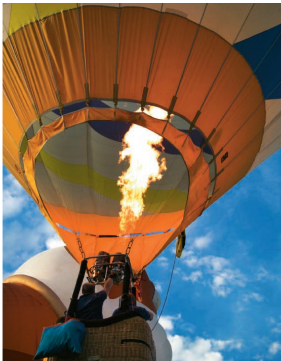
FIGURE 10.7 One of two burners is operating at the moment as this hot air balloon ascends. The burners are fueled by propane ( C_3H_8 ), a liquefied petroleum gas (LPG). Like other forms of petroleum, propane releases large amounts of heat during the chemical reaction of burning. Source: © Open Door/Alamy, RF.
