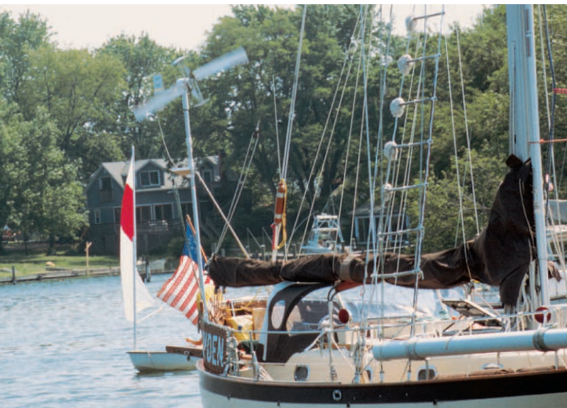
FIGURE 3.21 Wind is another form of solar energy. This wind turbine generates electrical energy for this sailboat, charging batteries for backup power when the wind is not blowing. In case you are wondering, the turbine cannot be used to make a wind to move the boat. In accord with Newton's laws of motion, this would not produce a net force on the boat. Source: © Bill W. Tillery.
