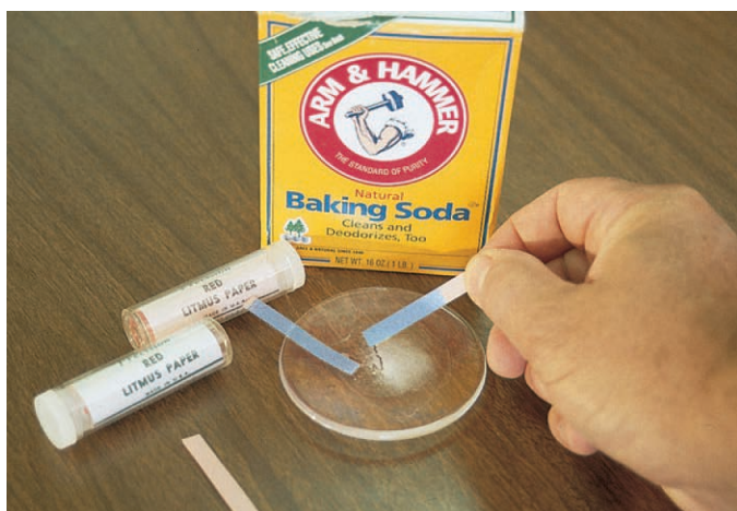
FIGURE 11.14 (A) Acid solutions will change the color of blue litmus to red. (B) Solutions of bases will change the color of red litmus to blue. Source: a & b: © Bill W. Tillery.
