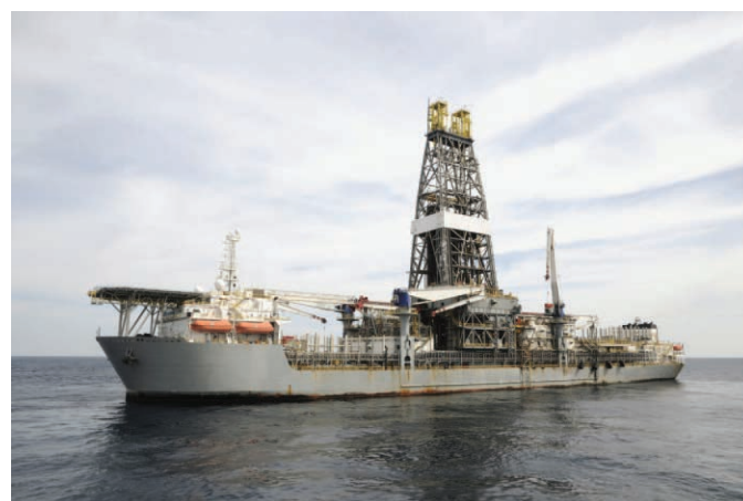
FIGURE 18.1 This drilling ship samples sediment and rock from the deep ocean floor. It can only sample materials well within the upper crust of Earth, however, barely scratching the surface of Earth's interior. Source: © Brad Martin/Getty Images, RF.
