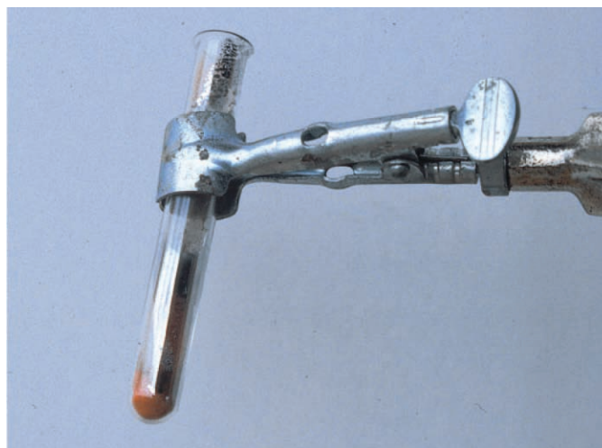
FIGURE 10.11 Mercury(II) oxide is decomposed by heat, leaving the silver-colored element mercury behind as oxygen is driven off. This is an example of a decomposition reaction, 2 \text{HgO} \rightarrow 2 \text{Hg} + \text{O}_2\uparrow .
