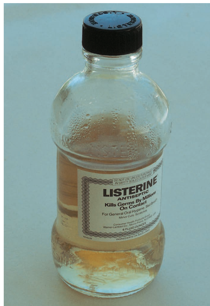
FIGURE 4.22 The inside of this closed bottle is isolated from the environment, so the space above the liquid becomes saturated. While it is saturated, the evaporation rate equals the condensation rate. When the bottle is cooled, condensation exceeds evaporation and droplets of liquid form on the inside surfaces. Source: © Bill W. Tillery.
