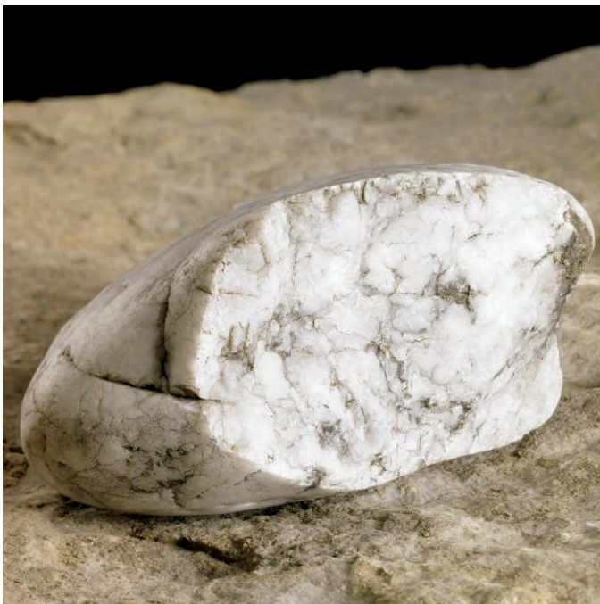
FIGURE 17.21 This is a sample of marble, a coarse-grained metamorphic rock with interlocking calcite crystals. The calcite crystals were recrystallized from limestone during metamorphism. Source: © Achim Prill/Photodisc/Getty Images, RF.
