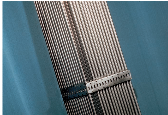
FIGURE 13.16 (A) These are uranium oxide fuel pellets that are stacked inside fuel rods, which are then locked together in a fuel rod assembly. (B) A fuel rod assembly. See also Figure 13.19, which shows a fuel rod assembly being loaded into a reactor. Source: a & b: © Arizona Public Service Company.
