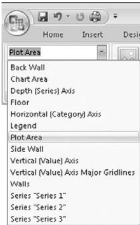
Figure 15-5 You can choose different chart elements to work with by using the menu in the Current Selection group of the Chart Tools Layout tab.
