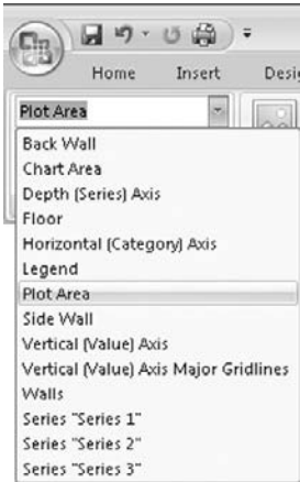
Figure 15-5 You can choose different chart elements to work with by using the menu in the Current Selection group of the Chart Tools Layout tab.
