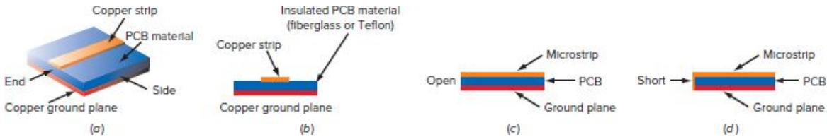
Figure 18-7 Microstrip transmission line used for reactive circuits. (a) Perspective view. (b) Edge or end view. (c) Side view (open line). (d) Side view (shorted line).
