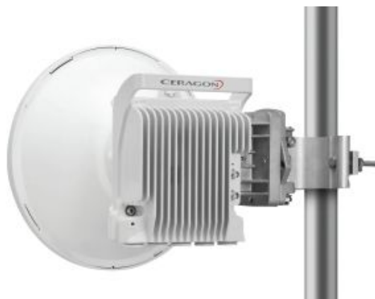
Figure 21-11 The Ceragon FibeAir IP-20C is typical of the small-cell backhaul units available. This one packages the radio, interfaces, and dish antenna into a single unit and is available in standard licensed band frequencies from 6 to 71 GHz. Typical data rate is 1 Gbps in a single Ethernet channel. It uses 2048 QAM.
