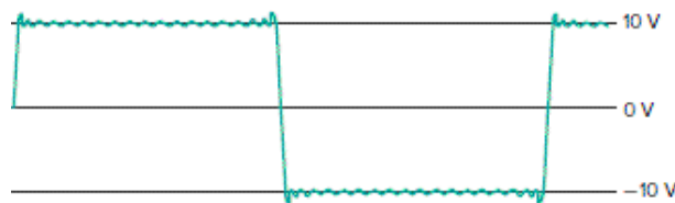
Figure 2-59 Square wave made up of 20 odd harmonics added to the fundamental.
