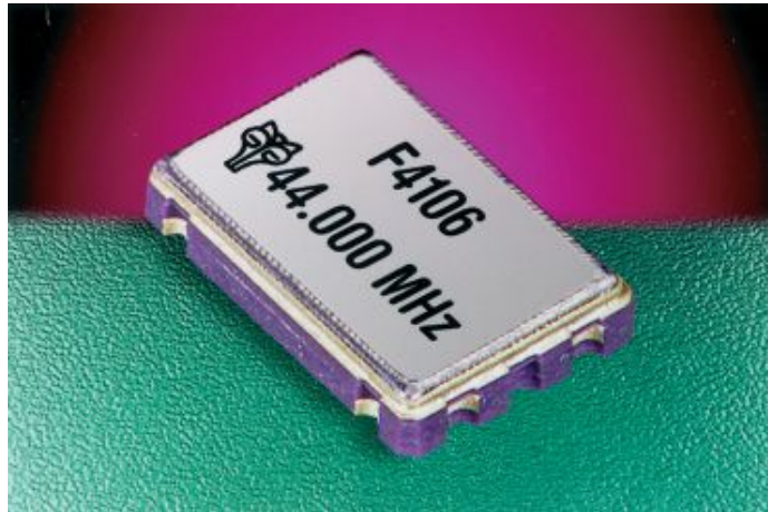
Figure 8-7 A surface-mount crystal oscillator in a sealed package.
