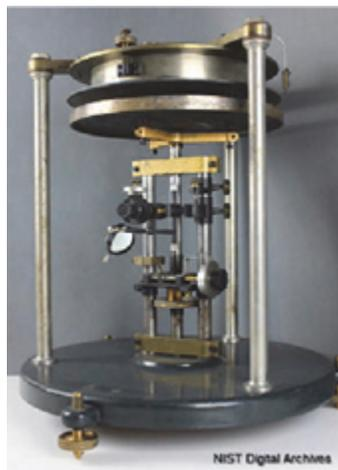
**Figure 5.1:** Photo of the adjustable parallel plate capacitor used to measure the speed of light in 1907. (Courtesy of National Institute of Standards and Technology Digital Collections, Gaithersburg, MD.) [1]
