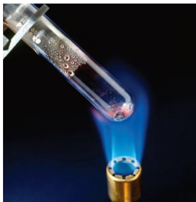
FIGURE 1.6 The red solid, mercury oxide, decomposes into liquid mercury and oxygen gas, when heated. Note the drops of liquid mercury condensing on the side of the test tube.
