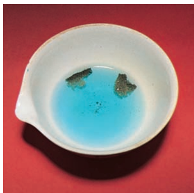
FIGURE 11.14 Copper(II) sulfide reacts with concentrated nitric acid to liberate nitrogen oxide and produce a solution of copper(II) sulfate, which displays the characteristic blue color of copper(II) ions in water.
