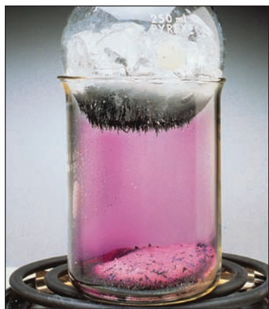
FIGURE 6.57 Iodine sublimes from the bottom of the beaker and condenses on the bottom of the chilled round-bottom flask.
