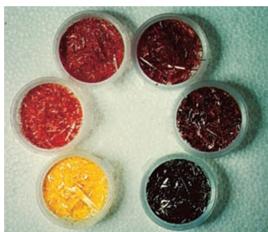
FIGURE 22.28 Mixed crystals of two semiconductors with different band gaps, CdS (yellow) and CdSe (black), show a range of colors, illustrating a decrease in the band gap energy as the composition of the mixture becomes richer in Se.
