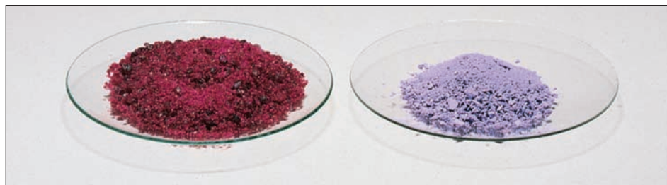
FIGURE 2.1 When cobalt(II) chloride crystallizes from solution, it brings with it six water molecules per formula unit, producing a red solid with the empirical formula \text{CoCl}_2 \cdot 6 \text{H}_2\text{O} . This solid melts at 86^\circ\text{C} ; it loses some of the water when heated above 110^\circ\text{C} to form a lavender solid with the empirical formula \text{CoCl}_2 \cdot 2 \text{H}_2\text{O} .
