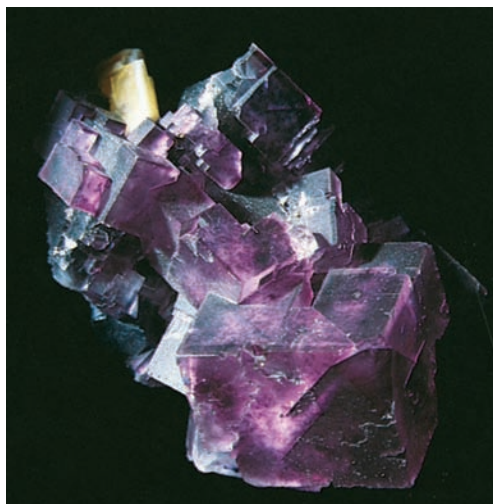
FIGURE 21.29 Pure calcium fluoride, \text{CaF}_2 , is white but the natural sample of calcium fluoride (fluorite) shown here is a rich purple because F-centers are present. These are lattice sites where the \text{F}^- anion is replaced by an electron only.
