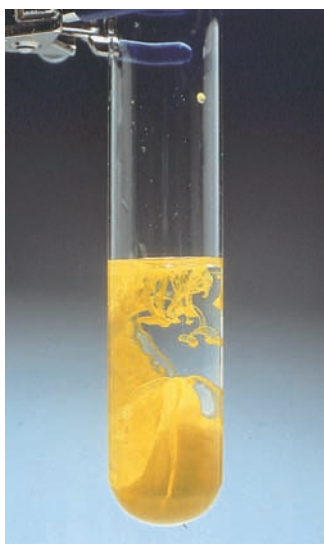
FIGURE 16.4 A yellow precipitate of lead iodide forms when a drop of KI solution is added to a solution of \text{Pb}(\text{NO}_3)_2 .
