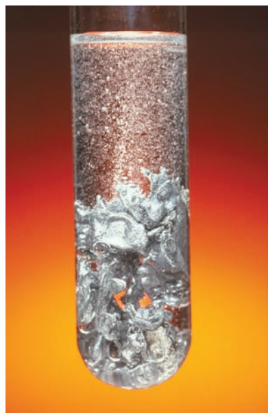
FIGURE 15.2 As zinc dissolves in dilute hydrochloric acid, bubbles of hydrogen appear, and zinc chloride forms in solution.
