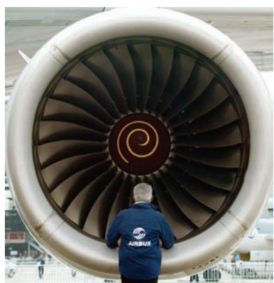
FIGURE 2.4 A jet engine fan blade made of a single-crystal titanium alloy.
