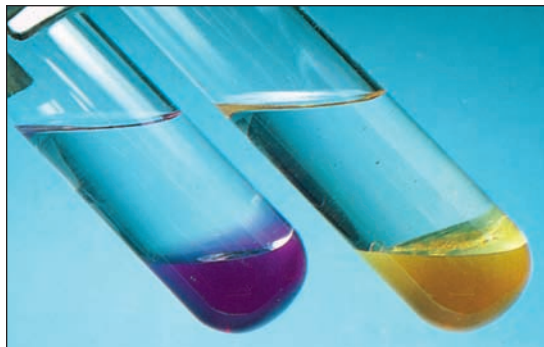
FIGURE 7.11 One way to distinguish alkanes from alkenes is by their reactions with aqueous KMnO_4 . This strong oxidizing agent does not react with hexane and retains its purple color (left). But, when KMnO_4 is placed in contact with 1-hexene, a redox reaction occurs in which the brown solid MnO_2 forms (right) and -OH groups are added to both sides of the double bond in the 1-hexene, giving a compound with the formula CH_3(CH_2)_3CH(OH)CH_2OH .
