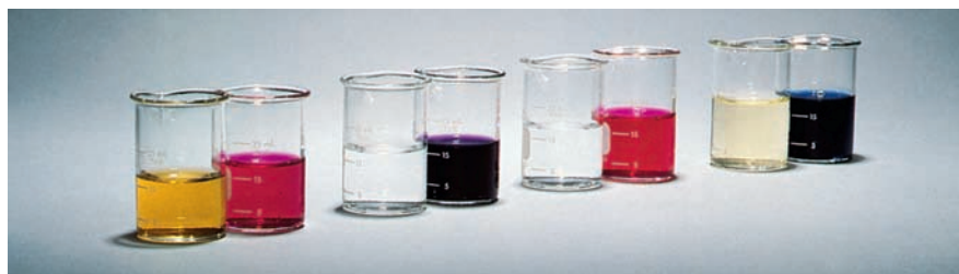
FIGURE 15.11 Color differences in four indicators: bromophenol red, thymolphthalein, phenolphthalein, and bromocresol green. In each case the acidic form is on the left and the basic form is on the right.
