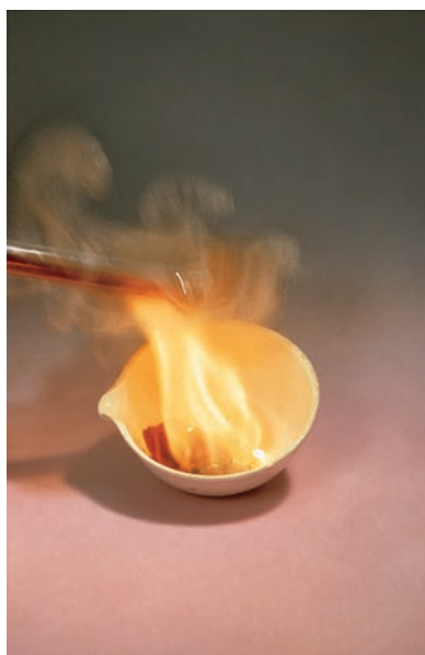
FIGURE 12.18 Red phosphorus reacts exothermically in liquid bromine. The rising gases are a mixture of the product \text{PBr}_3 and unreacted bromine that has boiled off.
