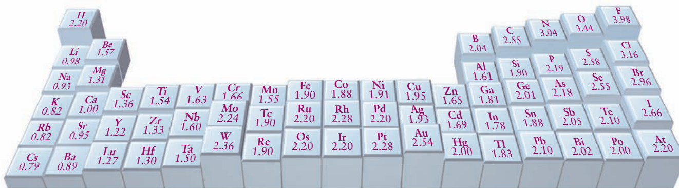
FIGURE 3.18 Average electronegativity of atoms, computed with the method that Linus Pauling developed. Electronegativity values have no units.
