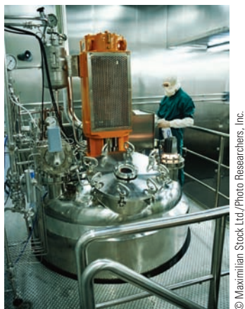
FIGURE 7.38 Fermentation tanks used in modern penicillin production.
