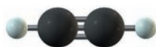
FIGURE 3.27 Ethyne, or acetylene, \text{C}_2\text{H}_2 , has a triple bond that makes it highly reactive.
