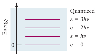
FIGURE 4.12 An oscillator described by Planck's postulate has discrete energy levels. It can gain or lose energy only in amounts that correspond to the difference between two energy levels.
