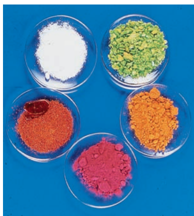
FIGURE 8.23 Several colored coordination compounds. (clockwise from top left) They are \text{Cr}(\text{CO})_6 (white), \text{K}_3[\text{Fe}(\text{C}_2\text{O}_4)_3] (green), [\text{Co}(\text{en})_3]^{3+} (orange), [\text{Co}(\text{NH}_3)_5(\text{OH}_2)]\text{Cl}_3 (red), and \text{K}_3[\text{Fe}(\text{CN})_6] (red-orange).
