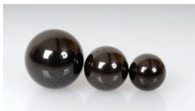
FIGURE 22.9 Silicon carbide ball bearings are harder, stiffer, and have smoother surfaces than steel bearings, resulting in improved performance due to reduced friction and less heat. Their high melting points make them the bearings of choice for demanding, high temperature applications.
