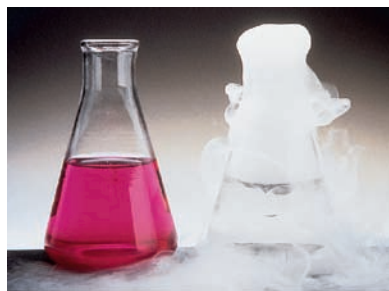
FIGURE 15.19 The indicator phenolphthalein is pink in basic solution ( left ). When dry ice (solid carbon dioxide) is placed in the bottom of the beaker ( right ), it dissolves to form carbonic acid. This neutralizes the base in solution, and causes the indicator to change to its colorless form characteristic of an acid solution.
