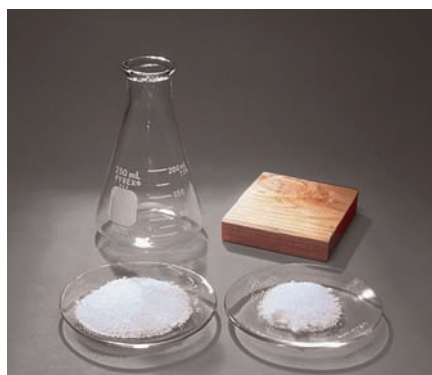
FIGURE 12.17 (a) When mixed in a flask, the two solids \text{Ba}(\text{OH})_2 \cdot 8\text{H}_2\text{O}(s) and \text{NH}_4\text{NO}_3(s) undergo an acid–base reaction: \text{Ba}(\text{OH})_2 \cdot 8\text{H}_2\text{O}(s) + 2 \text{NH}_4\text{NO}_3(s) \longrightarrow \text{Ba}(\text{NO}_3)_2(aq) + 2 \text{NH}_3(aq) + 10 \text{H}_2\text{O}(\ell) . (b) The water produced dissolves excess ammonium nitrate in an endothermic reaction. The dissolution absorbs so much heat that the water on the surface of the wet wooden block freezes to the bottom of the flask, and the block can be lifted up with the flask.
