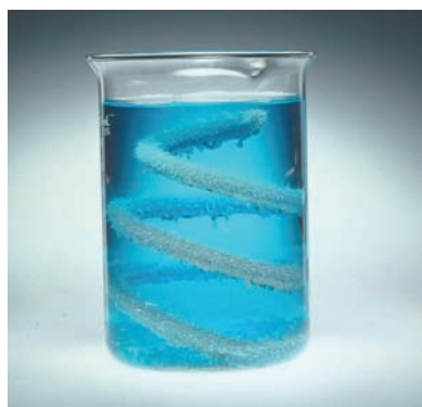
FIGURE 11.13 When a piece of copper wire is inserted into a solution of silver nitrate, metallic silver deposits on the wire and the solution turns blue as \text{Cu}^{2+} ions form.
