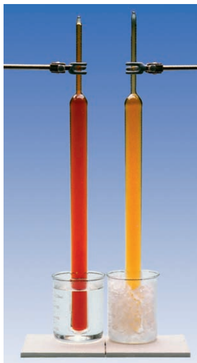
FIGURE 14.9 The equilibrium between \text{N}_2\text{O}_4 and \text{NO}_2 depends on temperature. The tube on the right, held in an ice bath at 0^\circ\text{C} , contains mostly \text{N}_2\text{O}_4 . Its color is pale because only \text{NO}_2 is colored. The deeper color in the tube on the left, which is held at 50^\circ\text{C} , reflects the increased \text{NO}_2 present in equilibrium at the higher temperature. The tubes contain the same masses of substance, distributed in different ways between \text{NO}_2 and \text{N}_2\text{O}_4 .
