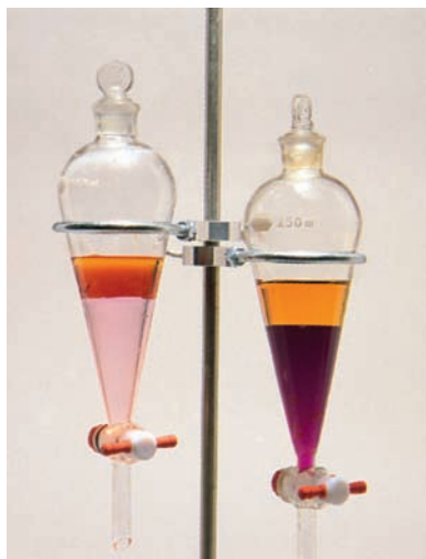
FIGURE 14.14 Iodine is dissolved in water and poured on top of carbon tetrachloride in a separatory funnel (left). After the funnel is shaken (right), the iodine reaches a partition equilibrium between the upper (aqueous) phase and the lower ( \text{CCl}_4 ) phase. The deeper color in the lower phase indicates that iodine dissolves preferentially in the denser \text{CCl}_4 phase.
