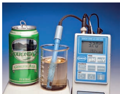
FIGURE 15.4 A simple pH meter with a digital readout. Most soft drinks are quite acidic due to the reaction of dissolved \text{CO}_2 with water to make carbonic acid ( \text{H}_2\text{CO}_3 ).
