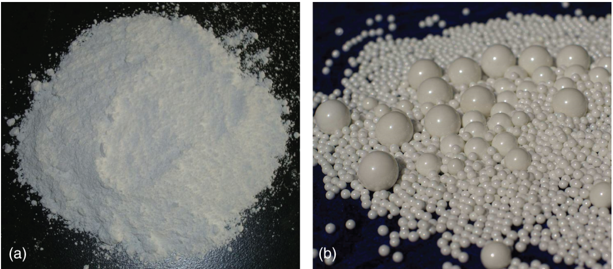
Figure 5.2 (a) High-purity \text{ZrO}_2 powders, (b) High-purity \text{ZrO}_2 beads.
