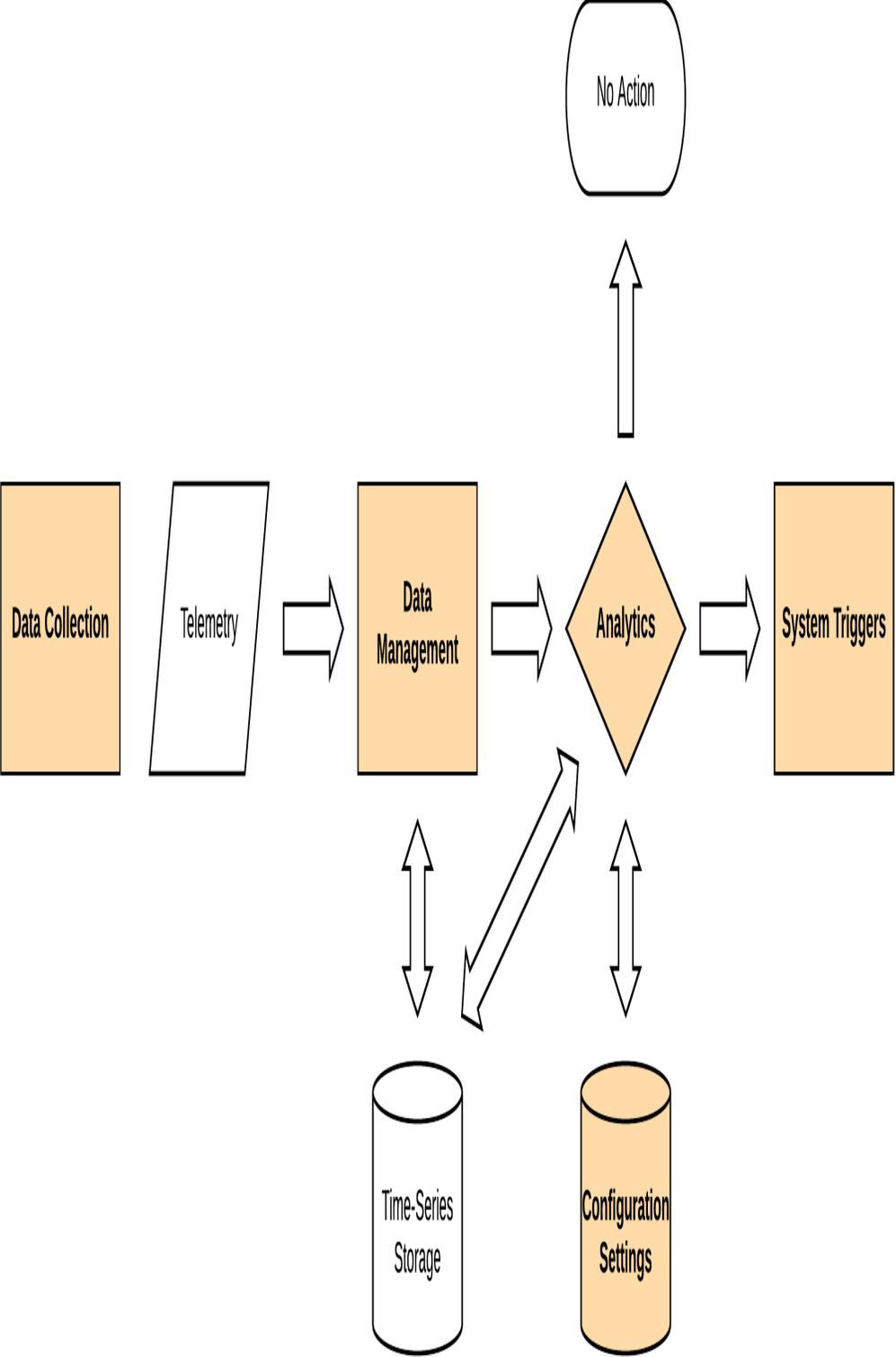
*Figure 1-1. Simple IoT data flow*
