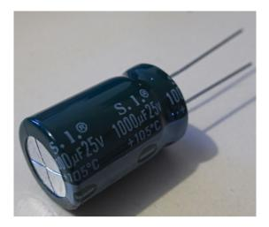
A capacitor is a component that can be used to store electrical energy. It stores energy when there is a difference in voltage between its two plates. Once the voltage difference dissipates, it releases the stored energy.
