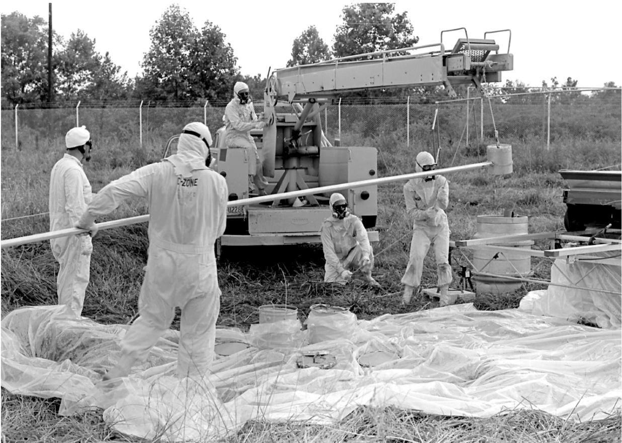
5.4 Stanley Auerbach operates a hoist handling a cask of cesium-137-tagged sand in the post-nuclear-attack ecology study plots at Oak Ridge National Laboratory, Tennessee, c. 1968. Oak Ridge National Laboratory
