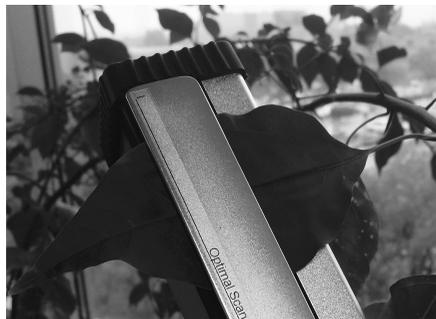
**FIGURE 13.12** Leaf size measurements by portable scanners.
