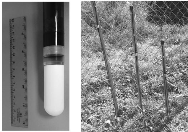
**FIGURE 4.18** Soil tensiometers: (a): ceramic cup. (b): three tensiometers installed at various depths.
