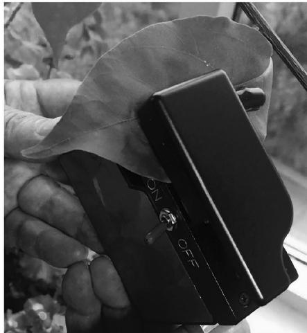
**FIGURE 13.17** Portable leaf spectrometer.
