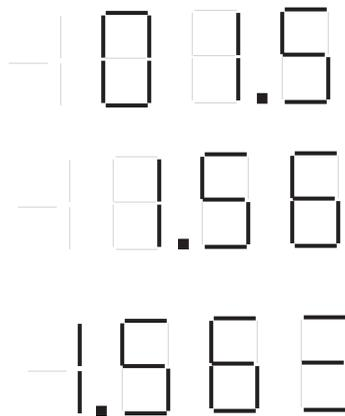
FIGURE 3.14 A V DC reading on 200 V, 20 V, and 2 V scale.
