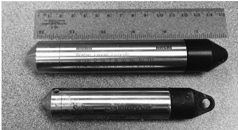
FIGURE 5.15 Examples of submersed sensor plus datalogger.
