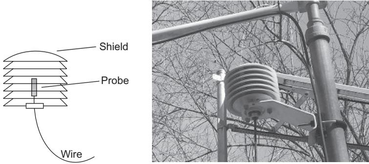
FIGURE 3.26 Radiation shield to protect the temperature transducer in air temperature measurement.
