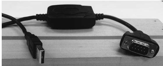
**FIGURE 2.6** Examples of RS-232 to USB cable for compatibility with legacy systems.
