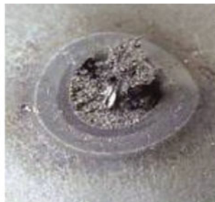
Interfacial Fracture with Partial Thickness Fracture
