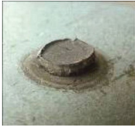
Fig. 4.16 The full button pull indicates acceptable weld quality when testing conventional steels [Source AWS]
