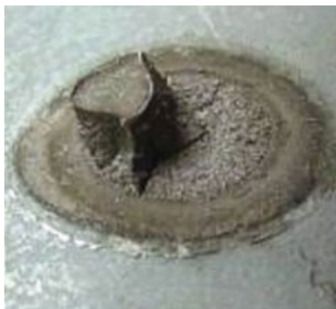
Interfacial Fracture with Button Pull
