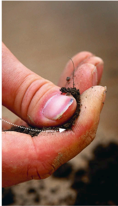
Test for sandy soil by rubbing earth through your fingertips. It will feel gritty.
