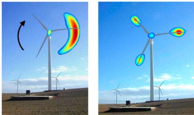
FIGURE 31.2 In-field beamforming measurements [12].
