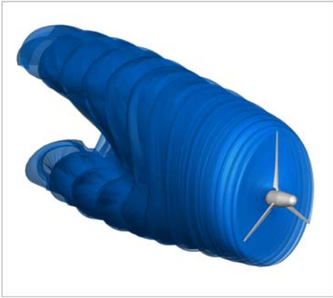
FIGURE 23.5 Mexico rotor in yawed flow: predicted three-dimensional shape of rotor wake by a panel code. From Greco L, Testa C. Wind turbine unsteady aerodynamics and performance by a free-wake panel method. Renew. Energy 2021;164:444–459.
