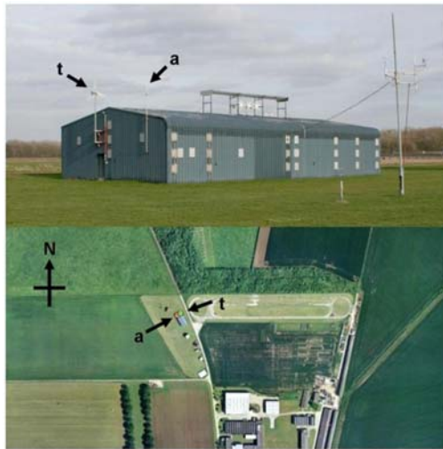
FIGURE 9.13 Windsave WS1000 turbine ( t ) and ultrasonic anemometer (Vaisala WMT50, a ) on South West side of an industrial shed surrounded by low-lying fields. Silsoe site measured wind-speed data, March 2008–February 2009. NOABL wind-speed is 4.6 m/s, and for NOABL-MCS, 3.8 m/s.
