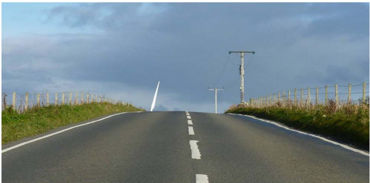
FIGURE 30.15 An isolated blade tip creates a windscreen wiper effect. South Ronaldsay, UK. Photo: B Dower. All rights reserved.
