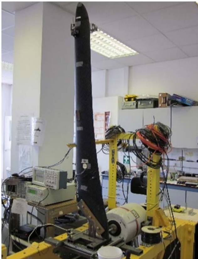
FIGURE 19.5 Wind turbine blade exposed to dynamic loading testing [36].
