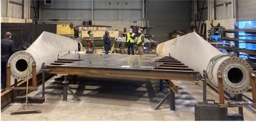
FIGURE 19.3 Connection test on wind turbine blades in Munster Technological University Ireland (Heavy Structure Lab).
