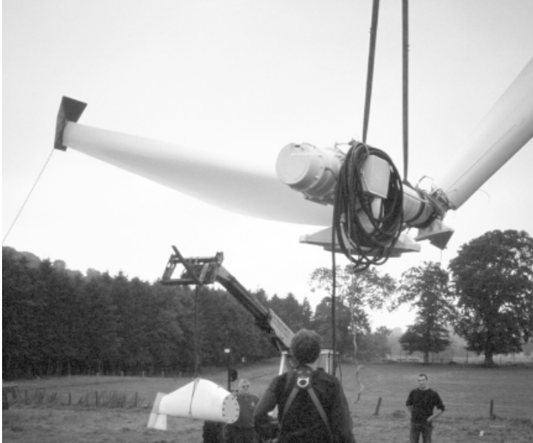
Figure 4.16 Vane-type tip brakes on the AOC15/50 wind turbine. The brake plate at the blade tip is held in place by an electromagnetic latch and deploys automatically under the action of centrifugal force.
