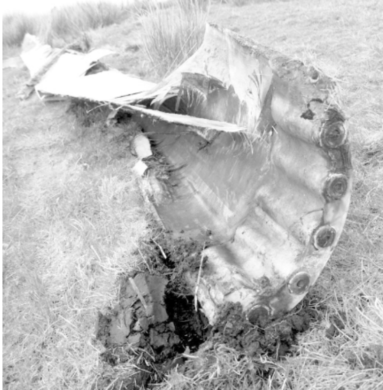
Figure 5.18 Lightning damage. Heat and pressure generated by the strike have blown the surfaces of this blade apart, with evidence of charring. All large blades now incorporate effective lightning protection.
