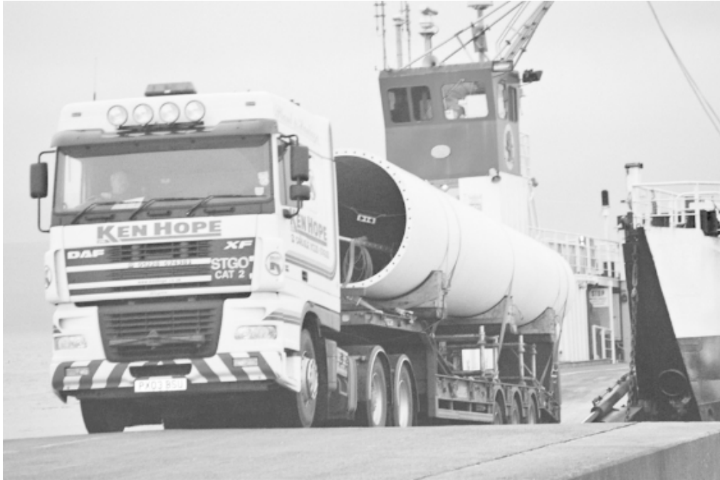
Figure 11.11 Ferry delivery of V27 tower section to Gigha in 2004. (Photo courtesy Donald Mackay)
