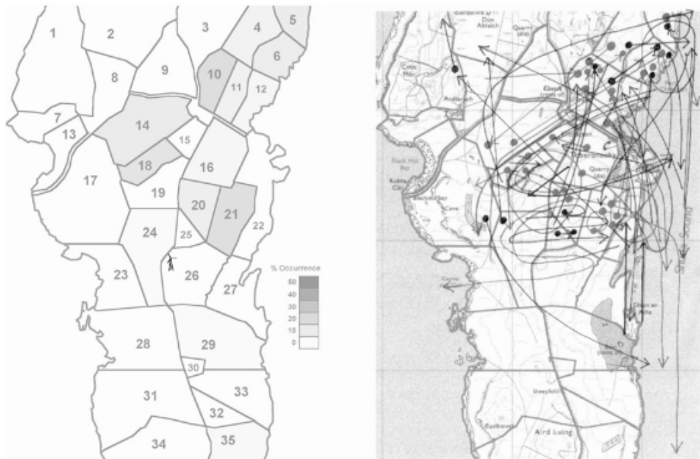
Figure 10.1 Pre-development species survey for a small wind turbine project on the Island of Luing, Argyll (Lamont et al., 2003). (Left) frequency distribution of barnacle geese in numbered fields; (right) observed flight lines from roost areas. (© Crown copyright and database rights 2019, OS licence number 100037385)
