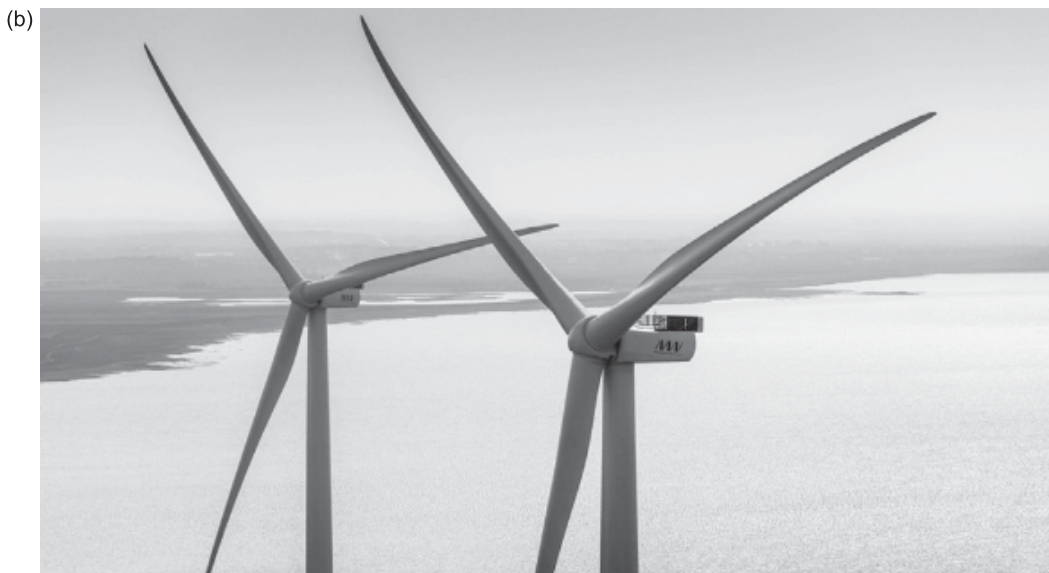
Figure 4.5 High and low solidity. The Windmatic 22 kW (a) designed by Christian Riisager in 1975 had 10% solidity and a design tip speed ratio of 4.0. The Vestas V164-8MW (b) has solidity of 4% and design tip speed ratio of 8.0. (V164 photo courtesy Vestas Wind Systems A/S)
