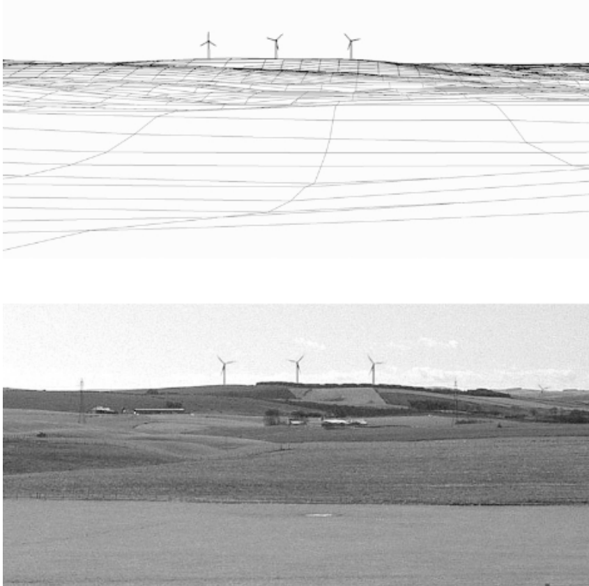
Figure 10.4 Visual representation of a proposed three-turbine windfarm: ( top ) wireframe plot based on digital terrain data; ( bottom ) photomontage. (Reproduced with kind permission of Greenspan Energy Ltd)
