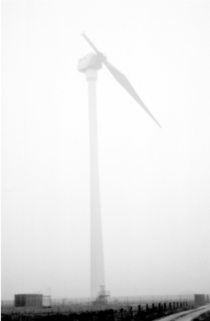
Figure 4.8 Monopteros: a single-bladed 640 kW wind turbine. Photographed on a foggy day at the DEWI test site, Wilhelmshaven, 1992.
