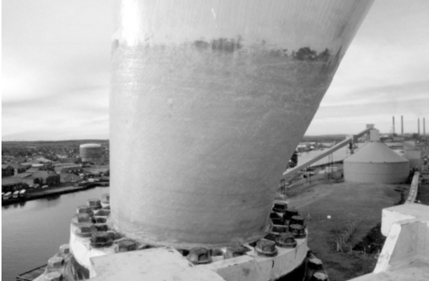
Figure 8.19 Flanged blade root. No longer used, this attachment method was susceptible to fatigue due to stress concentration at root–flange interface. (Windmaster 300 kW blade at Blyth Harbour, 1995)
