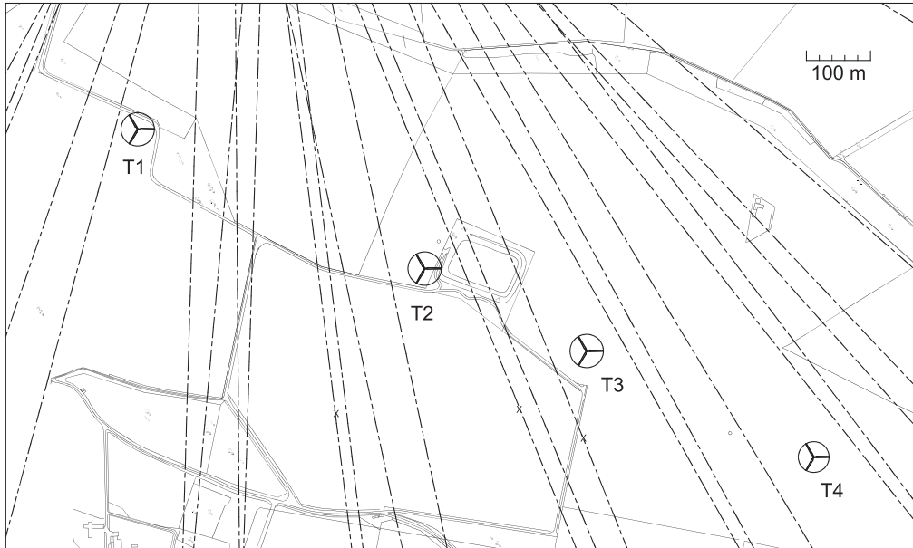
Figure 10.15 Co-existing with microwave links. Accurate surveying of link paths (dashed lines) and turbine positions enabled this windfarm in Aberdeenshire to be constructed without causing interference, where conservative link avoidance criteria would have ruled it out. Equation (10.7) applies. (© Crown copyright and database rights 2019, OS licence number 100037385)
