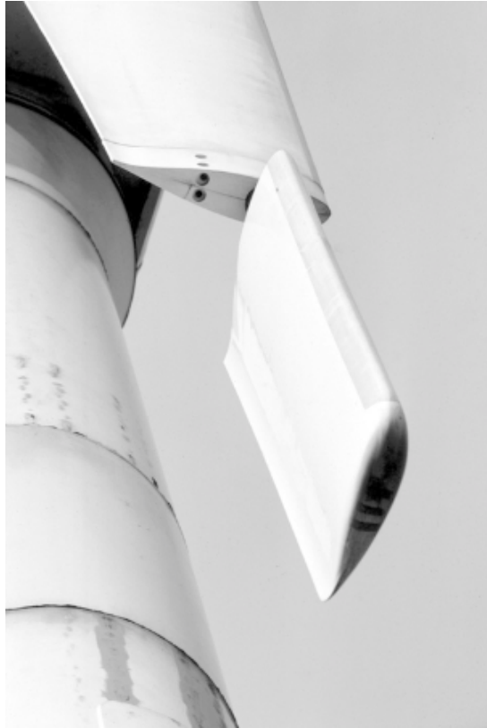
Figure 6.12 Tip air brake. The blade tip is shown pitched to 90° for maximum braking torque: it automatically deploys on loss of grid or on detection of overspeed. On this CSVP machine, the pitch system was also used for power regulation (Howden HWP28, Orkney, 1991).
