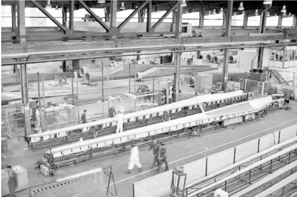
Figure 8.21 Manufacture of 23 m glass-epoxy blades via resin infusion moulding. Dry glass fabric is being laid into the two half moulds to facilitate the vacuum resin infusion process. Partly finished blades can be seen in the background. (Aerpac UK factory, Kirkcaldy, circa 2000)
