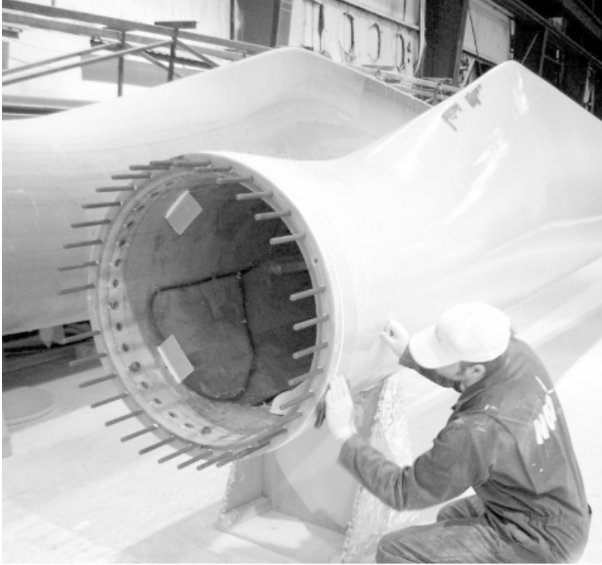
Figure 8.14 Root of a 16 m GFRP blade being finished, NOI Scotland factory, circa 2003. Note the thick root shell where multi-axial glass fabrics are used to resist complex stresses; also note the T-bolt root attachments.
