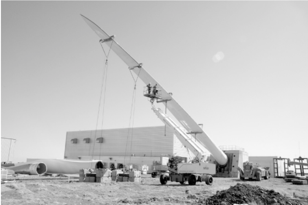
Figure 8.28 Static testing of a 45 m blade using distributed weight loading at the National Wind Technology Center, Colorado, in 2006. The blade is angled upwards to allow for static bending deflection. (Reproduced with permission from the National Renewable Energy Laboratory. Original image from NREL/PR-500-48898, available at https://www.nrel.gov/docs/fy10osti/48898.pdf )
