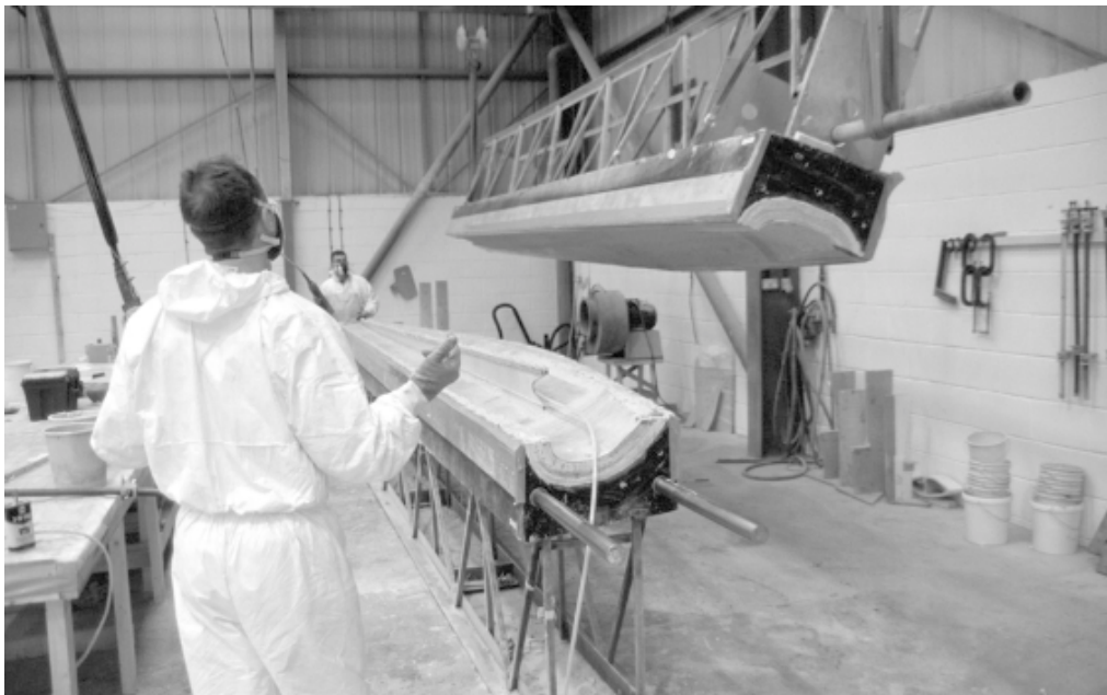
Figure 8.24 Joining the halves of a wood-epoxy blade. The shear web has been pre-bonded into the lower blade shell and adhesive paste applied to the leading and trailing edge bond lines. (Aerpac UK factory circa 1997)
