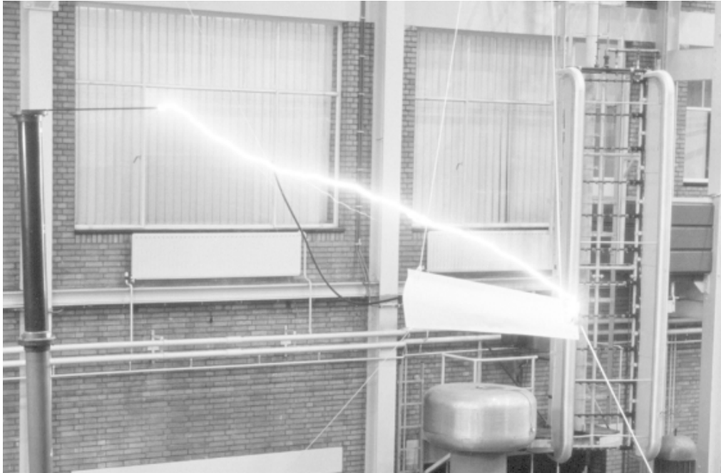
Figure 5.19 Lightning test on the tip of a 19 m Aerpac blade at the KEMA high-voltage labs, Arnhem, 1995. The discharge has successfully gone to ground via a silver-plated receptor. (Photo reproduced with kind permission of KEMA Laboratories)
