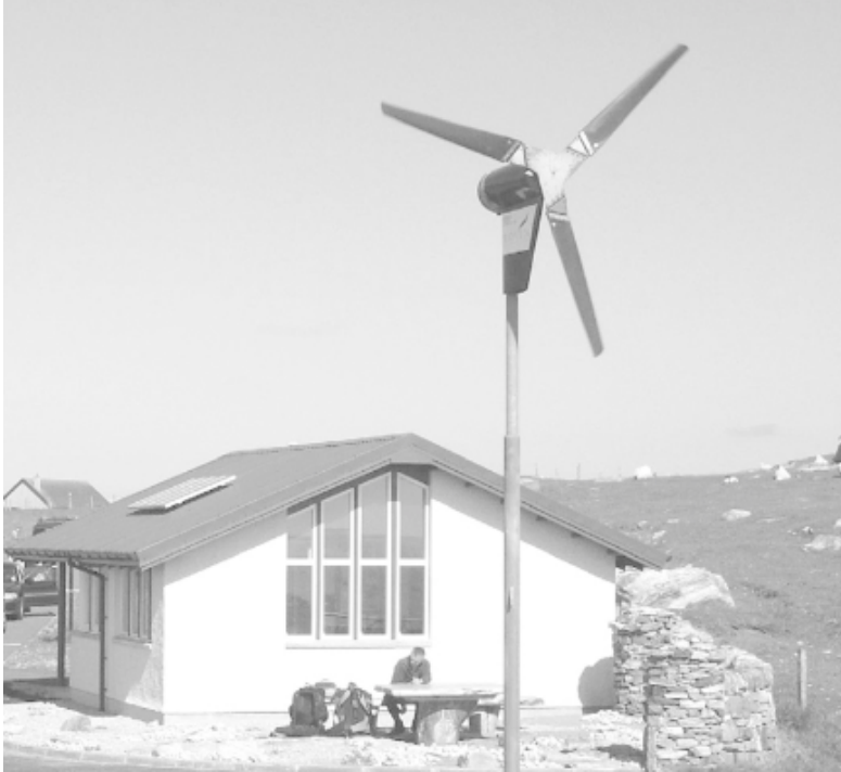
Figure 4.18 Proven 600 W free-yaw downwind machine. The streamlined nacelle shroud helps to eliminate tower shadow. (Photo reproduced with kind permission of Charlie Robb)
