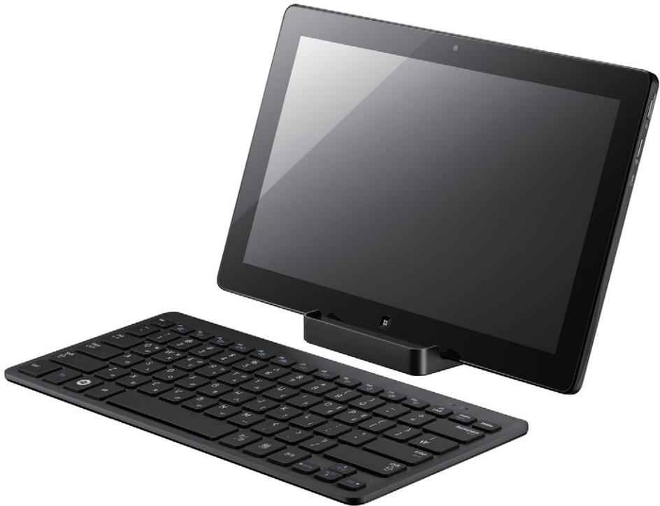
**FIGURE 1-10:** A docked tablet can function as a desktop computer by adding a keyboard and mouse.
