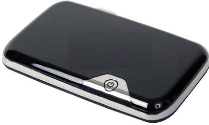
**FIGURE 13-8:** A portable wireless router can connect multiple PCs and devices to a cellular data network.
