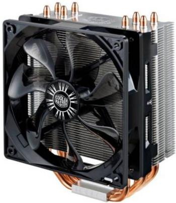
As the name denotes, CPU Cooler is used to cool the processor. If you work with your computer for a long time, the internal components become hot. It's essential to cool down the processor to extend the functionality to prevent abnormal sounds from inside your PC. You can either make use of the bundled CPU cooler or a dedicated third-party CPU
