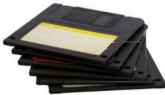
A floppy drive is mainly used to store data from your PC inside a specially designed floppy disk. The storage capacity of the floppy disk measures only 1.44MB and you can only store data within this capacity. The floppy disk was popular until 2006 but got outdated when portable hard drives and USB pen drives became popular. However, computer technicians still use floppies to perform system level work.
