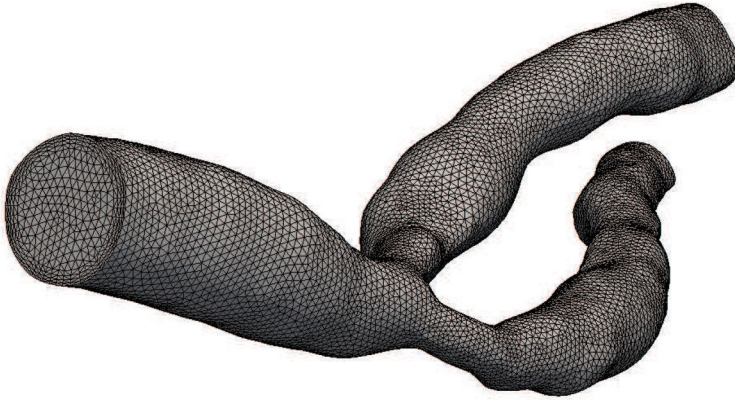
Figure 2.1 Computational mesh of a carotid bifurcation: unstructured volumetric mesh comprised of tetrahedrons.
