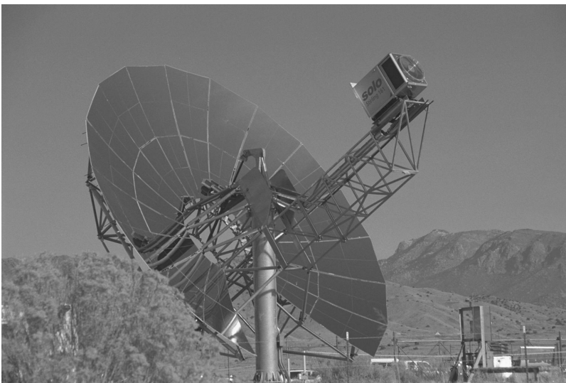
FIGURE 67.3 Advanced dish development system (ADDs) on test at Sandia National Laboratories' National Solar Thermal Test Facility. (Photograph courtesy of Sandia National Laboratories)
