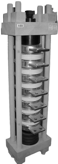
FIGURE 120.7 High-voltage switch built of stacked thyristors.
