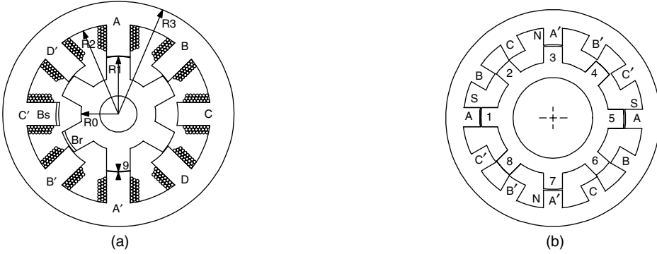
FIGURE 76.21 Cross-sections of three-phase SR machines: (a) four-phase 8/6 structure; (b) 12/8, two-repetition structure. (From Husain, I. 2002. Switched reluctance machines, in Power Electronics Handbook , Skvarenina, T. L., Ed., CRC Press, Boca Raton, FL.)
