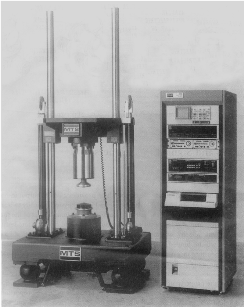
FIGURE 19.5 Shock machine and associated instrumentation. (Courtesy MTS Systems Corp.)
