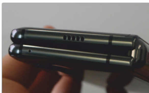
NEW MATERIALS Many more metal elements make the overall body of the Galaxy Fold far tougher.
