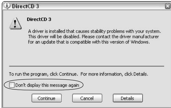
• Figure 11-1: A telltale sign of an auto-starting program attempting to load a bad driver.
