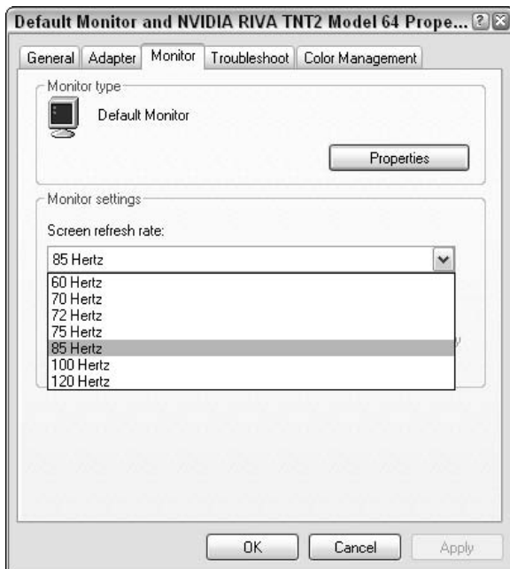
• Figure 7-8: You can adjust refresh settings manually, but Windows XP may not use them.
