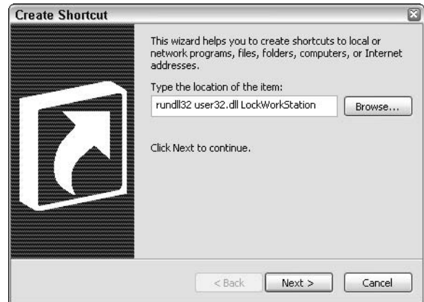
• Figure 6-5: To switch users quickly, use LockWorkStation .
