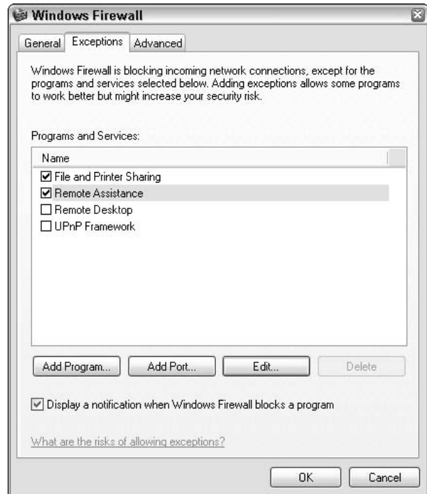
• Figure 61-1: Windows Firewall must be set to allow Remote Assistance to poke through.
