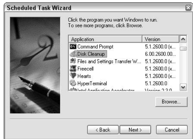
• Figure 56-9: The Windows Scheduler runs any program on your computer, at the time(s) you specify.
