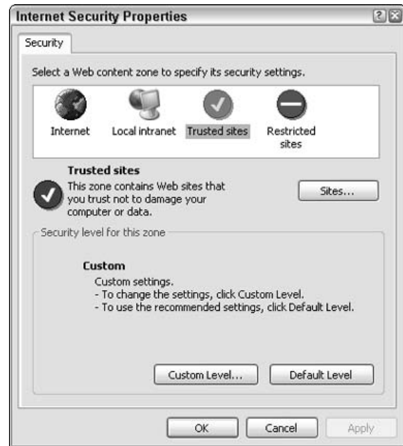
• Figure 23-22: Control the security of each zone and assign sites to zones in this dialog box.
