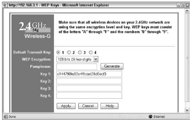
• Figure 46-5: The Linksys WRT54G’s WEP encryption key goes in a specific box. Other routers are similar.
