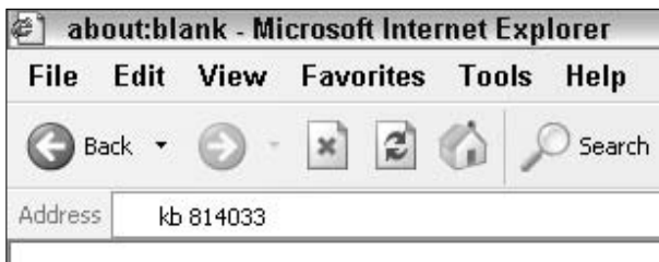
• Figure 23-12: With this trick, I just type kb and the article number I'm looking for.
