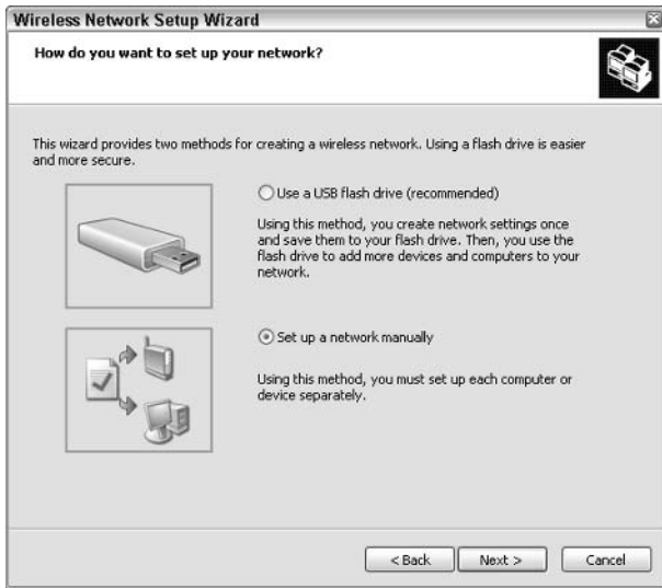
• Figure 46-2: Unfortunately, you can only use a key drive if your wireless router has a USB port, and it understands WSNK.
