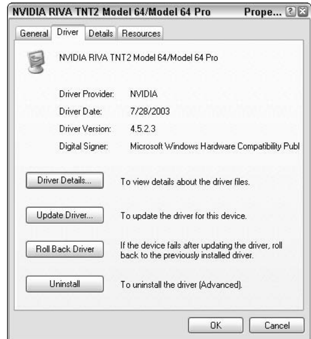
• Figure 58-9: Properties for the video card with the updated driver.
