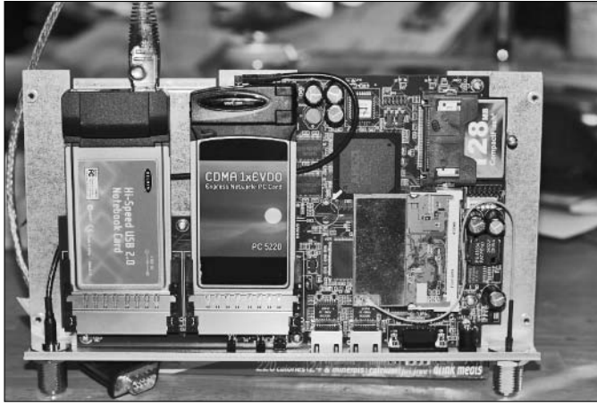
Figure 11-7: The insides of a completed Stompbox EV-DO/Wi-Fi router.
