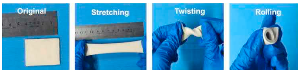
FIGURE 31.10 Images of the TENG with silver-coated glass microspheres by Li et al. Copyright (2021) [38].
